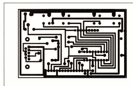
Figure 3. PCB track bottom side
