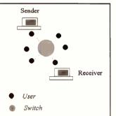
Figure 1. Local arrangement of users without, and then with a single network switch reducing the number of required interconnections for every user to talk or travel to every other user.
