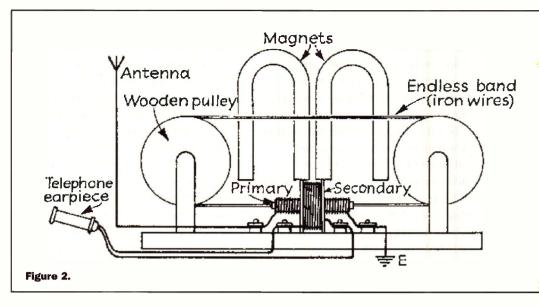
began experimental work to produce a commercially viable detector, based on Rutherford's research. The result was the detectors shown in Figures 1 and 2. The earlier of the two designs used a rotating magnet and stationary coils, whilst the second attempt was - in its way - a far more practical version of Rutherford's origination.
