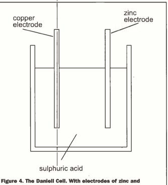
Figure 4. The Daniell Cell. With electrodes of zinc and copper, and sulphuric acid as the aqueous medium giving half cells of zinc/zinc sulphate and copper/copper sulphate, Daniell's cell could give larger continuous currents than Volta's cell.
