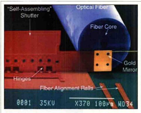
Example of first practical micro electro mechanical optical switch. When the bar is lowered (as shown) the signal on the left is deflected to the rear fibre. When raised the signal path continues to the fibre on the right without interaction.
