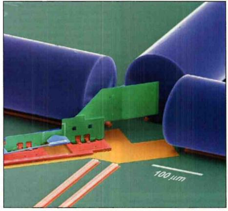
Further example of microelectro mechanical optical switch
