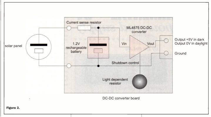
A light dependent resistor controls the on/off of the DC-DC converter. If the ambient light intensity is higher than a preset threshold, the DC-DC converter is switched off. During switch off, the battery is isolated from the load completely so that there is no current flowing through the load. If the ambient light intensity is lower than the threshold, the DC-DC converter is switched on, outputting +5V DC voltage.
