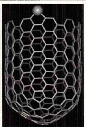
Simulated image of collection of singlewall carbon nanotubes. Courtesy Rice University
