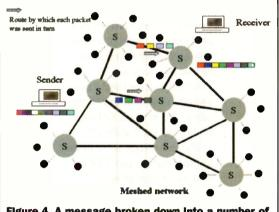
Figure 4. A message broken down into a number of equal sized packets for transmission using packet switching.
