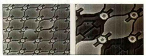
Complex MEMS system of array of independently actuated mirrors to control colour on a display module. Courtesy Texas Instruments
