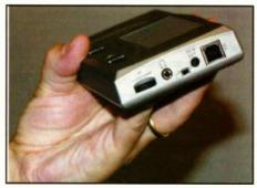
A side view of the Hango Personal Jukebox, showing the USB Interface across which MP3 tracks are transferred from a PC - and power/headphone sockets. No S/PDIF output for your hi-fl, though... Photo courtesy of Adrian Caspersz.
