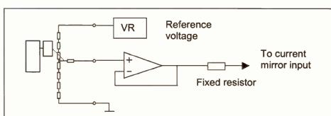
Figure 8. Block Diagram of Digital Controlled Potentiometer with Buffer to Give Wider Range or More Resolution of Control Current.
