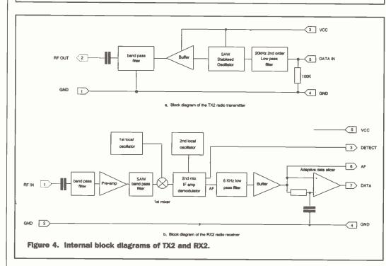
and 433MHz version, the operation voltage is between 2.2V to 4 V DC with a typical current consumption of 6mA at 3V. Digital data to be sent (which should be a CMOS logic level at the same power supply voltage) is fed into Pin 5. An antenna is connected to Pin 2. The block diagram of the module is given in Figure 4a.
