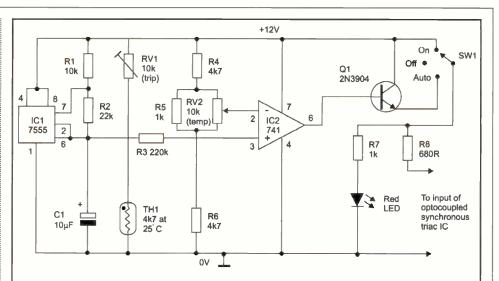
Figure 10. Fully automatic 'burst-fire' LED control circuit for use in the Figure 3 heater control system.
