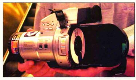
One of the most interesting digital stills cameras on view was the Sony MVC-CD1000., which dispenses with traditional flash memory or floppy discs. Instead, Images are stored on a special 8cm CD-R that has a capacity of 156MB capacity. Once the disc has been burnt, it can be read by a PC. We applaud Sony's efforts, but surely CD-RW would have been a more logical storage medium? Other features include a 10x optical zoom and a 2.1 megapixel resolution.
