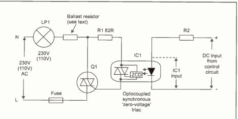
Figure 18. In extreme cases, such as in flashing-lamp disco displays, the main triac (Q1) can be protected against damage from a 'catastrophic' lamp failure by a ballast resistor, wired as shown.
