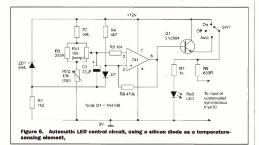
thus developed (via RV1) between the R1-ZD1 junction and pin-2 of the 741 op-amp, and a temperature-dependent voltage with a coefficient of -2mV/°C is developed between the R1-ZD1 junction and pin-3 of the op-amp. Thus, a differential voltage with a coefficient of -2mV/OC appears between pin-2 and pin-3 of the op-amp, which is wired as a high-gain (open loop) voltage comparator with slight hysteresis applied via R6.
