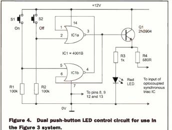
toggle switch that - when closed - connects the IC1 LED to the 12V DC supply via a 680R resistor that limits the LED 'on' current to about 15mA, thereby switching the electric load fully on.
