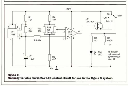
'Burst fire' AC power control principles
