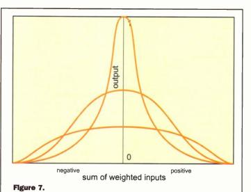
possible outputs as zero and one. However, by substituting the simple comparator with a slightly different bit of circuitry, analogue computations are possible. Two alternative types of artificial neurons which are commonly used have transfer functions of the forms shown in Figures 6 and 7.
