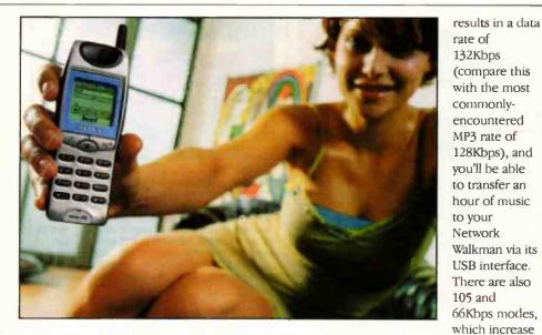
Cellphones equipped with WAP microbrowsers are proving popular, despite the inconsistency of the services that can be accessed. Here's the latest CMD-J5 model from Sony. This WAP-compatible handset features a voice recorder (as its LCD screen demonstrates), compatibility with HTML (yes, really!) and a thumbwheel for site navigation.
