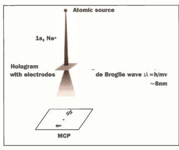
Figure 1. Schematic diagram of experimental setup. The atomic source, the hologram, and the screen of microchanical plate (MCP) were placed vertically.
