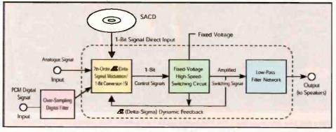
Block diagram, showing one channel of the Sharp SM-SX1 digital amplifier.
