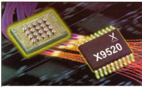
The explosive growth of the fiber optic communications market has created a fast growing market for Xicor's family of X9520 devices. The X9520 is targeted at controlling the laser diodes in fiber optic modules for Fibre Channel and Qigabit Ethernet. The X9520 integrates 3 digital potentiometers, 2k bit memory, and 3 voltages monitors that combine Xicor's EEPROM technology with mixed signal functions.
