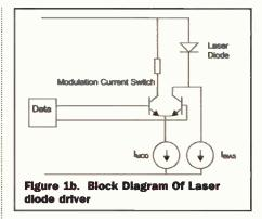
operating bias current of the diode, which in turn varies the output power. Further advantages for optical fibre communications are the high coupled power and cutoff frequencies allowing data rates in excess of 1Gb/sec.
