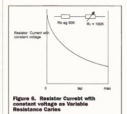
The use of resistors with discrete steps can potentially make the resolution overly coarse. The worst case is where the variable resistor is at a minimum (current maximum) as shown in Figure 6.
