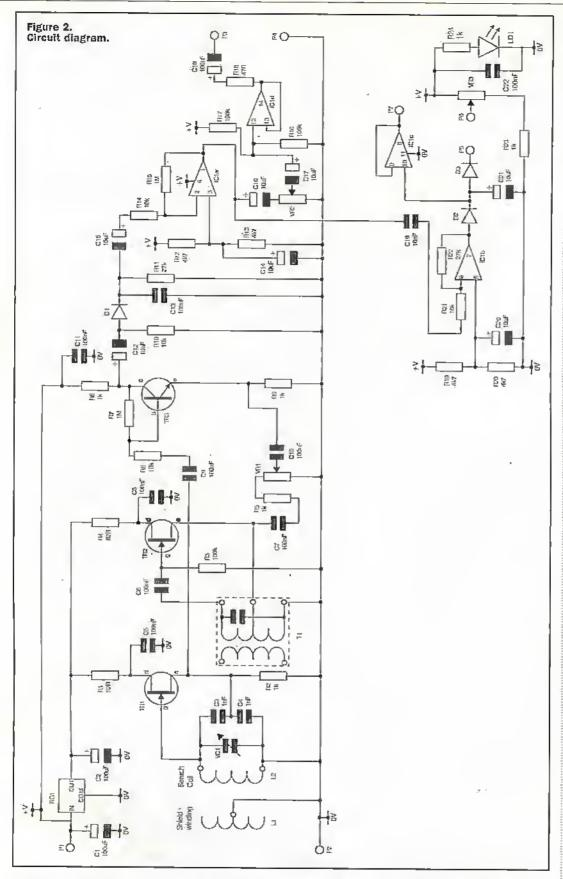
frequency is determined by tuned circuit T1, a standard IF oscillator tuning can with an integral capacitor. The operation of this stage is slightly different to the search coil oscillator as the feedback is applied directly to a tap in the inductor as opposed to using a capacitive tap.
