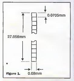
character size (dots) determines the number of heating elements used, see Figure 2. Print speed is normally 285 dots (20.1mm) per second.
