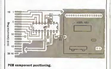
holding up the sandwich of artwork-board-artwork to a light source and lining up the two drill holes in line with the artwork. Secure with tape
