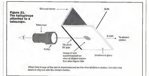
Rotating mirror on axis AB also rotates plane CD. Mirrors are rotated on axis AB until CD
