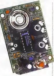
The circuit can be literally constructed in under 10 minutes. But before starting construction it is worth deciding whether you wish the sensor probes to be remote from the board and sounder, This can be up to two metres and so does provide some flexibility in any application, and Velleman thoughtfully provided a convenient 'break' point on the board so that the sensor
