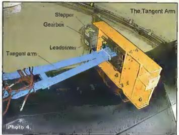
Direction defines the direction of rotation whilst a pulse on the step line moves the motor one 400th of a revolution. (They are 200 step per revolution motors and the drivers run in half-step mode).
