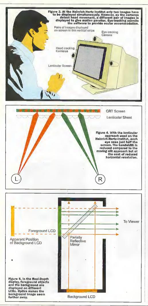
800Hz or one picture every 1.25ms. In fact, a CRT with this sort of refresh rate is one of the more demanding elements of this display method. Not only is ultra-fast electronics required - almost an order of magnitude faster than run-of-the-mill displays - but the phosphor must be ultrahright and have a very fast decay time.
