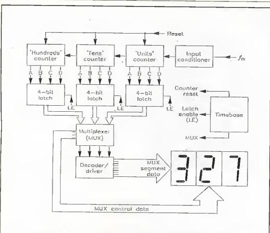
Figure 15. Realistic implementation of the multiplexing technique in a 3-digit frequency meter.
