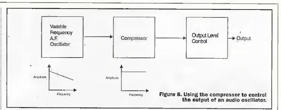
depend on the sensitivity of the microphone. When set up correctly, the compressor may improve the effectiveness of a communication link especially under weak signal conditions.
