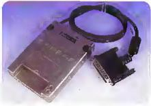
A SmartMedia and PCMCIA card reader and writer that simply plugs into a parallel port on the PC Install the drivers and the inserted card is displayed as an extra drive on your Windows system. A keyboard cable adapter is provided to supply power to the unit.
