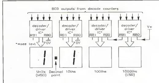
Figure 19. Ripple-blanking used to give trailing-zero suppression of the last two digits of a 31/r-digit DVM readout.
