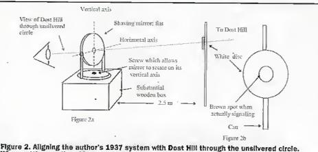
When setting up, the white disc is placed to obscure the view of Dost Hill through the unsilvered circle - Figure 2a. During signaling, the mirror is adjusted so that a beam of sunlight illuminates the white disc and the brown spot, caused by the unsilvered circle in the centre of the mirror, is maintained in the centre of the disc - Figure 2b.
