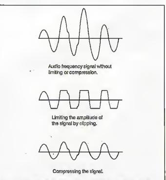
Figure 1. Simplified graphical comparison of signal clipping and compression.
