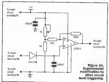
automatically start a recording device such as a cassette or digital recorder. Similarly the unit could be used to switch on a door phone or video camera when a visitor speaks into the microphone. If a continuous output is required the output from P7 can be used to drive a simple latch. This can be arranged so that the output remains active until the latch is reset.
