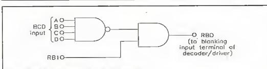
Figure 20. DIY ripple-blanking logic (active-high type).
