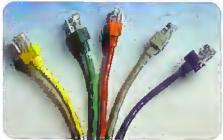
A range of UTP cross-over patch cables suitable for connecting two network cards directly to create a simple network, also suitable for connecting two hubs together when uplink ports are not available
