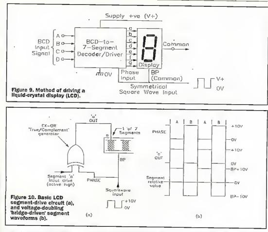
BR and in part B it is 10V negative to BR so the LCD is effectively driven by a squarewave with a peak-to-peak value of 20V but with zero de value. This form of drive is generally known as a voltagedoubling 'bridge drive' system. In practice, many LCD-driving ICs (such as the 4543B) incorporate this type of drive system in the form of a 7-section
