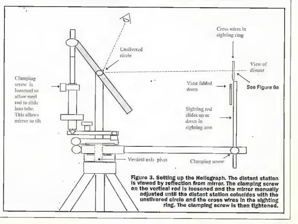
the sun; I then adjust the mirror so as to observe the distant station through reflection from the mirror. See Figure 3.
