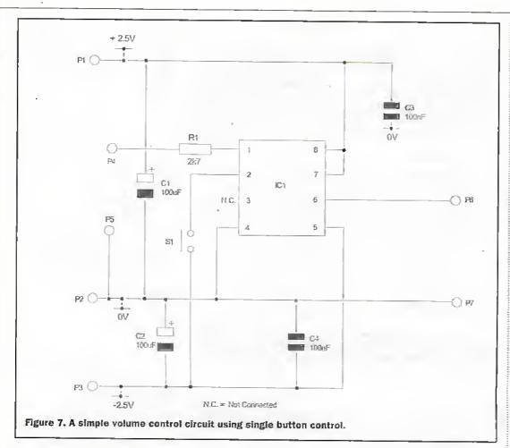
input signal is applied between P4(input) and P5 (0V) with the output available between P6 (output) and P7 (0V). It should be noted that the IC control inputs, to which S1 and S2 are connected are referenced to the –V supply. To prevent overload and possible damage to the IC, the input signal voltage swing should not be allowed to exceed the supply voltage.
