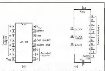
Figure 1. Outline and pin designations (a) and basic functional diagram (b) of the 4017B decade counter/divider IC.
