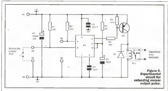
and in most cases it should be possible to power the unit from the same 12V supply as the microwave transmitter module. However, it is always wise to check the total current consumption to make sure that it is within the capability of the power supply used.
