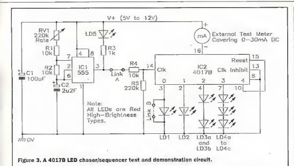
Note that the clocking signal is fed to the 4017B IC via removable Link A, and can thus be physically interrupted. whenever required; R4 and R5 protect the 4017B's input against damage when Link A is open or IC2's positive supply . connection is broken.
