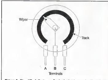
Figure 1. Simplified diagram of a typical rotary potentiometer.
