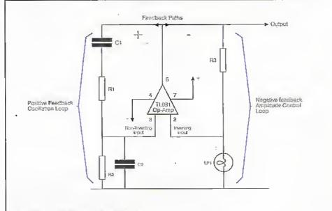
Figure 2a. Basic Wein Bridge Circuit.
