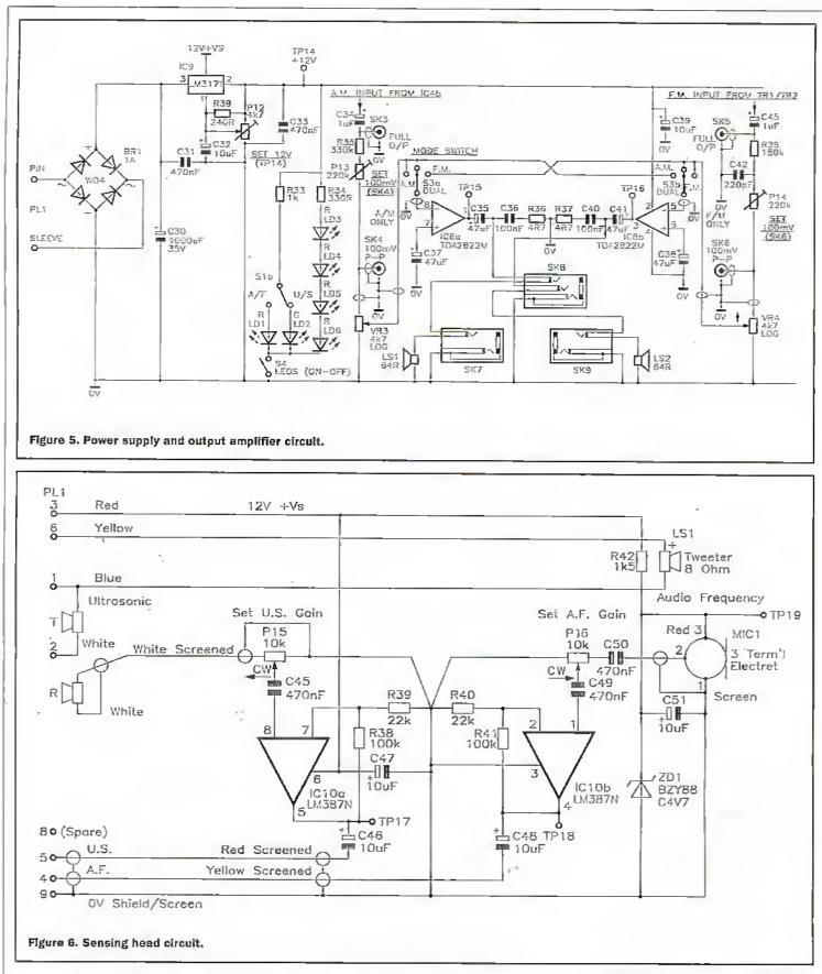
op-amp, the rest of which is used in the FM signal processing channel. The other input to IC7 is a gating signal. This is applied to pin 5 and can be used to vary the gain of the circuit, either by a fixed amount depending on the DC potential, in which case it can be used as an electronic attenuator or variable gain amplifier depending on the exact potential applied. If an AC signal is fed to this pin, as in the authors design, then the gain varies in sympathy with this signal and the chip
