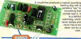
Power supply: 2 x 8VAC or 9 - 12VDC / 500mA · Choice of two different "dog sounds" · Reacts to surrounding noise with adjustable sensitivity · Speaker output : 2W at 4ohms · PCB dimensions : 142 x 75mm, 5.6" x 3"
