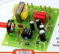
may be used as a free-standing amplifier with speaker, e.g. to listen to a telephone conversation, or the output may be connected to an amplifier or mixing panel (e.g. radio stations). The circuit is ideally suited for integration with the Velleman modular mixing panel.
