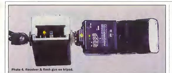
working tools and patience a shoe can be fabricated from a piece of 1 in, wide brass strip. When all else fails the foot of the flashgun can be taken apart and an additional 3-pole socket added in wherever there is space. Be aware that the internal generator in a flashgun may produce several hundred volts across a hefty capacitor; a nasty shock can be the result of not checking it is completely discharged prior to commencing work.
