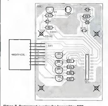
Figure 7. Component overlay for transmitter PCB.
