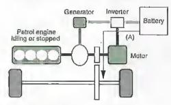
(A) Car propelled by electric motor.
