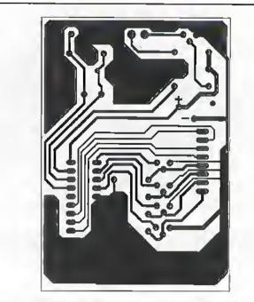
Figure 8. Underneath copper layer for transmitter PCB.
