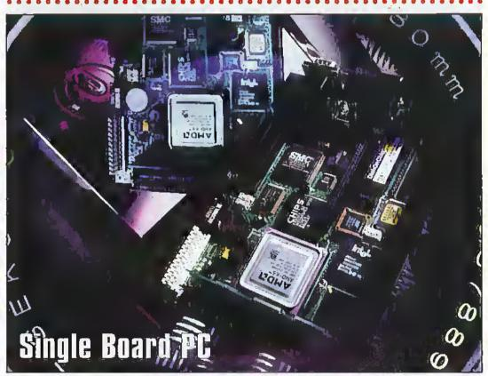
Blue Chip Technology has launched a powerful single board computer for audio, graphics and video applications. The 200MHz Pentium product has 64MB DRAM, 512KB L2 cache, an on-board SoundBlaster audio card and plug-in flash options for diskless operations.
