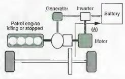
A renerative braking used to charge battery.
