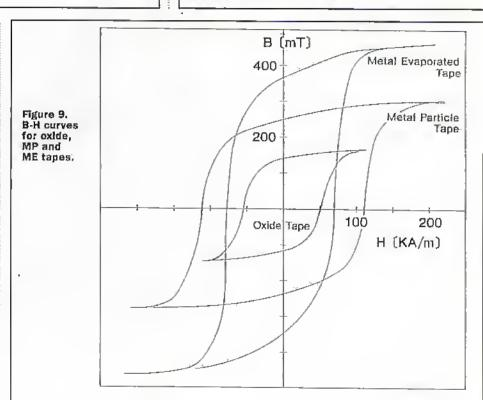
magnetism is required to reduce the magnetic flux density to zero. In the case of double layer tapes, the upper layer will have higher figures than the lower layer.
