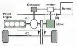
(D) If battery charge is low, engine power is used to generate electricity to charge battery.
