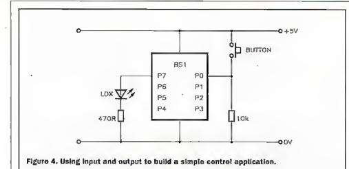
This program is intended to operate in conjunction with the circuit shown in Figure 4. It toggles (inverts) the state of an LED on pin7 when the active to low switch on pin0 is pressed. When the switch is held down, BUTTON waits, then rapidly auto-repeats the Toggle instruction, making the LED flash rapidly. When the switch is not pressed, BUTTON skips the Toggle instruction and the LED on pin7 is unaffected.
