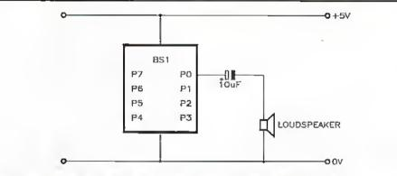
Figure 5. Connecting a loudspeaker to the STAMP to take advantage of the SOUND command.
