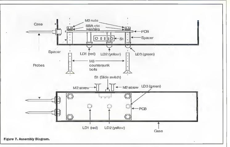
three level indication. When only the green LED is illuminated this indicates a dry (open circuit) condition. When the green and yellow LEDs are lit this indicates an intermediate condition where there is possibly some moisture present. When all three LEDs are illuminated there is a reasonable chance that the material under test has a significant moisture content. Under this condition, buzzer, BZ1 is also active.
