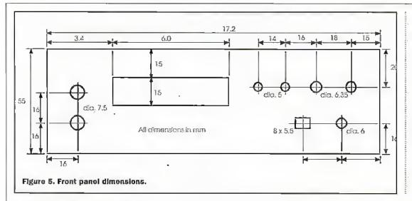
Drill the front and rear panels as in Figures 5,6. The PCB is held at one end using 14mm spacers from the base. Mount the spacers on the PCB and assemble to mark the locations for the holes in the base. The transformer bolts onto the base. There should be 5mm space all round.
