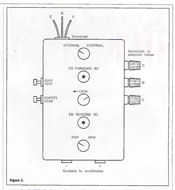
connected to the 'B' lead and set S2 to pnp. With S4 in EB position there will now be a forward current measurement. Now switch \$2 to npn, and \$4 in EB position, forward mode no longer indicates a reading, but \$3 in EB reverse does indicate a reading. Reverse the diode so that the cathode is now connected to 'E' letd, now S4 to EB will show conduction, but \$3 to EB does not. Set \$2 to pnp and \$3 to EB which will conduct and S4 to EB which does not. Remove the diode.
