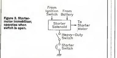
operating a hidden push-button switch. A small 'reminder' LED turns on when the engine is disabled by the immobiliser. This circuit thus gives a high level of protection, since it does not depend on the memory of its owner, and operates as follows.
