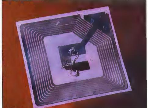
Photo 5b. Complete radio trequency Identification transponder manufactured in plastic.
