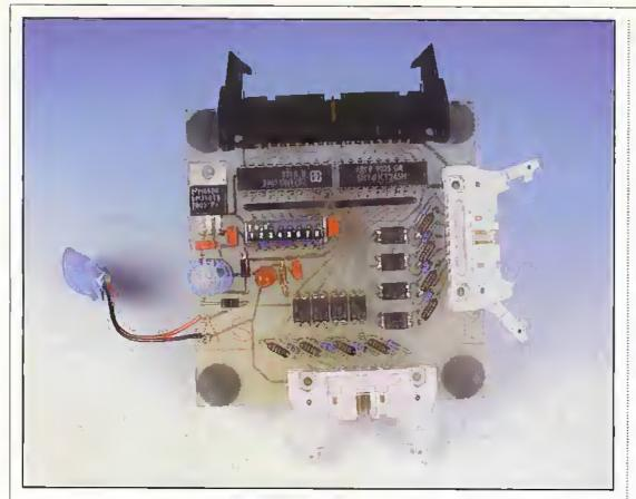
The light emitter and detector are physically spaced apart, usually by a few millimetres of plastic, which can provide electrical isolation up to several thousand volts. Because of these high ratings opto-isolators are used extensively in mains control systems, providing isolation between the "cold" low-voltage control circuits and the "hot" high-voltage mains switching circuits.
