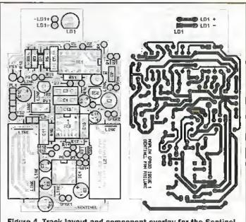
Figure 4. Track layout and component overlay for the Sentinel.
