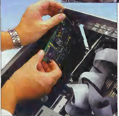
The PC's main board, called the motherboard because the smaller daughterboards plug into it, has a row of long expansion sockets at the back. You will see that some of these already have boards plugged into them. Your graphics card, sound card and possibly your 1/O and disk drive controller cards all plug in here.
