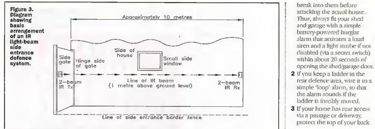
by a PIR alarm fitted with a 'corridor' type of lens, or by an IR dual 'light beam' alarm of the type described in Part 5 of this series; Figure 3 shows the basic arrangement of a suitable 2-beam IR light beam alarm system.
