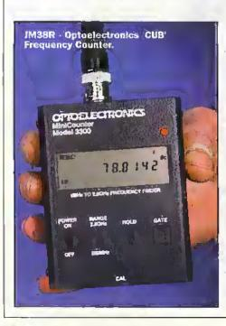
But if the frequency is not known you may think the only alternative is to search the bands and hope. Enter the frequency counter a useful hand-held device that is able to lock on to a local radio signal and display its exact frequency on a digital display.
