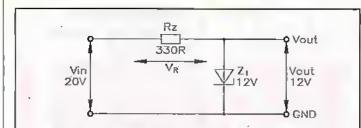
Figure 4. Zener diode is used to bring external voltage within operating parameters of the NE555
