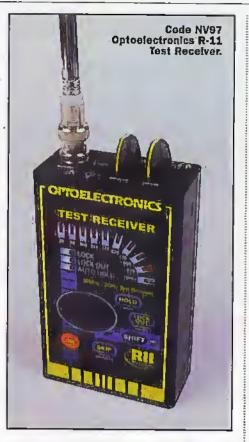
operation and a built in pager style vibrator to alert you when frequencies are recorded. It also has a distinctive double beep that informs you when a new frequency is found and a single beep indicating that a previously recorded frequency has been hit again. A 16 section bargraph is on the LCD front panel display which provides a real time relative indication of RF signal strength. The optional PC interface 'OPTOLINX' permits down loading of stored information on a PC.
