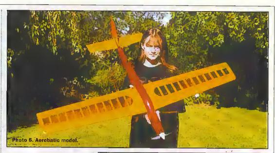
propeller and this speed controller using STP60N06-16 MOSFETS, and an own design acrobatic model using a Maplin MRI 19 triple wind motor<sup>1</sup> (GZ22Y) driving a 6" by 6" propeller and this speed controller using IRL2203 MOSFETS. Both use 7 cell 1700/2000 battery packs.
