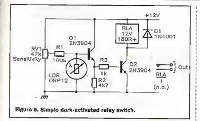
When light enters the normally dark area and falls on the LDR face, however, the LDR resistance falls to a fairly low value and base-bias is applied to Q1, which thus turns on and activates the relay and its RLA/L contacts, which can be used to control external circuitry. The relay can be any 12V type with a coil resistance of  $180\Omega$  or greater.
