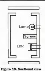
of a reflection-type smoke detector. top. The inside of the box is painted matt black, and the construction lets air pass through the box but excludes external light.
