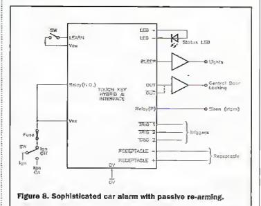
Module's LEARN input causes passive re-arming to occur.
