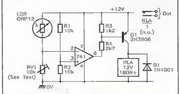
Figure 10. Precision light-activated relay switch.
