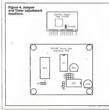
connecting wires are used. IC2 provides diode clamps to both supply rails for ESD and spike protection. IC2d provides an effective internal pull-down of 15K.
