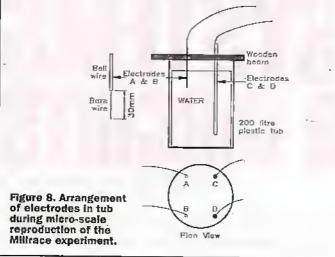
electrodes were cleaned with a plastic scouring cloth; this completely inhibited polarisation and it took several weeks of exposure to the air before it would reoccur. Indeed, after scouring, the charge held was found to be in direct ratio to the length of time the electrodes were exposed to air. So presumably, oxidation has some effect on polarisation, Scouring had no effect on the carbon electrodes, in any case, carbon oxides are gases.
