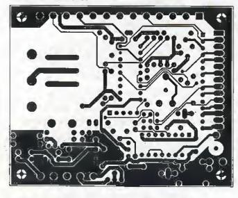
Figure 7. Track layout and component overlay for the Touch Hybrid Interface.
