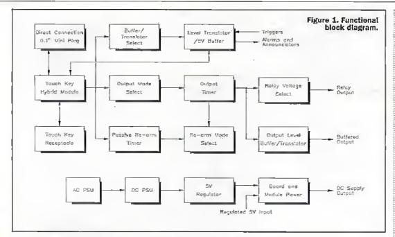
Regulator can be bypassed with an external regulated 5V supply. Alternatively, the pre-regulator and regulated inputs can be used as outputs to supply external components.
