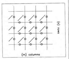
Figure 1. Part of an m × n keyboard matrix, showing positions of keyswitches on the row/column intersections.
