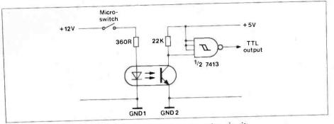
Figure 10. Using an opto-isolator to couple digital data between two circuits.
