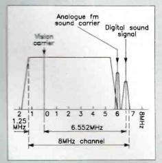
Figure 1. The frequency spectrum occupied by the NICAM 728 digital sound signal in relation to the vision and FM sound signals (UK System I). (Vertical axis not to scale.)
