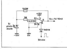
Figure 12. The silicon photo-diode used to measure light level. Good linearity exists between output voltage and ambient light level. The response is fast too.
