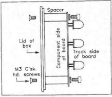
Figure 6. Installing the PCB.
