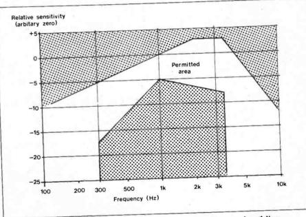
Figure 11. The telephone sensitivity must lie within these limits for a zero-length line.
