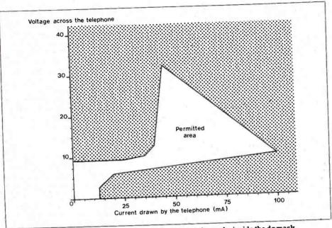
Figure 10. The voltage and current in the telephone must always be inside the dc mask.
