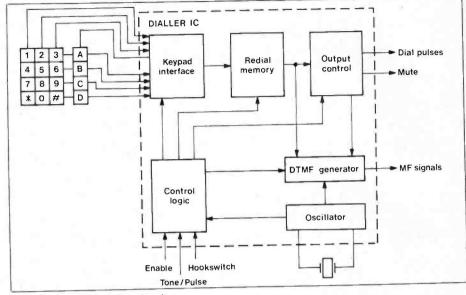
Figure 7. A typical dialler circuit.
