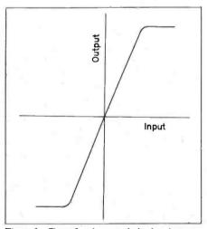
Figure 1c. Transfer characteristic showing peak clipping.
