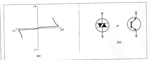
Figure 3. The diac, (a) characteristics, and (b) possible circuit symbols.
