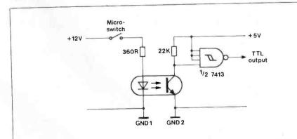
Figure 9. Using an opto-isolator to interface a microswitch to a digital circuit, avoiding "ground noise" problems.
