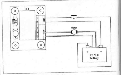
Figure 1. Wiring diagram for motor/most applications.
