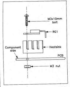
Figure 6. Assembly of regulator and heatsink.
