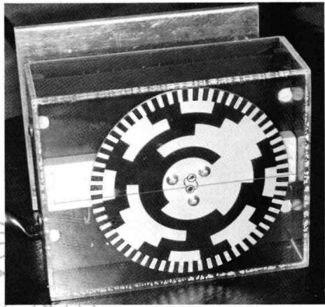
**P**hoto 5. An example of a digital shaft encoder, in this case a 5-bit type, as is evident from the five concentric rings.
