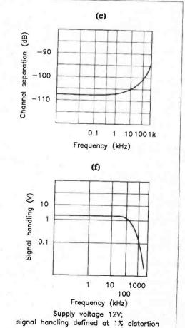
Figure 2 (a) Supply Current vs Supply Voltage, (b) Supply Current vs Temperature, (c) Channel Separation vs Frequency, (d) Attenuation of Caselected Inputs vs Frequency, (e) THD vs Frequency, (f) Signal Handling vs Frequency.
