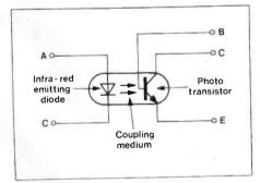
Figure 8. The optically-coupled isolator (opto-coupler or opto-isolator).
