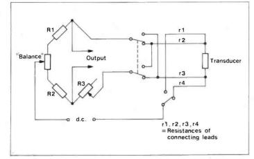
Figure 5. The Mueller bridge, used when long connecting leads are involved.
