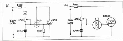
Figure 5. (a) Half-wave phase-control circuit using SUS to trigger a SCR, (b) full-wave phase-control circuit using diac to trigger a triac. Both circuits use single time constants.
