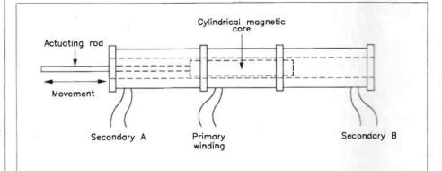
Figure 6. Basic construction of a Linear Variable Differential Transformer (L.V.D.T.)
