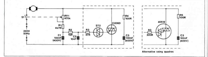
Figure 10. Two possible circuits for controlling the speed of a small universal motor. Either a diac/triac combination or a quadrac can be used.
