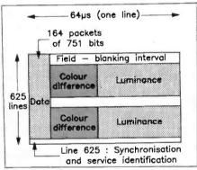
Figure 7. The structure of 625 line MAC/ packet frame, showing the time-division relationship between digital data (at the rate of 20.25Mbit/s for D-MAC) and the vision signal. The data is structured in the form of packets containing 751 bits, carried at the rate of 4,100 packets per second.
