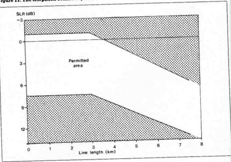
Figure 12. The send loudness rating (SLR) must be between specified limits.
