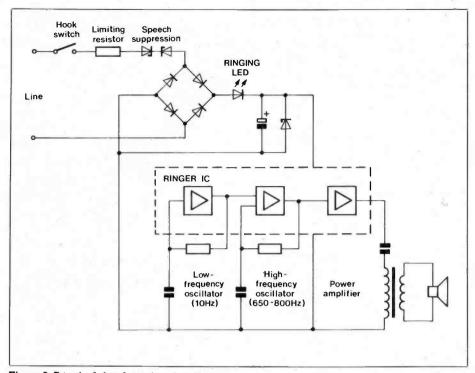
Figure 2. A typical ring detection circuit.
