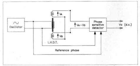
Figure 7. A polarity-sensitive output, proportional to linear displacement, can be obtained from a L.V.D.T. using a 'phase sensitive detector'.
