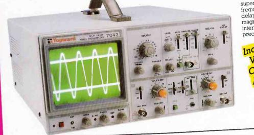
As above, but with 40MHz bandwidth and super bright 12kV tube even at the highest frequencies. This instrument also has a delayed sweep time base to provide magnified waveforms and accurate time interval measurement. Truly superb precision instrument.
