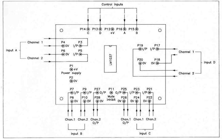
Figure 5. Wiring Diagram.
