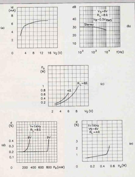
Figure 2. Electrical characteristics. (a) Quiescent current vs Supply voltage. (b) Supply voltage rejection vs Frequency. (c) Output power vs Supply voltage (THD = 10%, f = 1kHz stereo). (d) Distortion vs Output power (stereo). (e) Distortion vs Output power (stereo).
