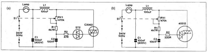
Figure 9. Two alternative lamp dimmer circuits, (a) using a diac and triac, (b) using a quadrac.
