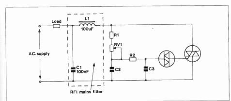
Figure 6. Double time-constant phase control circuit, with filter (L1 and C1) to eliminate RFI. October 1989 Maplin Magazine
