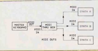
Figure 2. Connecting synthesisers using MIDI Thru' Box.
