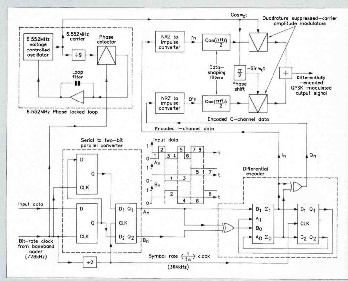
Figure 4. NICAM 728: Block diagram showing the processes of differential encoding, data-signal shaping and modulation at the transmitter.
