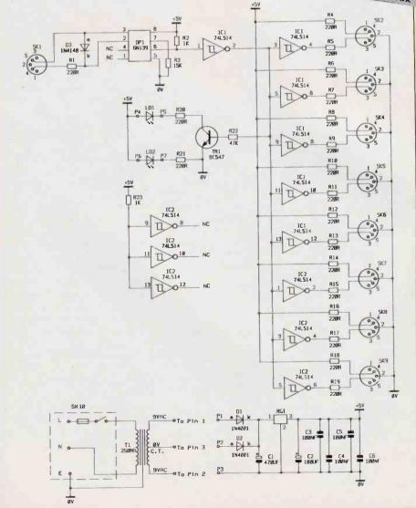
Figure 3. Circuit diagram of MIDI Thru' Box.
