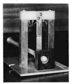
Photo 1. A single strain gauge attached to a member under test in loading jig.
