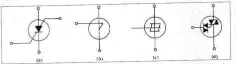
Figure 4. Circuit symbols for four members of the thyristor family. (a) SCS (b) SUS (c) SBS and (d) quadrac.
