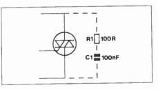
Figure 7. RC 'snubber' circuit to avoid accidental dv/dt triggering when the load is inductive.
