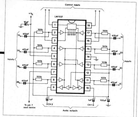
pins (pin 7) of the devices together and connecting the two pairs of output pins (pin 9 and pin 10) in parallel. It should be noted that only one output capacitor is required for each channel.
