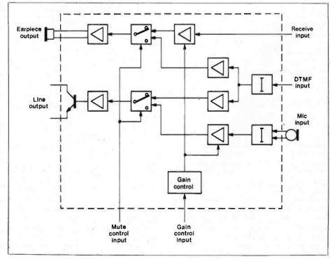
Figure 5. Block diagram of speech IC (simplified).
