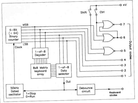
Figure 2. A scanned keyboard.
