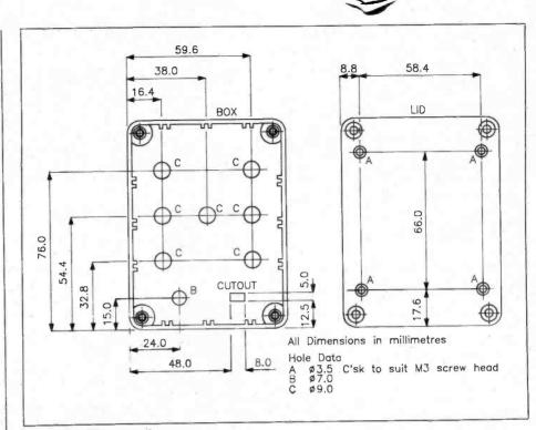
Figure 5. Drilling Details.
