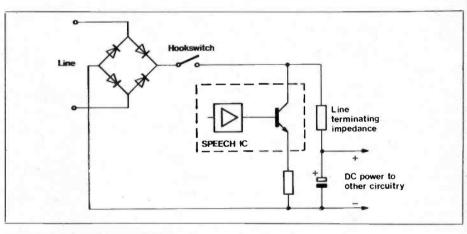
Figure 4. Line impedance matching and power extraction.
