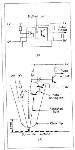
Figure 11. (a) Principle of optical coupling applied to the generation of pulses by a rotating, slotted disc (e.g. to measure engine speed), (b) Using a LED and a photo-Darlington amplifier to read bar codes.
