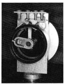
Photo 4. Example of large wirewound (rotary) potentiometric transducer.
