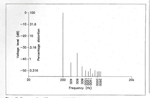
Figure 2b. Spectrum of amplifier output with 200Hz sine wave input showing harmonics up to the 13th.
