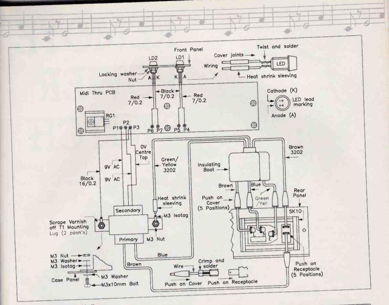
Figure 8. Wiring and assembly diagram.
