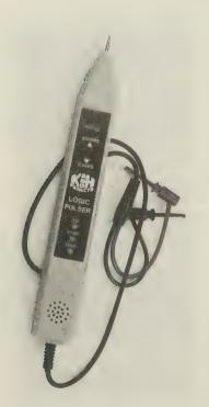
Photo 15 CMOS/TTL logic pulser which may be used to inject pulses into digital circuits. This device is similar in appearance to a logic probe. Maplin order code: YU56L (matching logic probe, Maplin order code: FY73Q)
