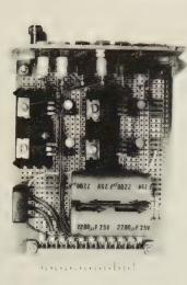
Photo 3 A simple dual-rail power supply based on 78 and 79 series regulators. The power supply is built on a matrix board (see Chapter 10). Note the heatsinks fitted to the regulators the device incorporates safe operating area protection as well as input overvoltage protection (up to 60 V, 10 ms) and short-circuit protection.
