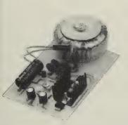
Photo 24 Pre-amplifier/ general-purpose power supply module
