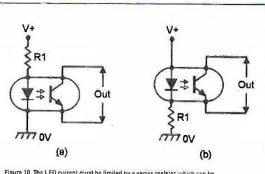
Figure 10. The LED current must be limited by a series resistor, which can be connected to either the anode (a) or the cathode (b).
