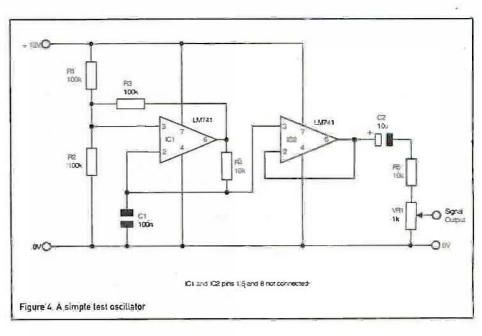
may be mounted on the same circuit board as the amplifier or wired externally. The leads to the potentiometer should be kept as short as possible to minimise unwanted noise pickup.
