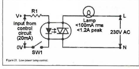
of a normal LED, and the SCR/triac is used like a normal low-power SCR/triac. Figures 21 to 23 show various ways of using an optocoupled triac; R1 should be chosen to pass a LED current of at least 20mA; all other component values are those used with a 230V AC supply.
