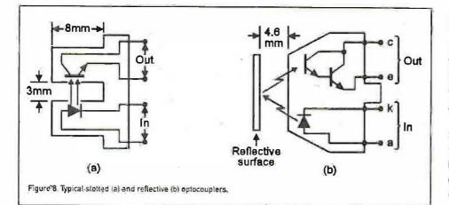
for the slotted and reflective optocoupler devices of Figures 8. The Figure 8(a) device
