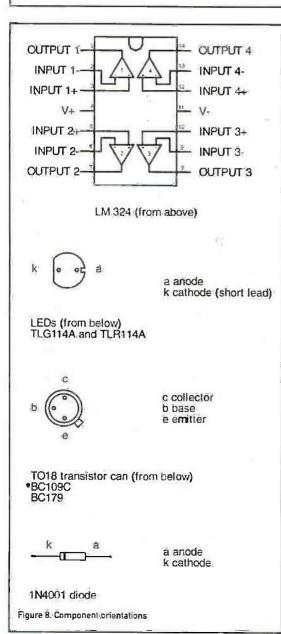
The correct orientation of the transistors, diodes and LEDs, and electrolytic capacitors needs to be observed. The polarity of an electrolytic capacitor is marked on its cover; figure 8 gives details of the physical configuration of the other components.
