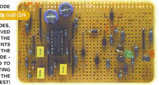
The oscillator generates a square wave at approximately 2 kHz to provide the test signal that is applied to the diode.
