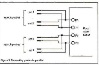
With insulating spacers. Under normal conditions the two contacts must be high resistance. Any leakage may trigger the alarm. Specially designed cables are available for use with flood alarms.
