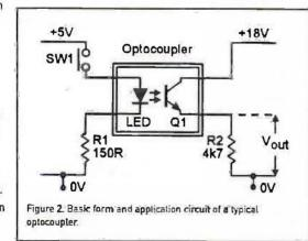
through the LED via R1, and the resulting, light falls on Q1 face, causing the phototransistor to conduct and generate an output voltage across R2.
