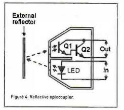
specifying optocoupling efficiency is to quote the output-to-input current transfer ratio (CTR) of the device, i.e., the ratio of the output collector current (IC) of the phototransistor, to the forward current (IF) of the LED. Thus, CTR = IC/IF. In practice, CTR may be expressed as a simple figure such as 0.5, or (by multiplying this figure by 100) as a percentage figure such as 50%.
