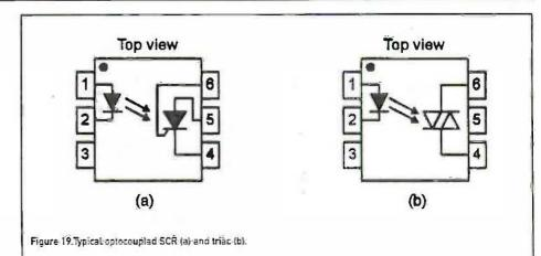
300mA for the SCR and 100mA for the triac. The SCR device's surge-current rating is 5A at a pulse width of 100?S and a duty cycle of less than 1%: the triac device's surge rating is 1.2A at a pulse width of 10?S
