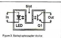
the LED and the phototransistor (which usually operate in the infra-red range) are always closely matched spectrally, The most convenient way of
