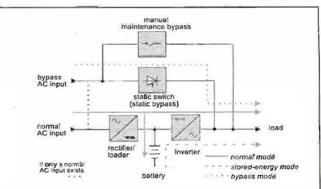
Figure 5. UPS with the double-conversion topology. The inverter is connected in series between the AC input and the load. Power for the load flows continuously through the inverter.
