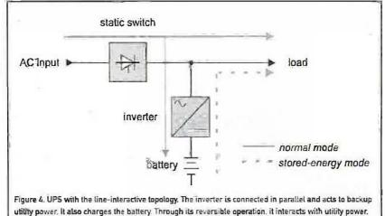
tolerances or fails, the inverter and battery continue to support load power. The UPS runs in stored-energy mode for the duration of the stored-energy time or until the AC-input supply returns to within UPS preset tolerances, at which point the UPS returns to normal mode.
