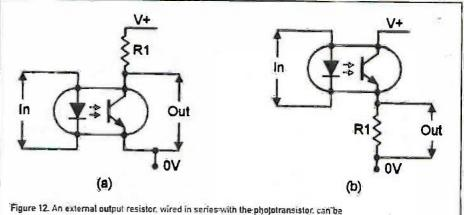
connected to either the collector (a) or emitter (b).
