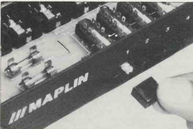
Photo 12. Fit rectangular buttons on to switches.
