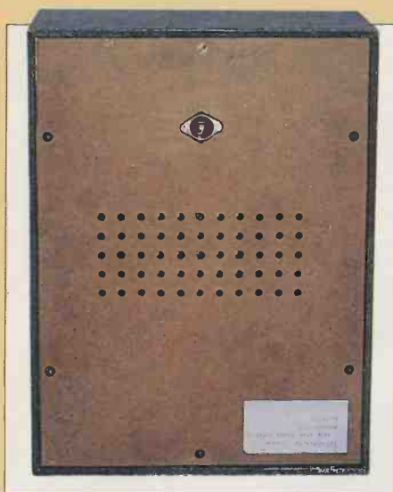
Photo 4. Back view of the basic 'unit stereo' loudspeaker, showing the perforated back; the perforations are an attempt to stop the back 'drumming', but are ineffective if the box is hung on a wall.
