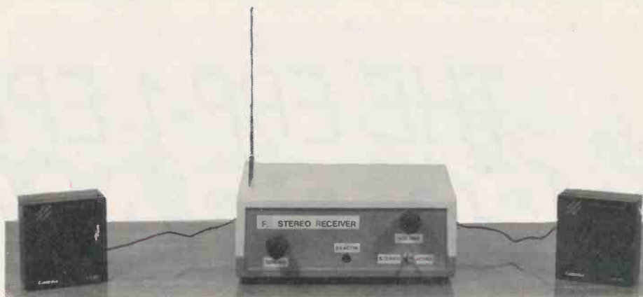
Photo 5. The completed conversion with whip aerial extended and using the Personal Speaker Set, available from Maplin as item YP64U.
