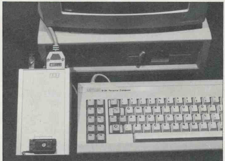
The EPP-1 in action, programming an EPROM.
