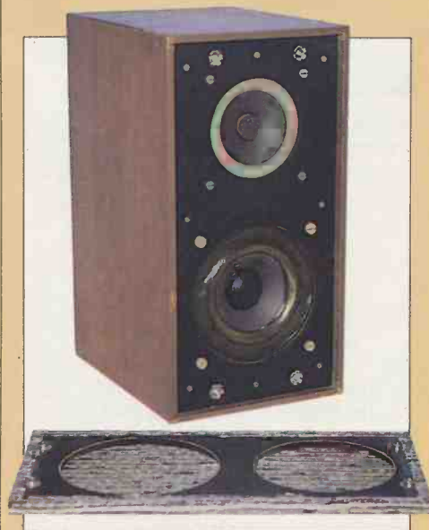
Photo 2. The 'Maxim' with the grille removed, to show the 100mm bass driver and the 70mm tweeter. The front panel of the enclosure is a steel plate.
