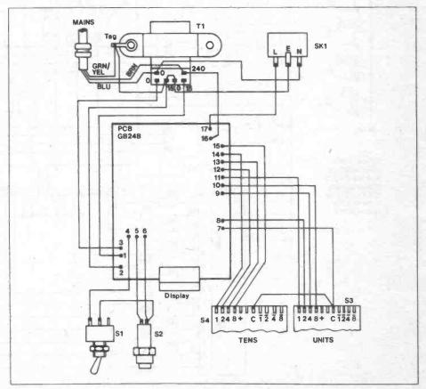
Figure 3. Interwiring diagram.
