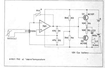
Figure 5. A 'frost alarm' for a car.
