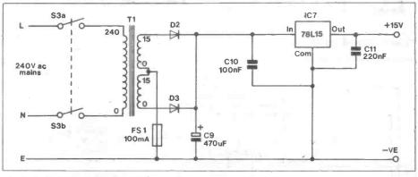
Figure 5. Mains power supply circuit.
