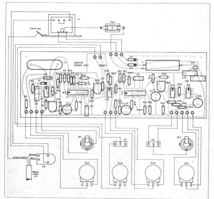
RV3 is given a setting that gives an unclipped output signal at pin 7 of IC3, and the setting of this component will probably not be very critical.
