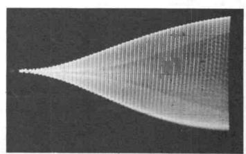
The response of a 6dB/octave high pass filter.
