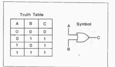
Figure 5. Two input OR gate.
