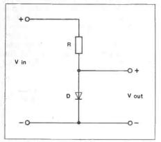
Figure 3. The basis of a log amplifier.
