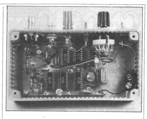
resistor and a parallel ceramic capacitor. TR1 is a UHF transistor with a very high ft. In its collector is a 1N914 diode, a non-linear load, which generates harmonics. Finally the RF output is taken via 10pF ceramic capacitor, C3, to both a BNC connector and a terminal post, thereby offering a choice of connection.
