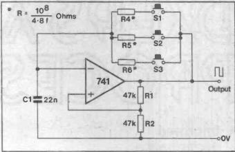
Figure 6. Circuit to detect presence of water.
