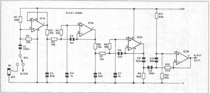
Figure 2. Circuit diagram of the filters.
