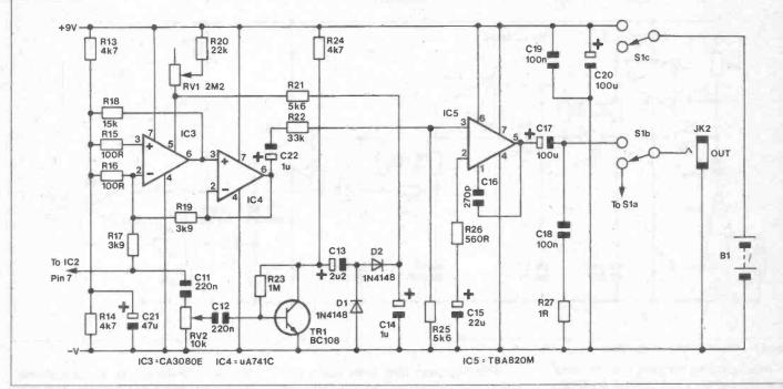
Figure 4. Circuit of the expander and output stages.
