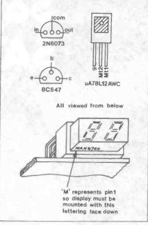
Figure 4. Pin configurations.
