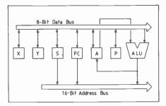
Figure 1. Simplified Architecture of the 6502.
