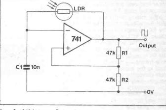
Figure 1. Basic astable waveform generator.
