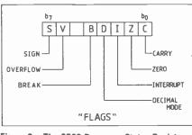
Figure 2. The 6502 Processor Status Register.
