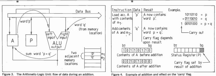
Figure 3. The Arithmetic-Logic Unit: flow of data during an addition.
