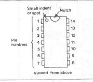
Figure 1. 14-pin dual-in-line (DIL) package.
