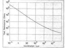
Figure 3. Characteristic of typical small photoconductive cell (LDR).
