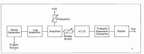
Figure 1. The simple sweep generator block diagram.
