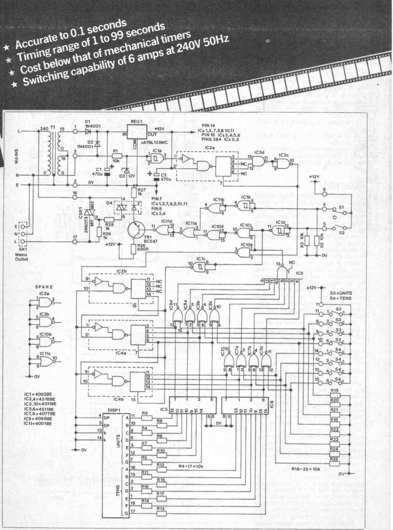
When the values of BCD input are the same the output is high. IC9 is an 8 input NAND gate giving low output on pin 13 only when all of the 8 BCD input pairs are the same. It is this output which controls the counting and also the output circuitry when S1 and S2 are in their off positions. The output of IC9 is over-ridden by the logic levels derived from S1 or S2 when either switch is used.
