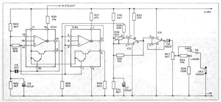
Figure 4. The VCO, waveform converter, and buffer amplifier circuits. 10
