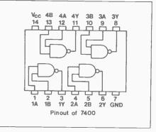
Figure 8. Quad two input NAND gate.
