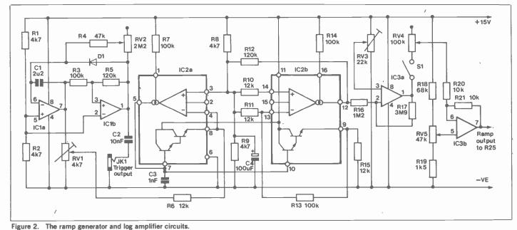
swept across the screen as the oscillator is swept over the audio frequency range. The spot can either be swept across the screen using triggered sweep with the trigger signal being obtained from the sweep oscillator, or the ramp signal from the sweep oscillator can be fed to the X input of the oscilloscope.
