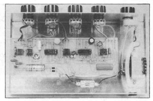
clipping circuit to round off the waveform to give the desired shape. In this circuit a soft clipping circuit is used, and one of the oscillographs shows the effect of this circuit. A buffer stage is used at the output of the unit to give a low output impedance.
