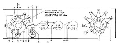
Fig. 12 Front Panel Wiring for Oscillator 1
