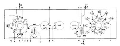
Fig. 13 Front Panel Wiring for Oscillators 2, 3 & 4
