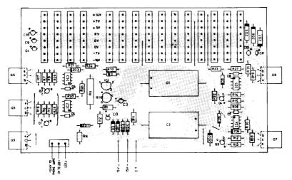
Fig. 2 Component Overlay for Power Supply
