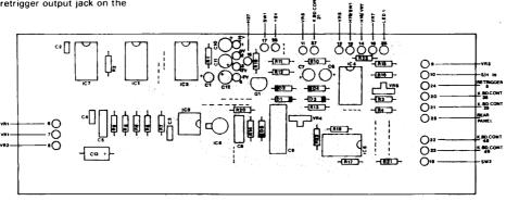
Fig. 17 Component Overlay for Sample and Noise
