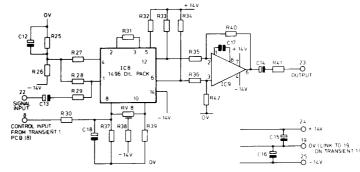
Fig. 23 Circuit Diagram of VCA Used In Envelope
