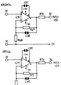
Fig. 44 Circuit Diagram of Joystick Controls
