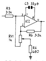
Fig. C Equivalent circuit of the equaliser with the potentiometer set for unity gain regardless of frequency.
