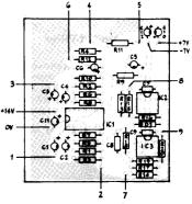
Fig. 48 Component Overlay for External Inputs
