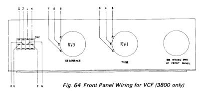
wiring to SW1 and SW3. Fix the assembly to the front panel.
