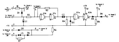
Fig. 34 Circuit Diagram of Transient Retrigger
