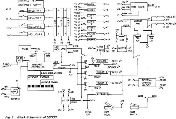
Transient 'A' for right output and patchboard for left output. Also control inputs may be coupled together so that a voltage from the patchboard may be used to control simultaneously the panning of left output from channel 1 to 2, and right output from channel 2 to 1. Note that it is the outputs that are panned between the two channels and not vice versa.
