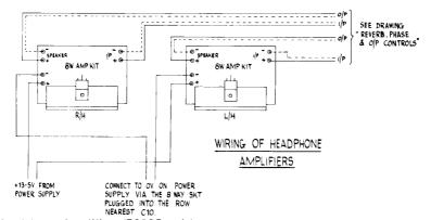
Fig. 57 Wiring of Headphone Amplifiers (5600S only)
