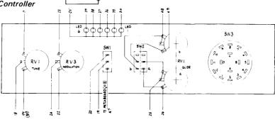
Fig. 8 Front Panel Wiring for Keyboard Controller
