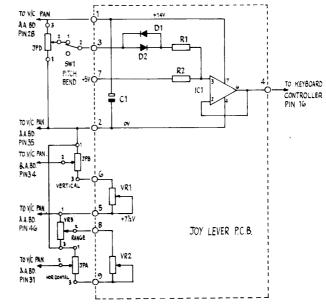
Fig. 46 Circuit Diagram of Joy Lever
