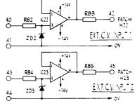
Fig. 42 Circuit Diagram of External Control Voltage Inputs
