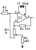
Fig. B Equivalent circuit of the equaliser with the potentiometer set for maximum cut at the resonant frequency of the network.
