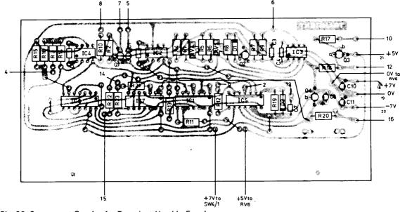
Fig. 20 Component Overlay for Transient Used In Envelope 24
