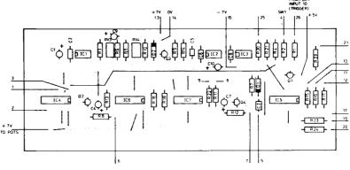
Fig. 29 Component Overlay for Transient 'A/B'
