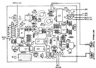
Fig. 35 Component Overlay for Reverb and Phase
