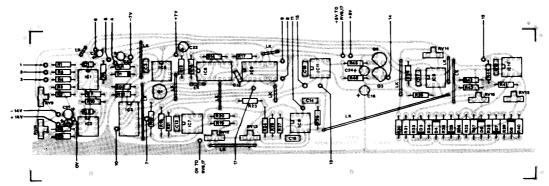
Fig. 9 Component Overlay for Oscillator
