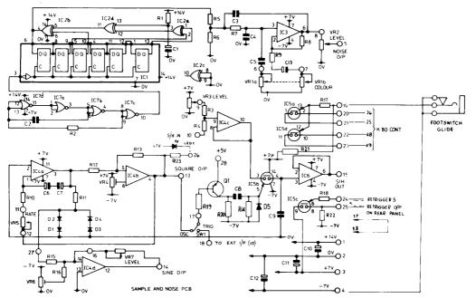
Fig. 60 Circuit Diagram of Sample and Noise (3800 only)
