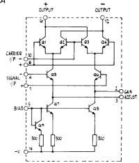
Fig. 28 Internal Circuit of MC1496
