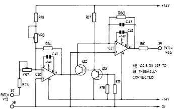
Fig. 43 Circuit Diagram of Exponential Converter
