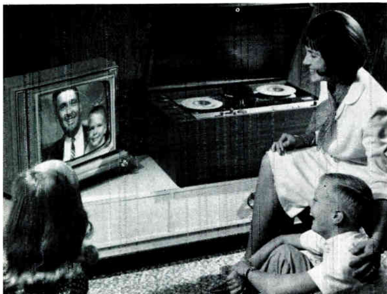
Fig. 6. This home video recorder unit—the 6200 HVR—will record programmes off the air, or pictures from a simple television camera, and will play them back (including a sound track) on most domestic television sets
