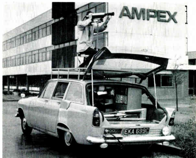
Fig. 5. A video recorder similar to that illustrated in Fig. 4 is here shown installed as part of a mobile recording system. The equipment also includes a camera unit, monitor screen and control apparatus
