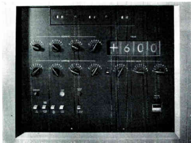
Fig. 11. This operator's control panel enables information to be obtained from, and instructions to be inserted into, the computer
