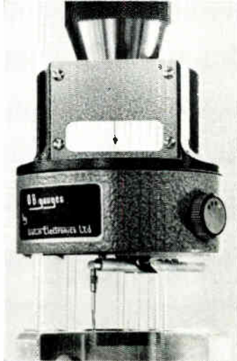
The 2½-lb OB Centre Locator which, when mounted by its ½-in. diameter paralleled shank in a drill chuck or collett, will gauge internal and external diameters ranging from ⅜ to 6 in.
