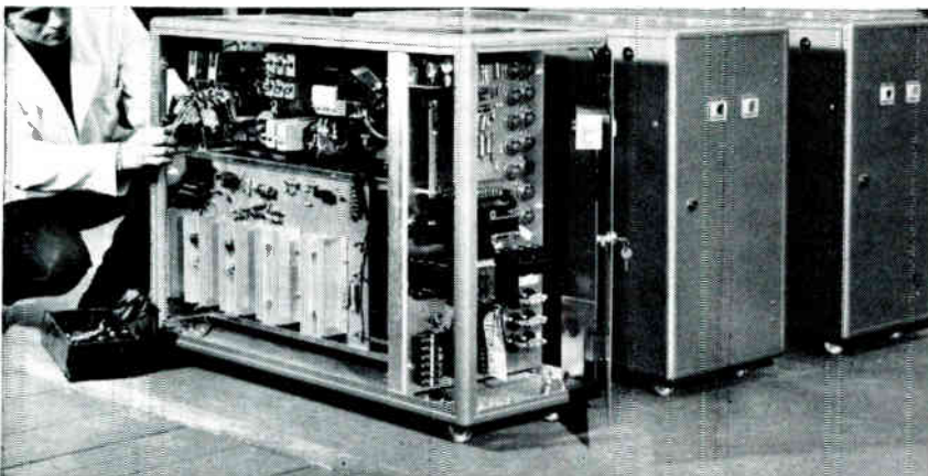
Castor-mounted Emotrol equipment currently being produced by AEI for the control of d.c. motors in flat-bed knitting machines.
