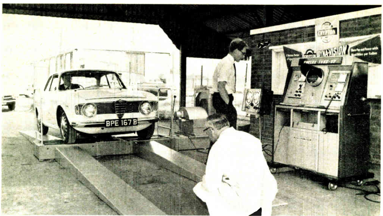
By invitation, Crypton Equipment (M.I. Group) provided full engine tuning facilities at Silverstone for a recent demonstration of imported cars. The picture shows an Alfa Romeo being guided on to the 'Road-Load' dynamometer for a high speed test. The eight Alfa Romeo models on view were all Crypton tuned before the demonstration
