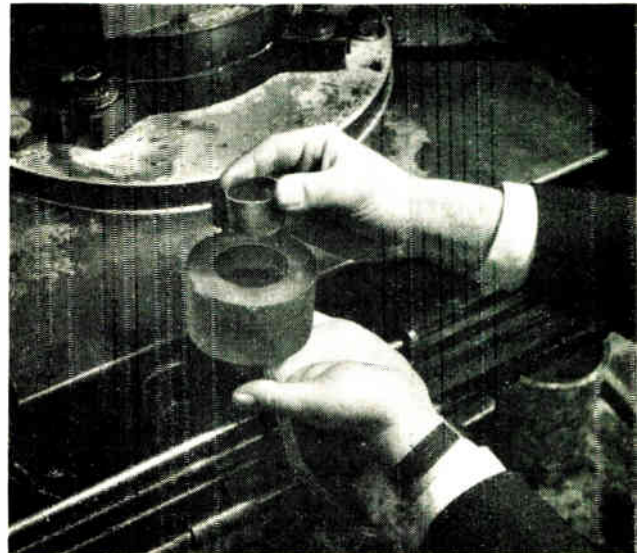
Fig. 2. The inductance coil of the tool alarm unit, potted in epoxy resin to fit the bolster of the press
