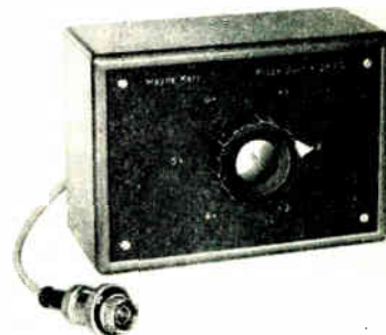
6-way Coaxial Switch JB731 for probe selection
