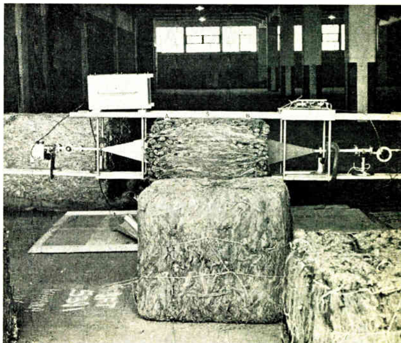
This illustration shows the application of the meter to the investigation of bulk tobacco
