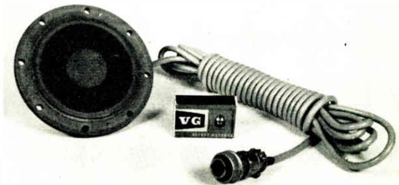
Ultrasonic transducer/transmitter unit for liquid level measurement in large storage tanks
