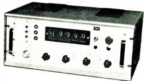
This shows one of the two digital voltmeters which are to be featured by Digital Measurements. Both models provide 5-digit, in-line readout plus polarity indication, binary coded output signals and 6 modes of operation; the total conversion time is 20 msec. Model DM2020 (63), illustrated here, has an accuracy of 0.01%, a sensitivity of 10 \mu V, a range from 0.19999 to 1999.9 V and a maximum input impedance of >10,000 M \Omega
