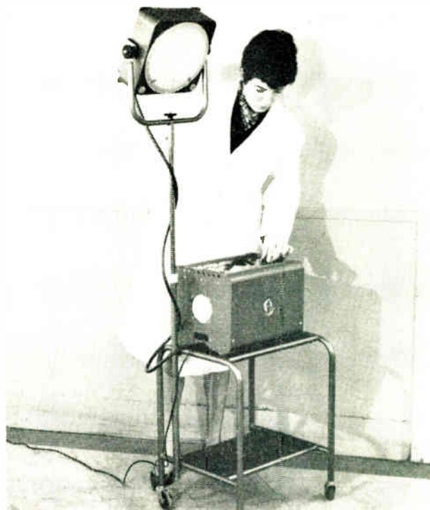
The picture shows a trolley with a built-in lamp standard for the E.M.I. Electronics Ltd. stroboscope type 6. This has a xenon discharge tube and a range of 300-60,000 flashes a minute
