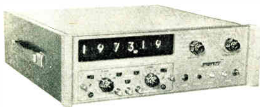
For the accurate measurement of frequency, time interval, period, phase lag and ratio Rank Cintel are showing this Systron model 1032 counter-timer. Ranges covered include frequency, 0 c/s to 2.5 Mc/s; period 1 \mu sec to 10 sec; time interval 1 \mu sec to 10 sec; ratio A : B = 10^6 max (input A = 0 to 2.5 Mc/s, input B = 0 to 1 Mc/s) (55)
