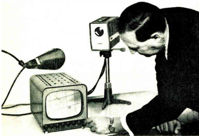
The author adjusts receiver controls as the E.M.I. type 8 closed-circuit television camera, without using a lens, transmits a picture of a transparency mounted in direct contact with the fibre optic window of the type 9686 tube
