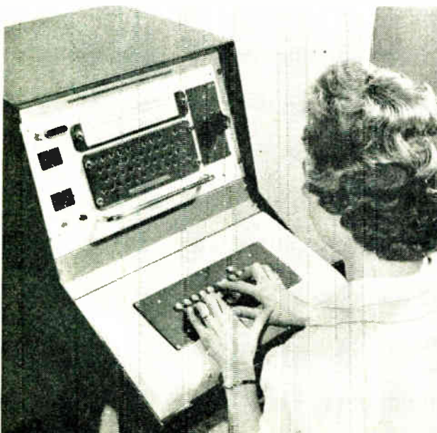
Close-up of keyboard and display panel of SAKI for training I.B.M. card-punch operators
