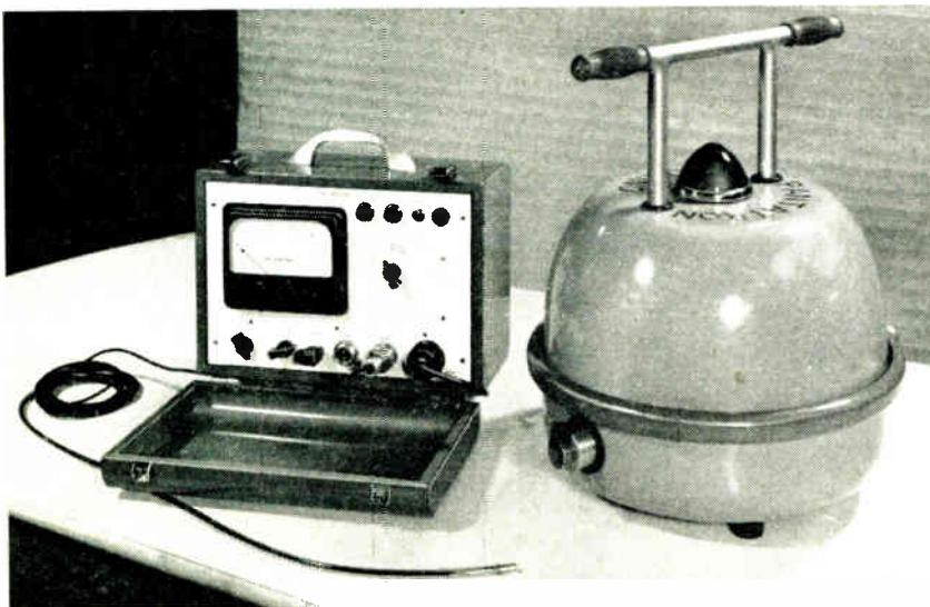
Apparatus using solid-state detectors for positioning of radioactive sources. (Pantatron Limited)
