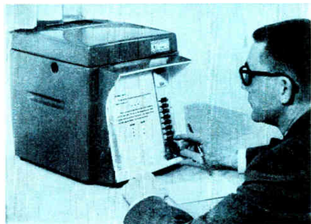
The AutoTutor being demonstrated by Mr. Norman Crowder, who developed the intrinsic programming technique used in this teaching machine
