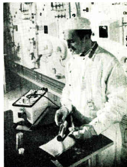
Left: The Mobile Radiography Unit of the Central Electricity Generating Board uses Type 255 Radiation Monitors in decontamination checks after leak tests in power station piping with radioactive sources
