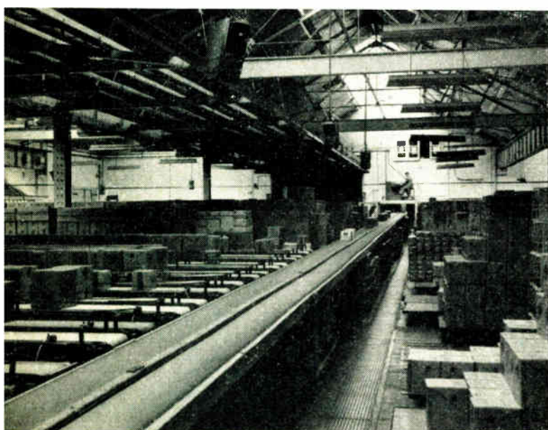
A common industrial application of counters is in counting packages on conveyor belts. An Allen West counter can be seen with its operator at the far end of the belt
