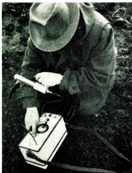
Left: The Mobile Radiography Unit of the Central Electricity Generating Board uses Type 255 Radiation Monitors in decontamination checks after leak tests in power station piping with radioactive sources
