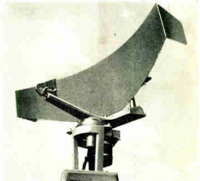
The 6-ft scanner which has a beamwidth of 1.2^\circ . It can be driven by a \frac{1}{2} -horse power motor and maintain normal performance in relative wind speeds of up to 80 knots
