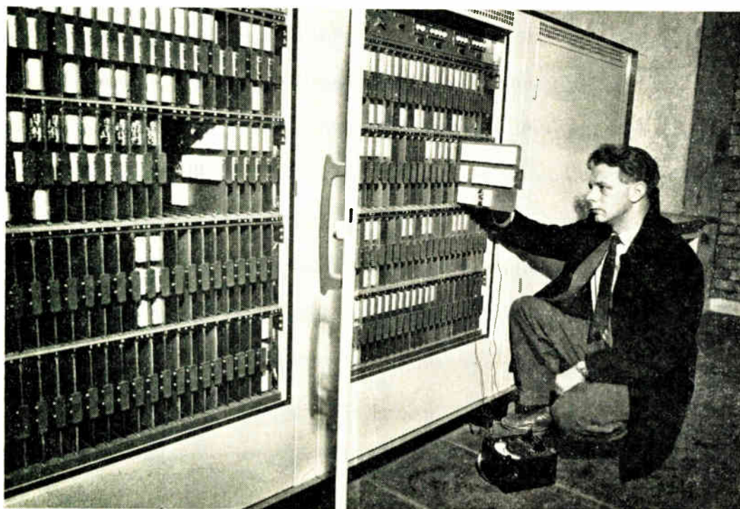
◀ This photo shows one of the scanners with its doors open to show the logical units
