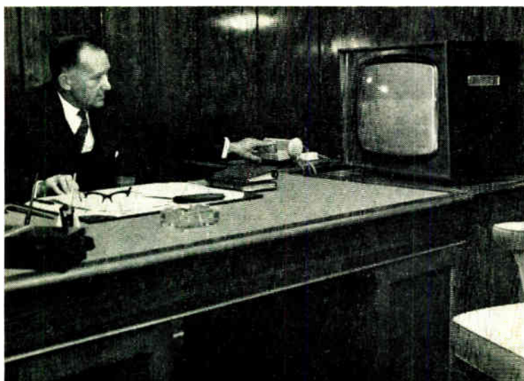
Closed-circuit television installed by Thorn Electrical Industries at a branch of the Westminster Bank. One picture shows a statement of account presented on a monitor in the manager's office, the other shows the transmitting end, also with a monitor. The statement is placed face downwards on a glass panel beneath which the camera tube is mounted
