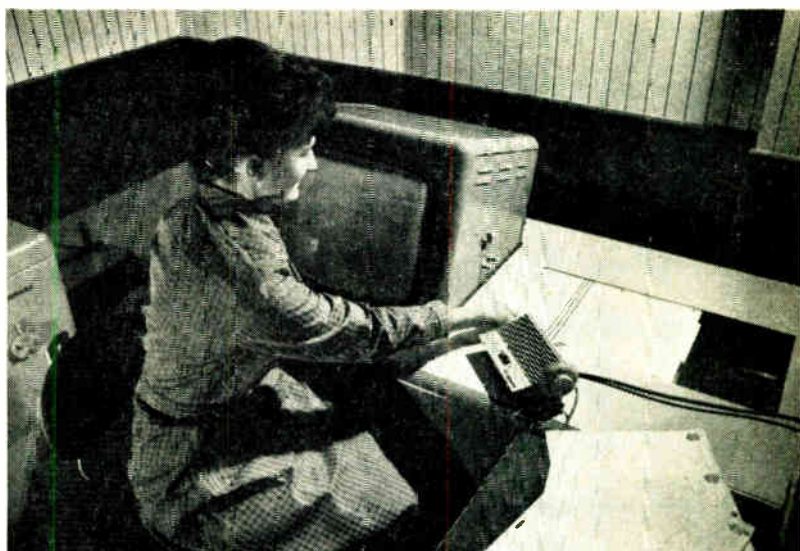
Closed-circuit television installed by Thorn Electrical Industries at a branch of the Westminster Bank. One picture shows a statement of account presented on a monitor in the manager's office, the other shows the transmitting end, also with a monitor. The statement is placed face downwards on a glass panel beneath which the camera tube is mounted
