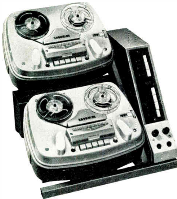
Illustrated here is the twin tape recorder unit with the control panel and shown above right is the Even Work Distribution unit
