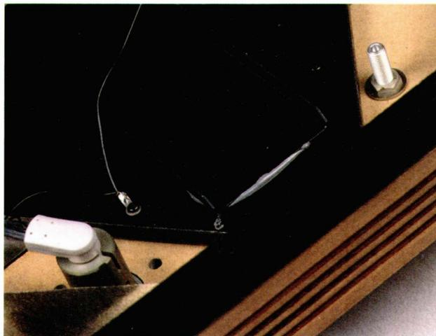
*Underside of sub-chassis showing later glued construction.*
