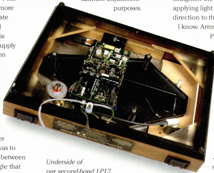
*Underside of our second-hand LP12 showing internal Valhalla power supply board and general layout.*
