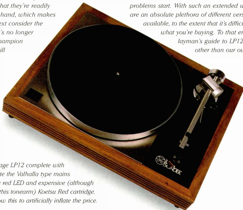
*A typical mid-vintage LP12 complete with Ittok tonearm. Note the Valhalla type mains switch with single red LED and expensive (although inappropriate for this tonearm) Koetsu Red cartridge. You shouldn't allow this to artificially inflate the price.*
