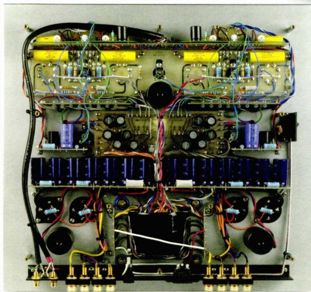
a hybrid amplifier, with a bi-polar input stage and J-fet phase splitters used to feed a hybrid J-fet/12AU7 cascode driver for each channel. The push-pull EL34s run in Class AB and the entire circuit is dual mono down to separate windings on the
