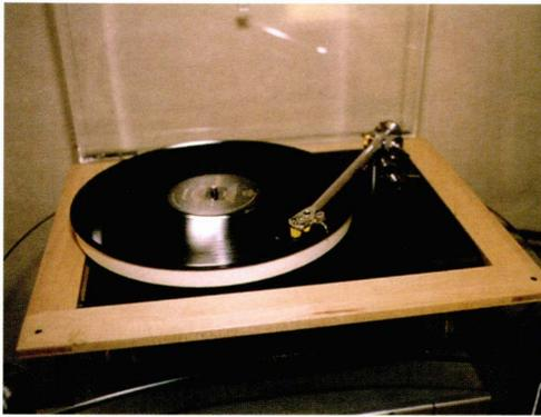
Planar 3) and no fancy carbon fibre armtube. Instead you get the same arm used on the perspective, an inverted ceramic bearing carrying an acrylic sub-platter and a substantial main platter turned from MDF but with a bonded acrylic surface and a record weight. The whole lot will set you back £500 and you get 25% off of the Ortofon cartridge of your choice! No wonder Mr Armstrong was smiling so broadly.
