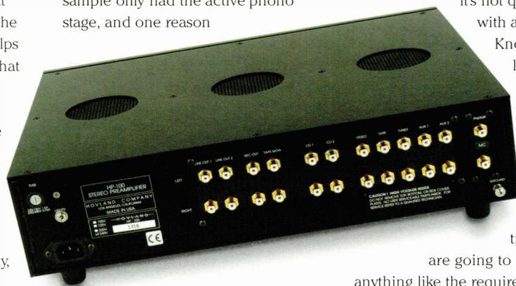
to get the pre-amp back (as well as it being the obvious partner for the Sapphire) is to listen to the higher gain phono stage. This employs a pair of custom wound transformers mounted immediately behind the phono input sockets, a neat arrangement that keeps the signal path as short as possible. Other refinements to the pre-amp
