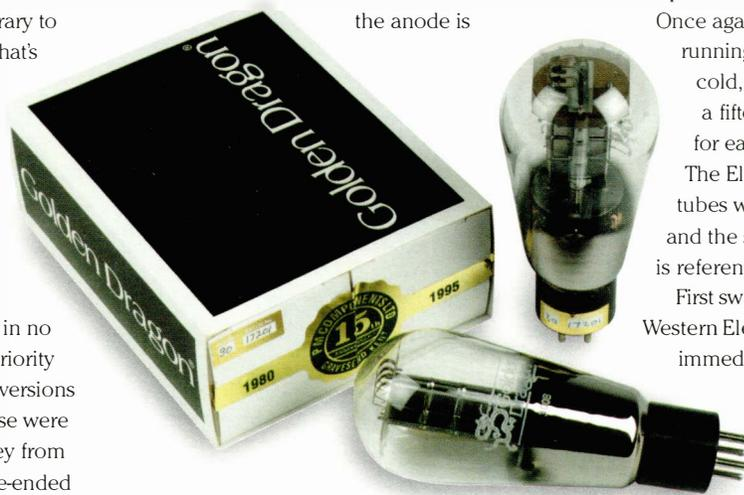
perforated with a grid of tiny holes. The theory is that the increased surface area improves efficiency, but as I'm far from qualified to discuss or pass judgement on such matters I'll confine myself to the way they sound. Just note that the M in the 300BM designation indicates this mesh anode.
