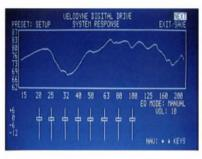
is to start fiddling with the available parameters, it is now that the hard graft begins, moving the sub (or microphone if you are doing it the other way round) to find the position(s) that yield the minimum number of peaks and troughs, i.e. the flattest overall response. Positioning is by far the most influential and critical of all the criteria in getting a good performance from the sub, and the electronic adjustments are there to tidy things up rather than radically alter behaviour.
