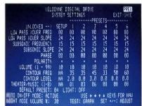
back to the sweep graph to indicate the changes made to the response. Using information gleaned form the measurements taken with just the 805's on their own, the low pass crossover was set along with the slope, the display confirming that these figures were not too wide of the mark.
