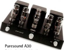
Originally dubbed (and reviewed by *Hi-Fi*+ as) the Bewitch A30, the name might have changed but the amp and its performance remain the same. This is a 32 Watt, class A, all-tube line integrated, built in China but specified by Guy Sargeant (ex-Audio Innovations). It uses a pair of 6550s a side and can be switched from ultralinear to triode output, in which guise you'll get 18 Watts per channel.
