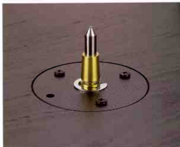
The main bearing has a brass taper to mate with and hold the platter. Tightly machined with no slack, this is a high quality item common to Chinese manufactured turntables, contributing to speed stability.
