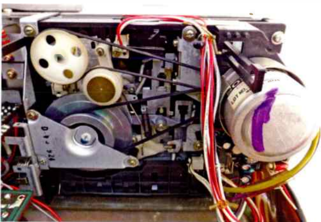
In this completely-mechanical transport, everything's driven with mechanical linkages. We can also see the belts, DC drive motor and capstan's flywheel (which must be removed to reveal the dried grease-stricken components).
