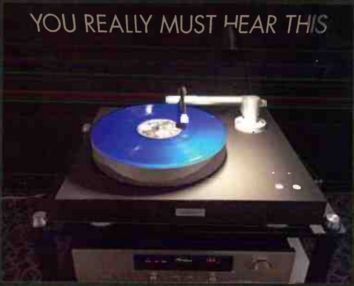
A Bergmann Magne air-bearing, parallel tracking turntable looking dramatic in the Doug Brady room. It uses an air-pump to float the arm freely on a bed of air so it can track inward unimpeded.
