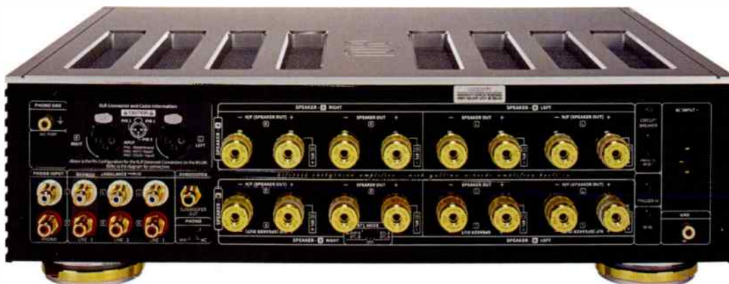
Loudspeaker sockets for bi-amped A and B channels occupy much of the rear. At left are balanced inputs (top) and line inputs (below), plus a single subwoofer output. The BTL mode switch lies beneath the speaker sockets.
