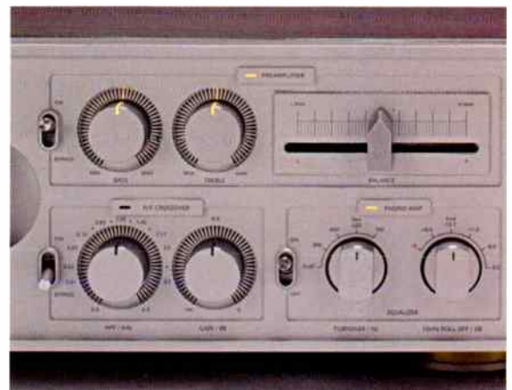
At top left, bass and treble tone controls with a Bypass switch that did not fully bypass them. Below are high-pass controls for the HF amplifier, again with Bypass switch. The Phono input (bottom right) has LF and HF adjustment to provide a wide variety of commercial equalisations from the past.
