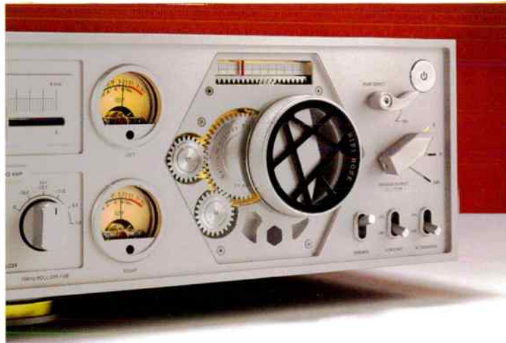
The large volume control drives a main gear that in turn spins two secondary gears (L & R). It also drives linear dial at top to show volume level. At left the meters show input level to warn of overload.
