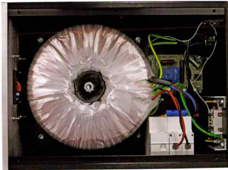
A huge toroidal transformer dominates the internal space. It feeds a large contact breaker – the white box at bottom right. The transformer sits on an isolating plate to suppress vibration and noise into the chassis.
