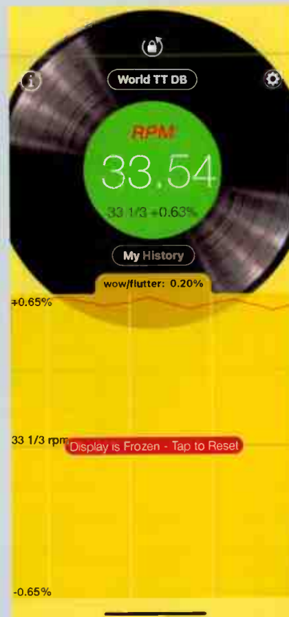
The RPM app's readout of speed as +0.63% fast, an acceptable error. Adjustment reduced this.
