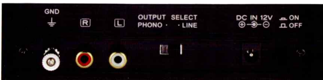
At rear a single pair of phono socket outputs switchable from Line to Phono. The Line output utilises an internal phono stage, the Phono output is direct from the cartridge, to feed an external preamplifier. Also here is a push-button power switch for the 12V power input.
