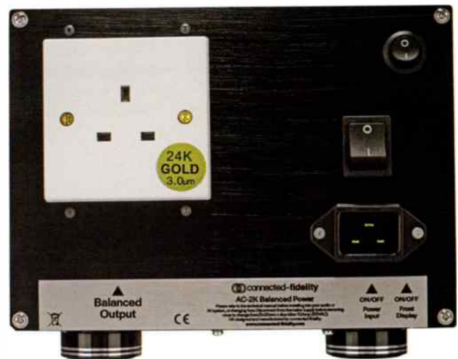
At right a large 16A input socket that demands use of a special heavy duty lead. Above it lies the main power switch and at top right a smaller switch for the front panel voltage display.
