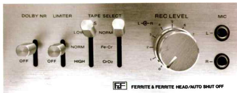
The TC-186SD isn't suitable for recording onto metal (Type IV) tapes, although it will play them with the 'EQ' switch set to the 'CrO2' position. Also visible are the Dolby and limiter switches, concentric recording level controls and rarely-used mike inputs.
