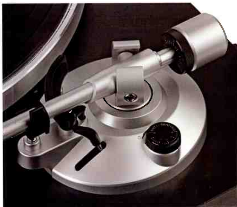
Anti-skate (outward bias) is conveniently applied by a dial on the arm base, shown here. Easier than the simple thread and weight system that's still common. The horizontal bearings are adjustable ball races.
