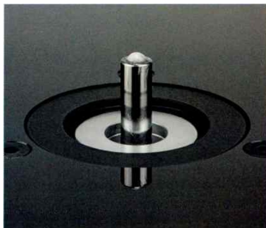
Pro-Ject's inverted bearing. The lower part is male, not female. This puts the contact area in the same plane as the stylus – not below it – minimising the effects of wobble in the bearing.
