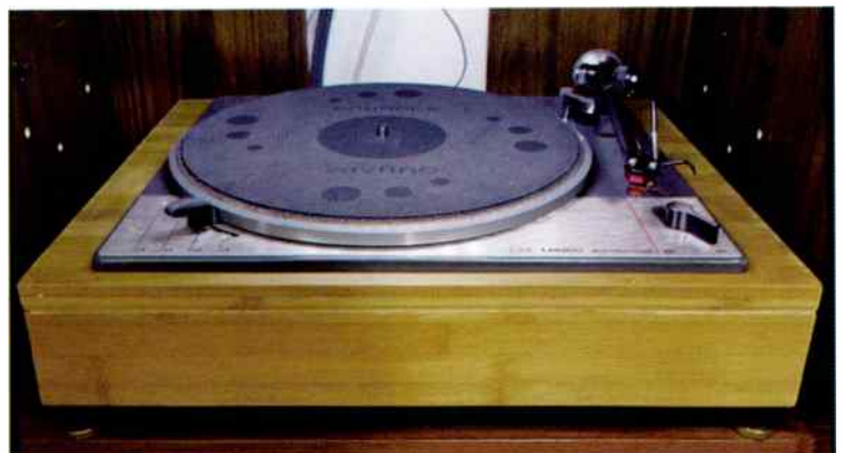
Joe Wdowiak's Lenco GL75 idler drive turntable with Rega RB300 arm, full restored. Lovely.
