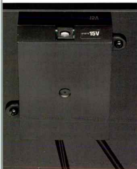
An under-side shot of the power supply showing speed adjuster screw. Get an RPM app for the 'phone to use this.
