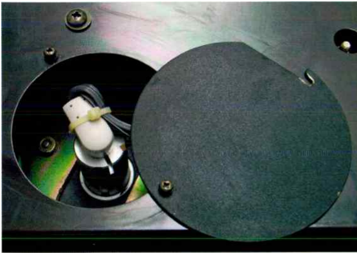
A removable base cover plate, which provides access to the tonearm base and wiring, marks out this RD80 as a later 'SL' variant. The tie-wrap secures the 5-pin output plug to the underside of the deck's Linn Basik LVV.
