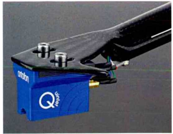
The arm's thin, flat headshell with slippery finger lift that's difficult to use. Most people will use the mechanical lift/lower, but it is undamped.
