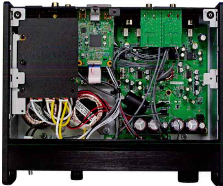
Much use of surface-mounted components is made in the UD-505-X, although audiophile-grade 'through-hole' electrolytic capacitors have been strategically-placed in the circuitry. Note too the pair of toroidal mains transformers.
