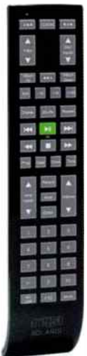
As well as the usual play and search/skip controls, the remote also gives the user access to the DAC filters and DAC input selection
