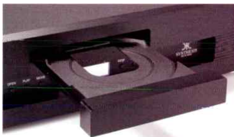
The Teac transport has a normal plastic tray, in the Synthesis fronted by a solid aluminium slab.
