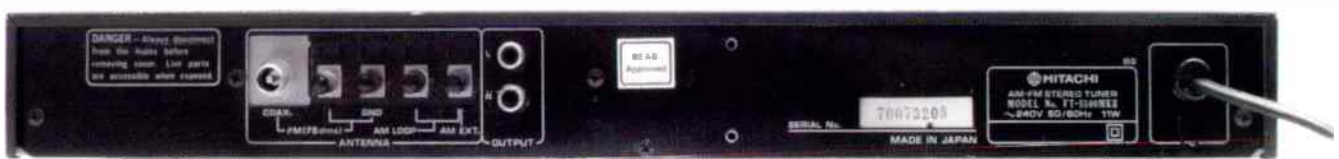
Like most digital tuners of its time, the FT5500 Mk II has VHF/FM (both 75 and 300-ohm) and AM aerial inputs, plus 'fixed level' audio outputs. Gone are the 'raw' discriminator and 'variable' outputs of earlier classics.
