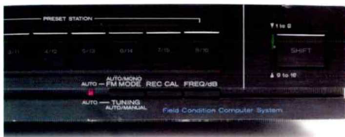
These controls give you some idea as to this tuner's flexibility. Note that sixteen favourite stations can be stored for instant access (a 'shift' button allows eight buttons to do the work of double that number!).
