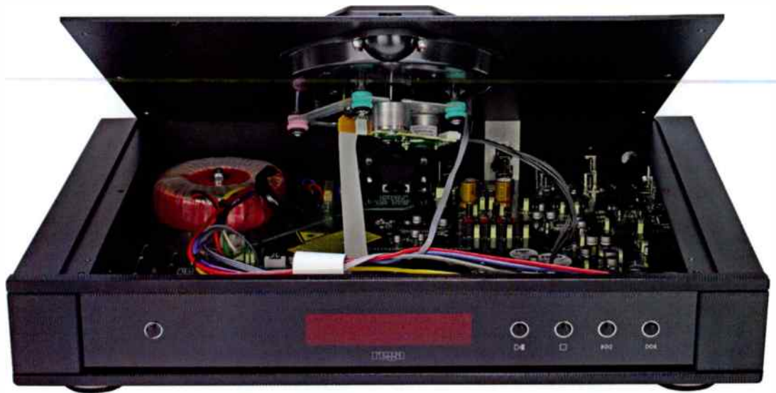
This top loader uses Wolfson WM8472 digital converter (DAC) chips and is driven by a linear power supply fed by a toroidal transformer (left rear).
