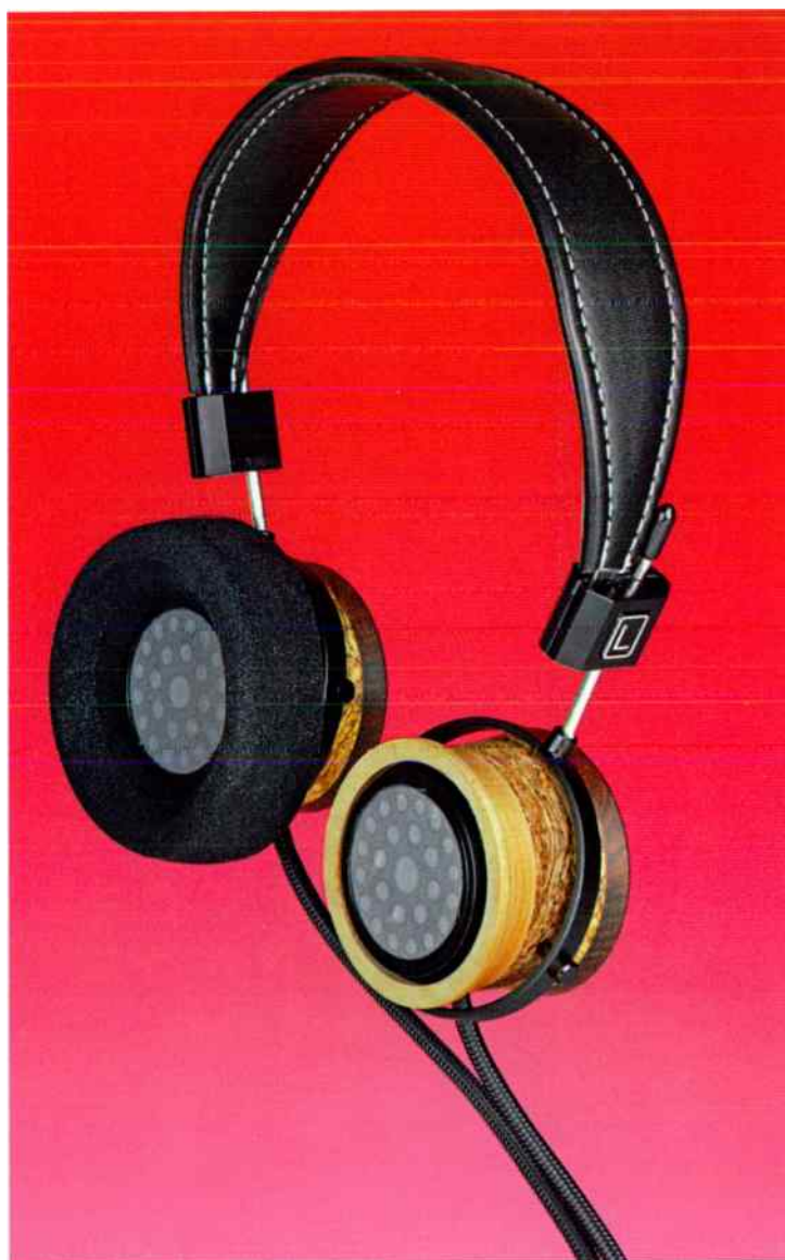
The foam ear pads can be removed for cleaning and they appear to hold the drive unit in place, which is loose in its cavity. This may make repair easy if a lead is yanked out by accident, since there was no cable clamp.
