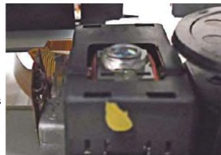
Like every other CD player, from the Sony CDP-101 to the latest models reviewed in this magazine, the DA-7000 relies on an optical pickup with semiconductor laser. This one still works; appropriately enough, a 1980s Hitachi slogan was 'in a word, reliability'!
