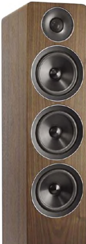
Three 130mm (5in) cone ceramic/aluminium sandwich drive units, topped by an aluminium tweeter, for consistency of material and sound. The two lower units handle bass, the third bass/midrange.
