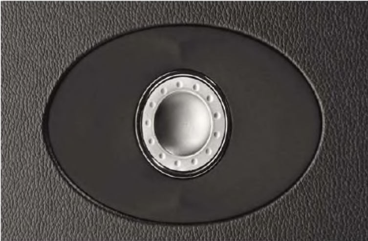
Focal's own-design 25mm inverted dome tweeter using aluminium/magnesium for light weight and stiffness. It fires into a shallow waveguide to aid dispersion and improve sensitivity.
