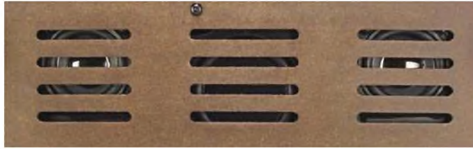
Two small loudspeakers are fixed to the underside to make the LS-55 much like an all-in-one record player from the 1960s. Even 5 Watts of power is similar.
