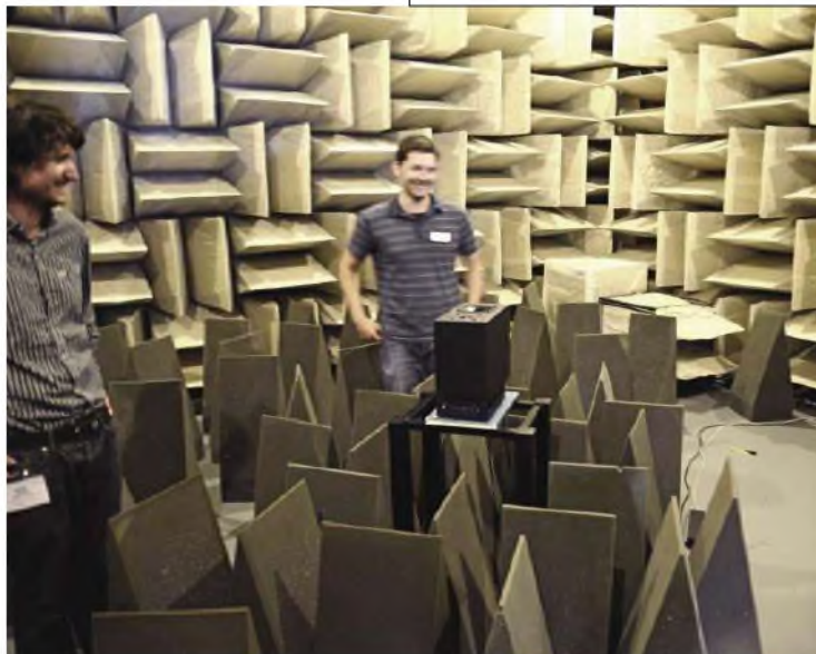
NPL's anechoic half-chamber (with hard floor). Totally silent. Over-furnish a room and it will sound similarly dead.
