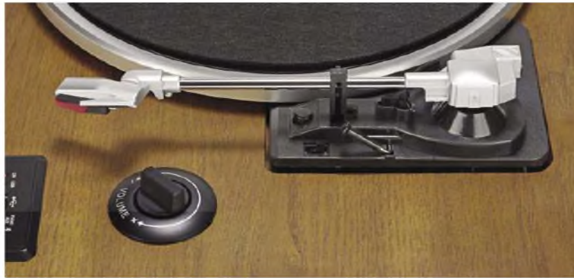
A light aluminium arm tube with flexible plastic headshell, carrying a clip-on ceramic cartridge. Tracking force nominally 5gm and not adjustable. Upgrade is not possible.
