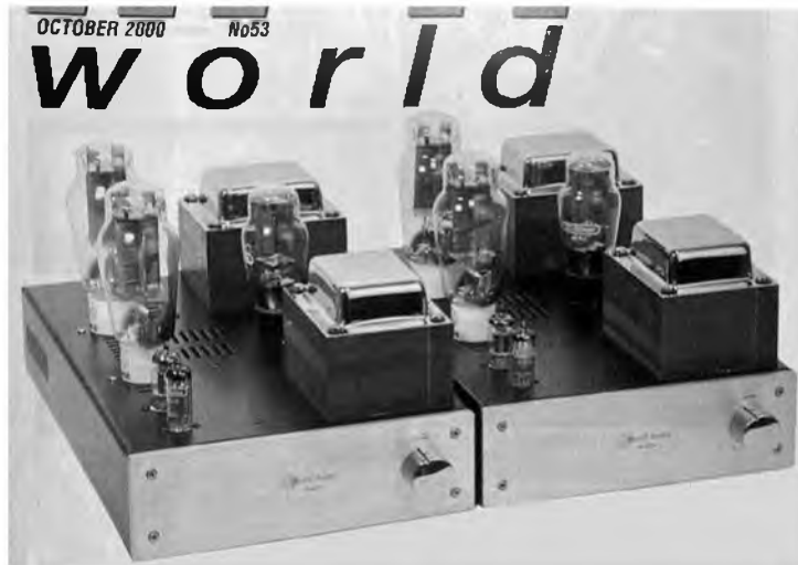
World Audio Design 300B PSE amplifier monoblocks produced 20 Watts each. Designed by Andy Grove.
