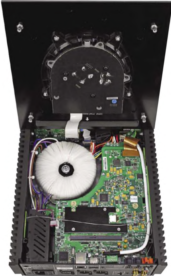
The top panel contains the specially-made volume control unit – a backlit rotary-encoder. Naim built the Atom HE’s power supply around the large toroidal transformer that dominates the main enclosure. No switch-mode supply here.
