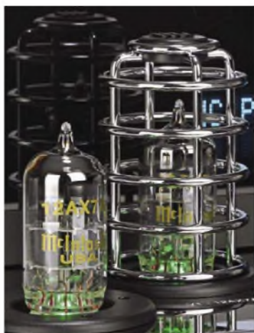
The 12AX7 double-triode preamplifier valves (tubes) provide line amplification and drive to the power amps. Note the green glow.
