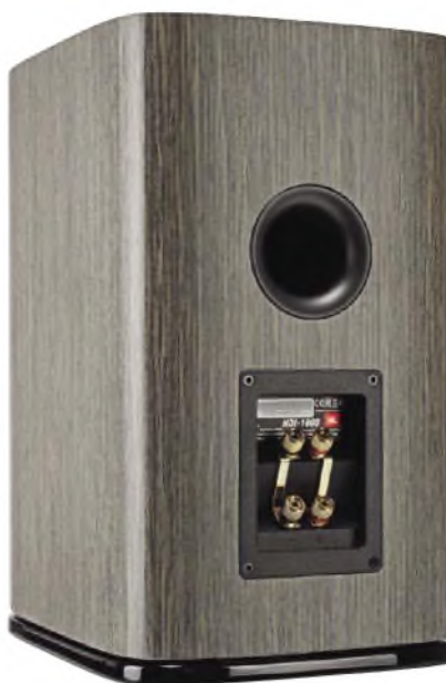
Bi-wire terminals with removable links sit on the rear panel, together with a port that reflex loads the bass unit.
