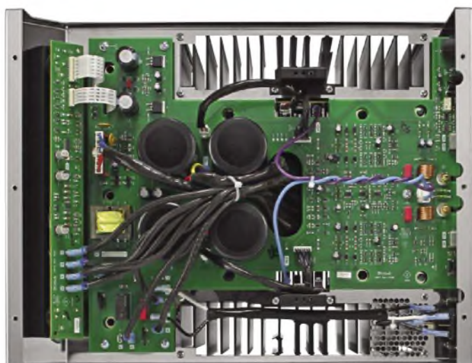
Large power supply smoothing capacitors at centre and big heat sink apertures at left and right on the MC830 chassis underside.
