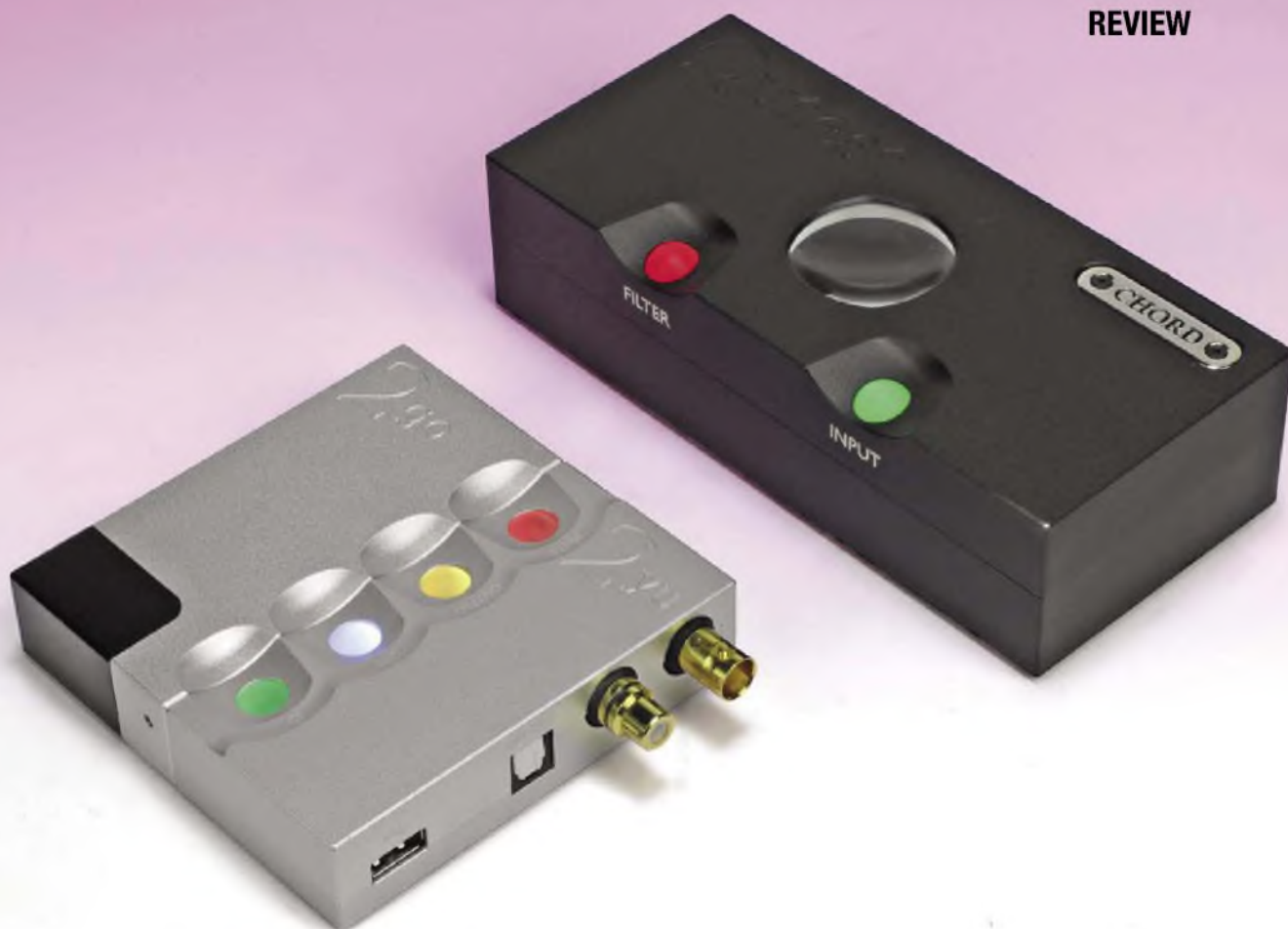
2yu has four digital outputs, to feed an external DAC or digital amplifier. At left USB, then S/PDIF through optical TOSLINK, RCA phono socket or BNC socket. We used it with Chord Electronics' Qute DAC, seen behind.
