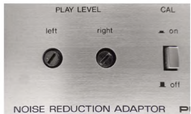
These recessed ‘play level’ trimpots form part of a calibration procedure. They’re adjusted with a flat-bladed screwdriver during playback of the recorded 1kHz test-tone, so that the N55’s fluorescent bar-graph meters register -5dB.
