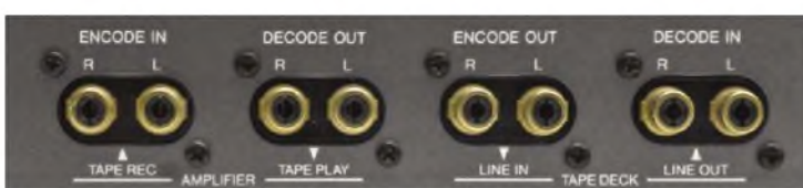
The rear-panel phono sockets allow the N55 to be easily 'inserted' between tape deck and amplifier. No balanced XLRs here...although the unit did find its way into some home studios.
