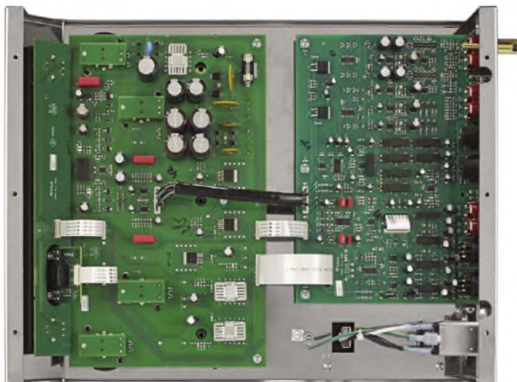
Underside of the C8. Valves sit on the front board (at left), mounted on four small daughter boards. The rear board (at right) carries relays and audio circuits. The MM and MC phono stages lie at top right, close to the gold plated earth terminal.
