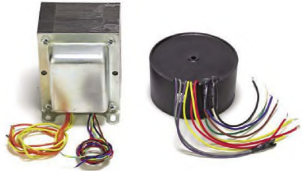
Transformers can, if imperfectly treated, hum or buzz. Note the black toroidal is potted to avoid this.
