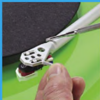
Tap arm with jeweller's screwdriver or teaspoon to see if it rings. Support lightly in finger.
