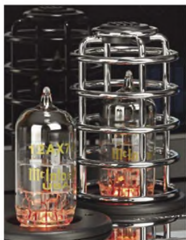
At switch on LEDs beneath the valves light up intense orange to indicate warm-up is taking place.
