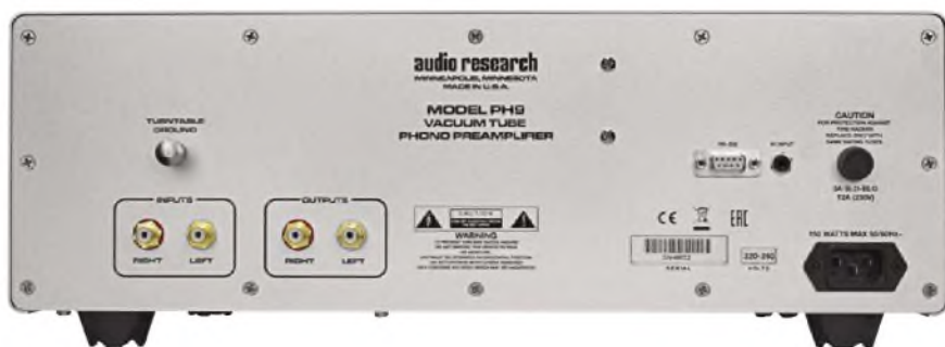
The rear panel carries just one pair of phono-socket inputs and outputs. They are internally connected to chassis earth a continuity test showed, making this an unbalanced input.
