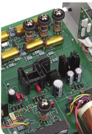
Even the 6H30P regulated power supply control tube has a damping ring around it.
