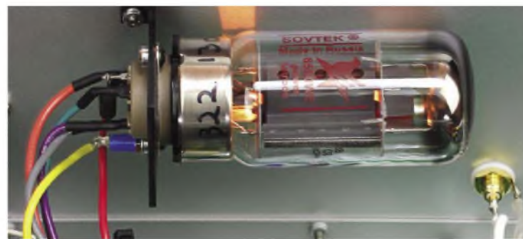
A 6550 beam tetrode that acts as a voltage regulator. Why do this? Because tubes give a deep, smooth sound when used in a power supply.
