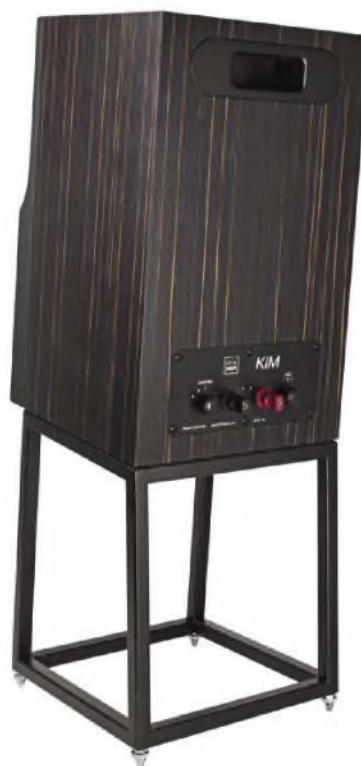
Rotary switched Bass Damping and Treble Level controls sit at either side of the mono-wire terminals at rear. At top a reflex port.
