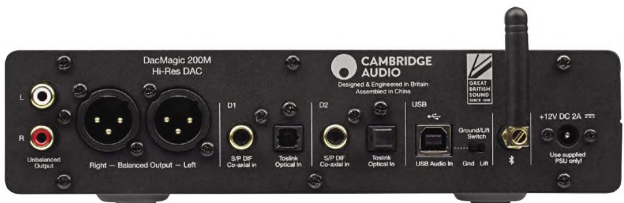
The rear carries unbalanced and balanced (XLR) analogue outputs (left). There are two sets of optical and electrical S/PDIF inputs, plus USB for computer connection and DSD. The stub aerial is for Bluetooth wireless reception from a mobile phone, tablet or portable player.
