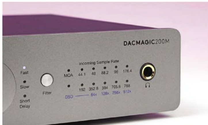
At left a Filter button sequences through Fast, Slow and Short Delay. Then MQA and DSD indicators, an array of sample-rate indicators and at right a 6.3mm headphone socket.
