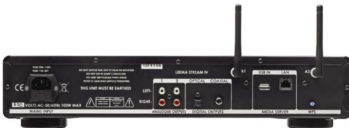
The Stream IV has an on-board linear power supply, 230V here. There are phono socket analogue outputs but no balanced XLRs. Digital S/PDIF outputs are fitted to connect to an optional external DAC, and at right lie a USB mass storage (Flash drive) socket and an RJ45 ethernet socket. There are wi-fi stub aerials too, with WPS connect button.
