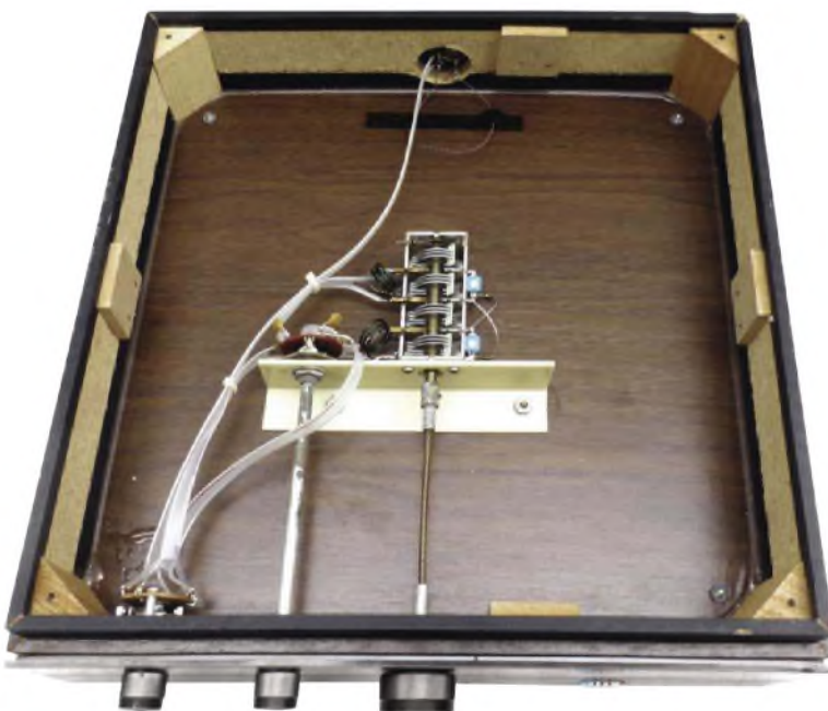
The Beam Box was made of wood, not metal, to avoid screening effects upon its short aerials. The variable capacitor and coils are spaced away from the front panel controls to avoid effects of the human body upon tuning. There is a rotary 'bandwidth' control switch, carrying the capacitors that it switches into position to modify the 'Q' of the aerial tuned circuit. Doing so sharpens its response to a narrower range of frequencies, to better reject others.
