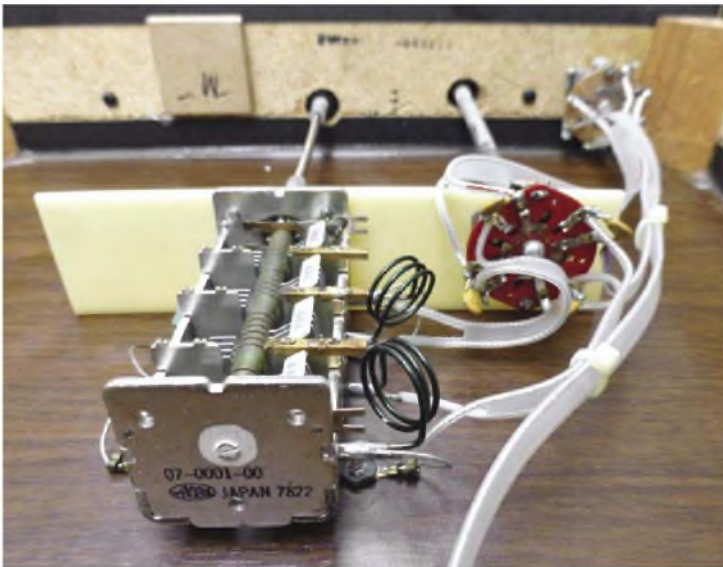
The tuning knob is coupled to this large four-gang variable capacitor, made by Japanese ALPS – the date code suggesting in 1978.
