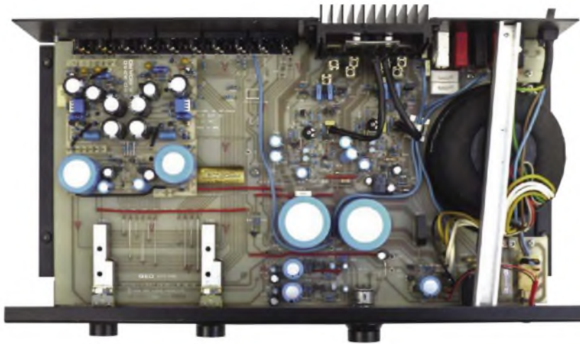
QED's "Signal Path Optimisation" in practice. The SA phono stage can be seen in the top left of the picture. To minimise hum pickup, the power supply – built around a toroidal transformer that's larger than its A240 Mk II equivalents – is located at the opposite end of the case. Between them lie the preamp stage, power supply capacitors and power amp associated with a small rear heatsink. The signal paths are completely free of ICs.
