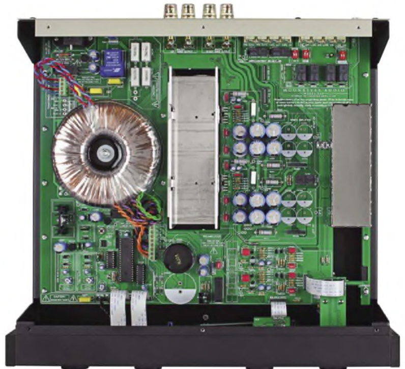
A large toroidal mains transformer at left forms the basis of a linear power supply. At centre lies a folded aluminium heatsink carrying the power transistors; with 40 Watts output cooling fins have been omitted. At right is a screening case covering the phono stage board.
