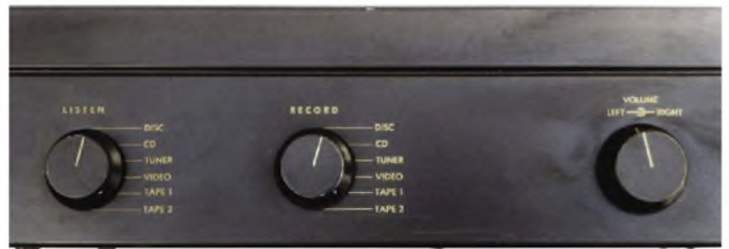
Instead of the push-buttons that QED fitted to its first amplifiers, the A270 used rotary switches to choose source input, and what is sent to your recording equipment – they did not have to be the same! The concentric volume control offers independent adjustment of the left and right channels; earlier QED amplifiers featured balance and volume knobs instead.
