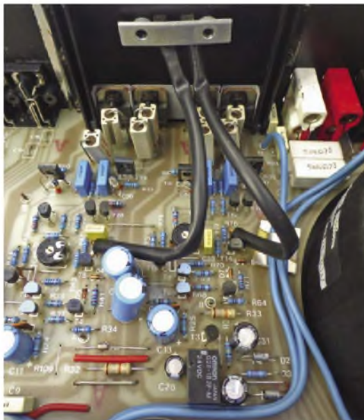
The A270's power amplifier is a fairly conventional complementary Class AB design, a split-rail power supply ensuring there's no need for unweildy (and signal-impairing) coupling capacitors on the output. Japanese power transistors are specified, and the heatsink they're fitted to is compact for a 2x50W amplifier.
