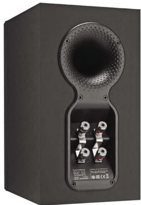
A large rear 'flowport' loads the small bass/mid-range unit to impose bass control. Beneath are bi-wire terminals able to accept 4mm banana plugs, bare wires or spades.
