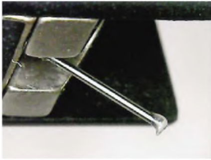
Precise attachment of the rectangular diamond shank to boron rod is seen in detail here, with bond agent carefully applied.
