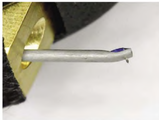
A clear shot of the aluminium cantilever shows how these items are made, having a crimped end to accept a bonded nude stylus in this case.
