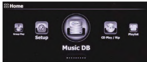
Home screen gives access to the music database of ripped and stored music, CD playback and ripping (needs external USB CD drive), playlists, the setup menu and 'group play' for multi-room systems.
