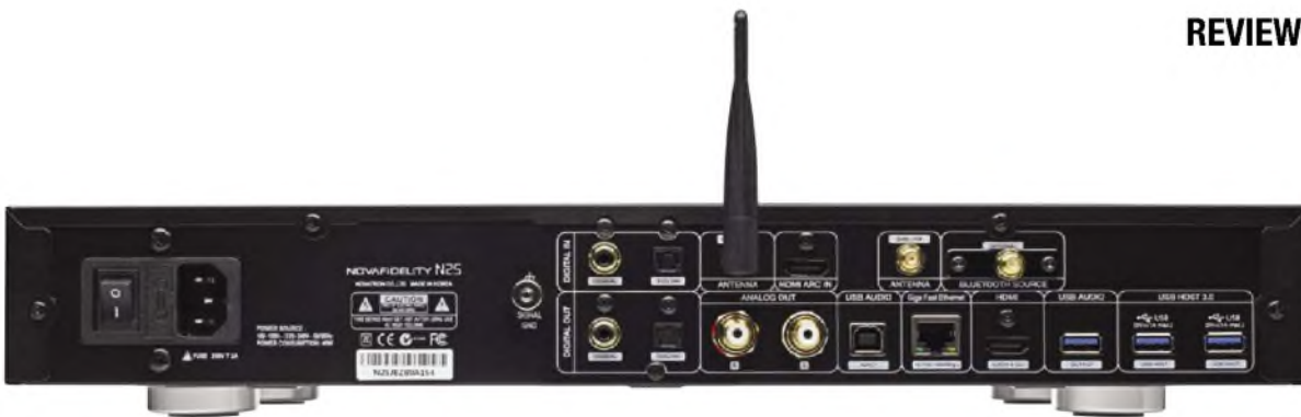
A wide array of digital inputs and outputs are provided via USB, RCA, HDMI and Toslink. Our unit was fitted with the optional Bluetooth transmitter module.
