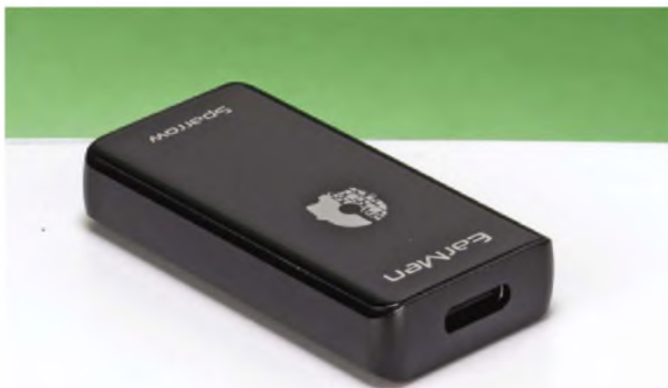
EarMen logo on front of Sparrow and Eagle glows green for normal playback and magenta when streaming MQA.
