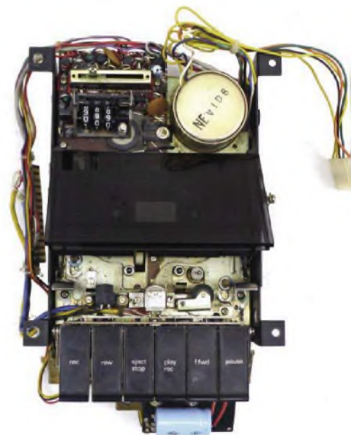
Nakamichi's well-engineered transport features a large flywheel, belt-driven from a servo-controlled motor, and the manufacturer's proprietary tape heads. Nakamichi used the same mechanism in the machines that it made as an OEM (Original Equipment Manufacturer) for the likes of Fisher, Elac, Sansui, Sonab and Concord...as well as Leak and Wharfedale.
