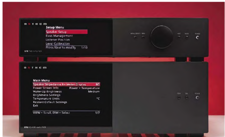
The STR Pre (top) provides a wide range of loudspeaker set-up conditions associated with room tuning, bass management of subwoofers, levels and turnover frequencies – made possible by turning all inputs to digital and processing them in a DSP.
