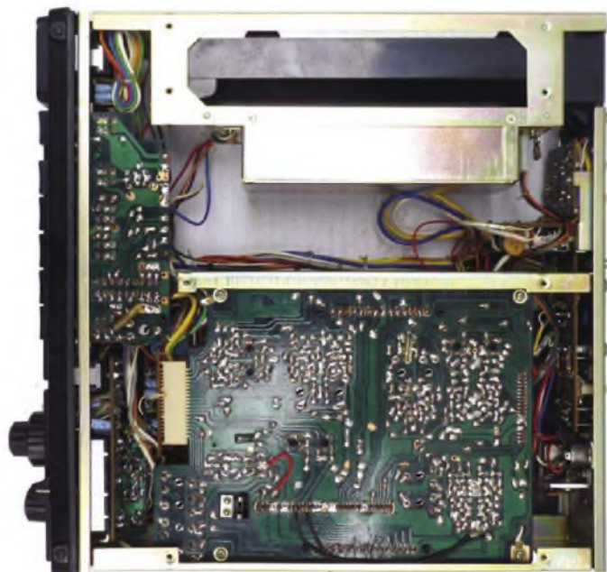
The neat internal layout of the Nakamichi 550. At top can be seen the battery compartment containing eight 'D' cells giving a total of 12V. Directly beneath is the metal box that contains the motor control and DC-DC conversion circuitry. Such screening is necessary to prevent interference from contaminating low-level audio signals.
