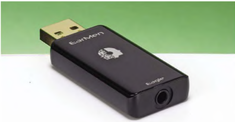
EarMen Eagle has a CNC-milled aluminium case and connects via USB.
