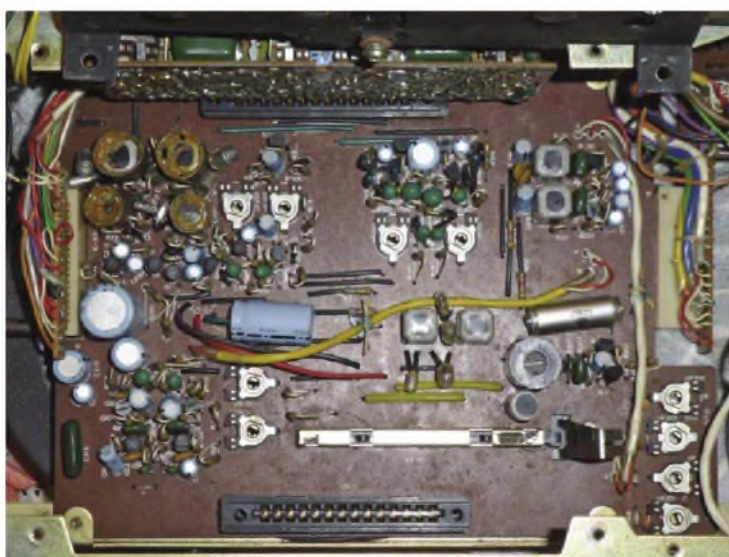
The Nakamichi 550 is built entirely around discrete components. This is a good thing, because it's easier to find substitutes for old transistors than source long-obsolete integrated circuits! This picture shows the long spring-loaded record/play switch, the 'fork' of which comes into contact with a prong on the deck, and the plug-in Dolby B board.
