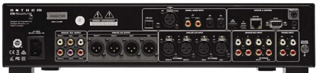
The STR Pre rear panel carries Home Theater (HT) balanced XLR inputs and outputs, which consume a lot of space. At top are the digital S/PDIF inputs plus a USB computer input (it offers no output). At right are separate MM and MC phono inputs.
