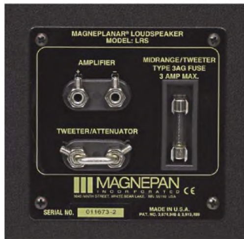
The unusual connecting panel of the LRS. It accepts 4mm plugs or bare wires of 4mm diameter, secured by a hex-key grub screw. The Tweeter/Attenuator link can be replaced by a resistor to reduce treble.
