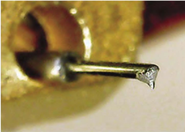
Our close up shows a stylus held by adhesive bond, inelegantly applied. The mass of the adhesive may explain high tip mass and poor tracking.
