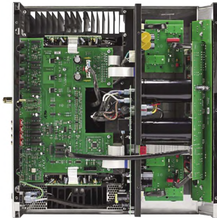
An underview, with front panel at right. McIntosh use a complex robotically manufactured board with surface mount components, including a microprocessor just below centre.
