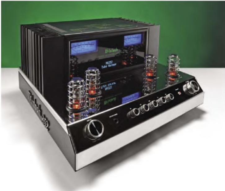
Big power meters give clear indication of output. They are electronically driven to capture peaks accurately. Centre scale is 2 Watts.
