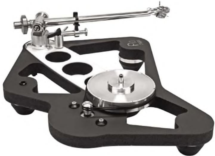
Rega's lightweight vestigial plinth has a plate coupling arm to centre spindle, to eliminate relative movement between them.
