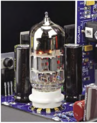
The CSA100's line amplifier uses a solitary 6922 dual-triode valve.
