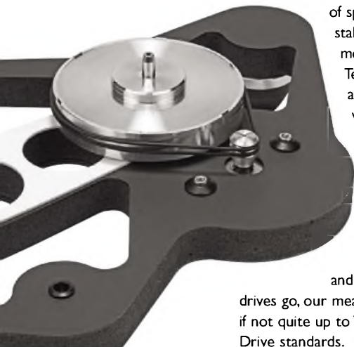
Belt drive to the hub in classic fashion, speed set by the motor power supply, not by moving belt on pulley.
