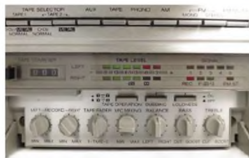
To maintain a neat appearance, some knobs and switches are covered by a drawbridge-style flap when you don’t need to use them. They include tone, recording-level, dubbing and mixing controls. None exhibited any crackling – good for a piece of equipment that’s nearly 40 years old. The LED indicators remain visible when the flap is closed.
