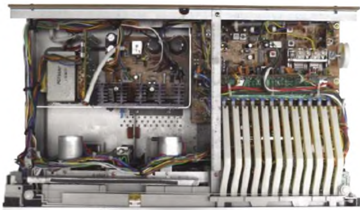
The internal layout of the SC-700 makes servicing far from easy – especially if you’re working on the cassette decks. However, a plate on the base of the unit provides access to some circuit boards. The plastic rods seen in the bottom-right of the picture couple front-panel buttons to associated switches. Not good news if you require access to the component side of the circuit board beneath!
