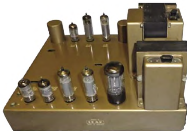
Leak Stereo 20 side view shows clearly its small EL84 power output valves (centre) and GZ34 rectifier (right). The transformers are tightly packed and the central mains transformer was known to run "warm". Power output 10 Watts – so large, sensitive loudspeakers needed.
