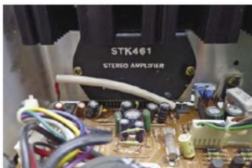
An STK461 integrated 'hybrid' module is the SC-700's power amplifier. It's claimed to deliver 25 watts or so per channel into 4 ohms. If one or both channels are dead you may have to replace the entire integrated module. Thankfully, at £10 a shot STK461s are not expensive.
