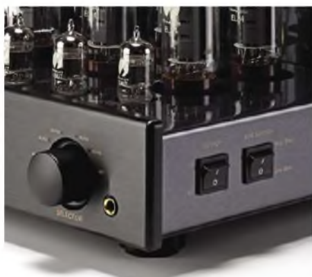
At right lie rocker switches to change bias and switch off output for headphone listening.
