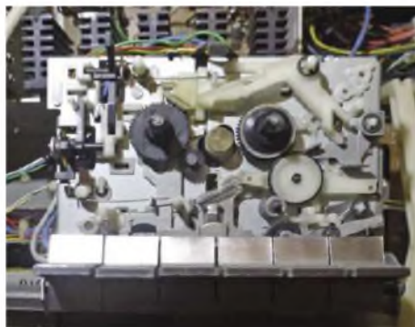
Here's the SC-700's simple but effective record/play transport. You can see the idler that couples the take-up spool carrier to the capstan shaft, via a cutaway in its housing.
