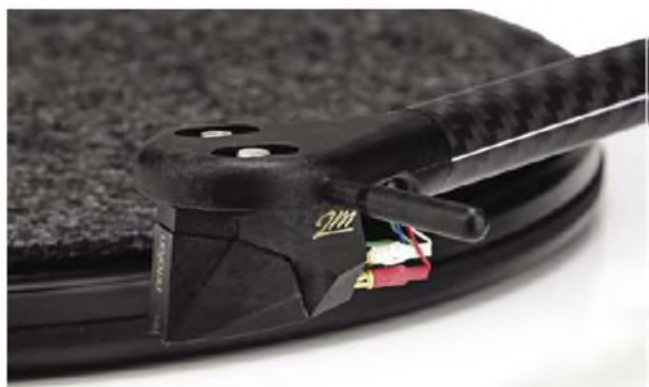
The arm with an Ortofon 2M Black MM cartridge we fitted. Not a price match, but gave a fine sound. Looks good too.
