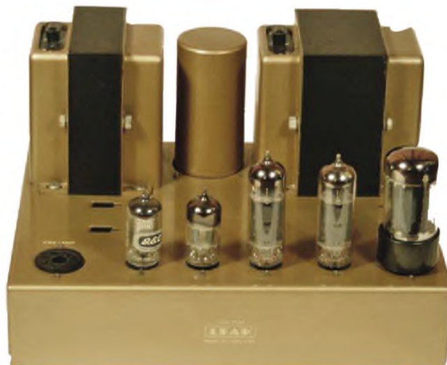
Leak TL/12 Plus – an update of the TL/12 – released 1956. It used smaller EL84 output valves in place of KT66s.
