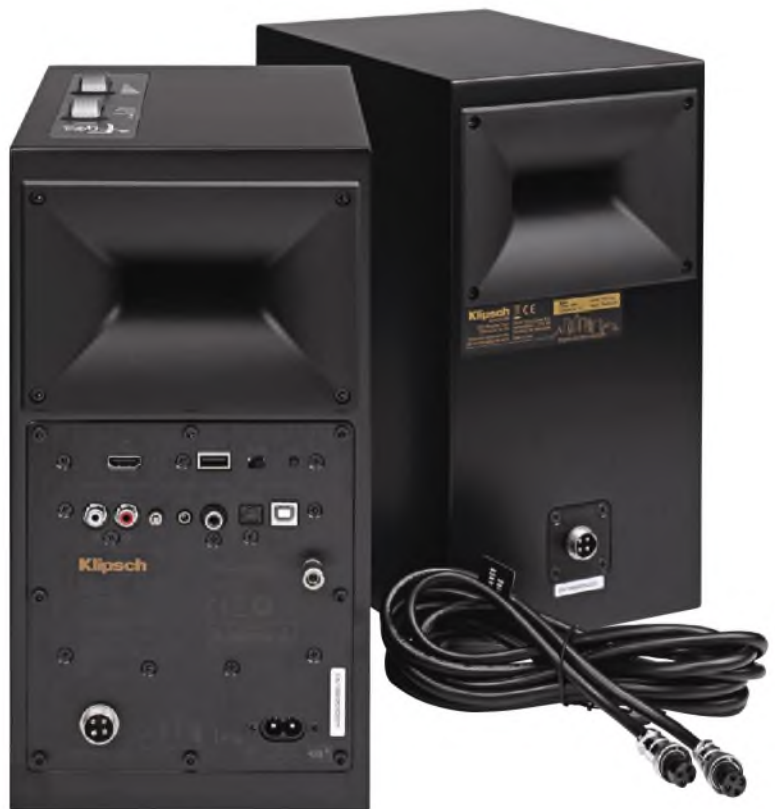
The right loudspeaker (at left in this picture) carries a small 110V-240V mains input, a four pin connector for the right passive speaker, plus an array of digital and analogue inputs. The RCA phono sockets are switched between Line and Phono for a turntable. There is a sub-woofer output too.
