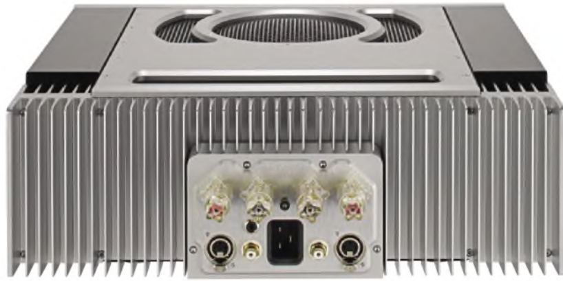
Massive heatsinks adorn the amplifier's rear, but it runs cool in normal use. One pair of loudspeakers only, and a large/unusual IEC mains socket sits between the analogue inputs.
