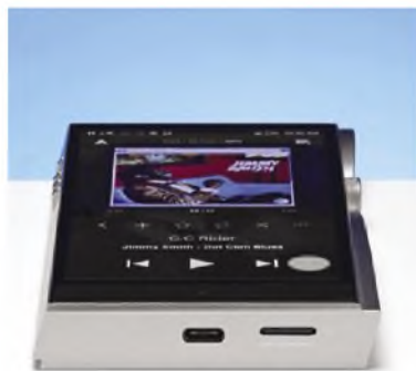
The underside has a USB C style socket for charging/file loading and (right) a single microSD card slot.
