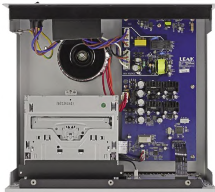
Under the hood of the CDT CD disc player. At left the slot-loading CD transport mechanism. Near top is the circular toroidal transformer of a linear power supply. The historic Leak logo (right) now adorns a modern electronic circuit board.
