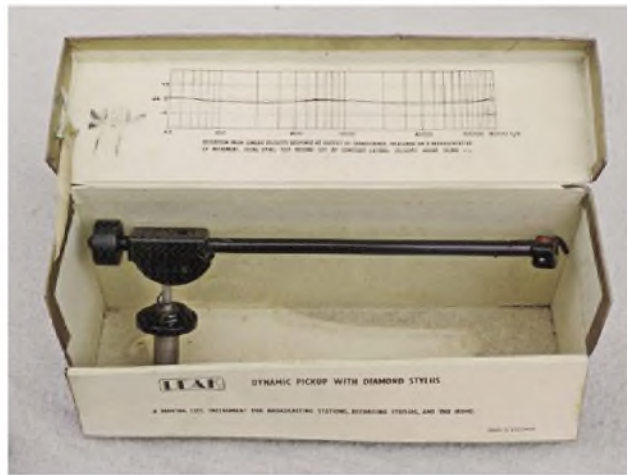
Leak 'Dynamic pickup' arm with moving coil cartridge for microgroove LP, introduced June 1954.
