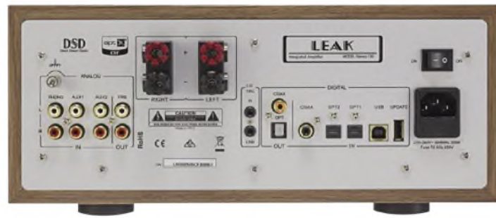
Comprehensive connectivity including Pre-Out to feed an external power amplifier. Plenty of digital inputs; no XLR balanced inputs. Note the DSD logo at top left: DSD can be played from a computer via USB connection.
