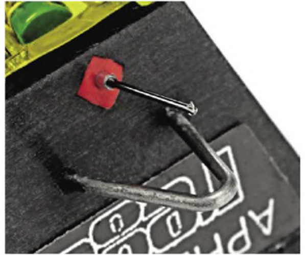
The boron rod cantilever carries a line contact stylus. Above is a guard. From above it can be seen clearly when cueing.
