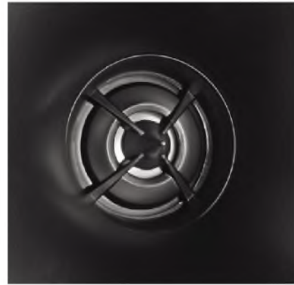
A 1 inch (25mm) titanium dome tweeter with phase cap and Tractrix horn loading that gives it wide dispersion and optimal acoustic coupling.
