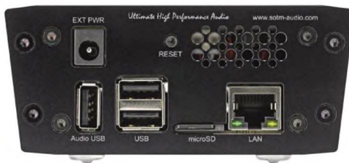
Rear panel is minimalist. A microSD card in a slot (centre, bottom) contains the operating system. Two USBs connect to external disc 'mass storage', whilst a third (bottom left) connects to a DAC.
