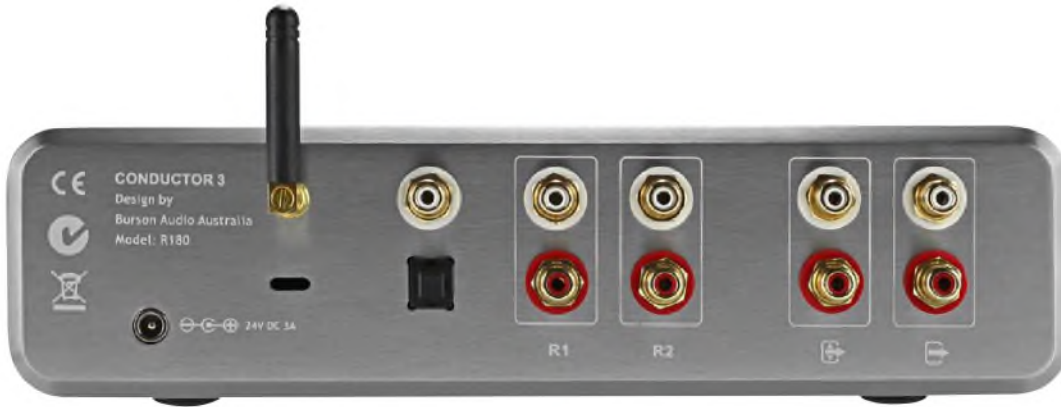
Rear panel carries a Bluetooth aerial and an array of solid, gold plated phono sockets, but lacks a balanced output.
