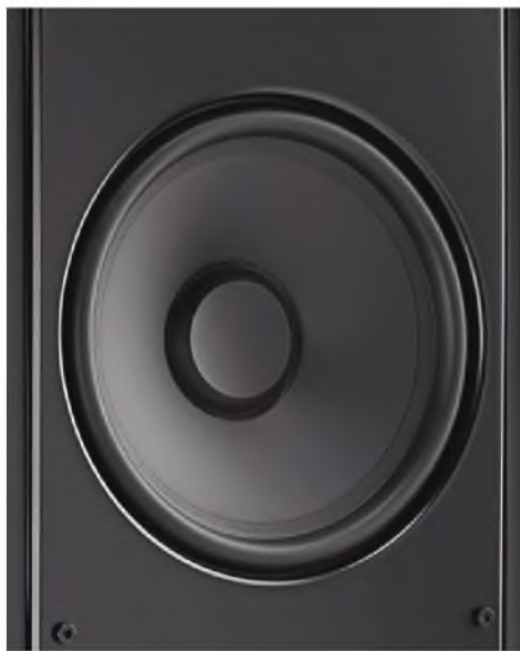
The 40i uses aluminium cone bass drive units with a central 'parasitic cone' – in this case a concave cap. It radiates high frequencies. The upper driver has a fixed pole piece cap. of the same shape.
