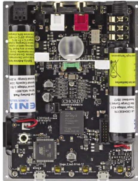
Li-ion rechargeable battery packs at left and right, the volume control sphere at top, and Chord's own DAC on an Artix FPGA.
