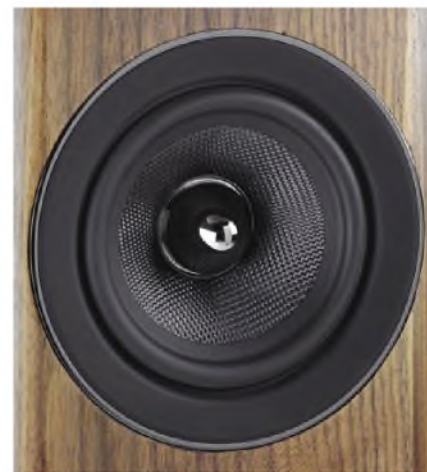
The Kevlar cone bass unit reaches up to 1.3kHz, covering a lot of the audio band. The silver parasitic dome delivers highs.
