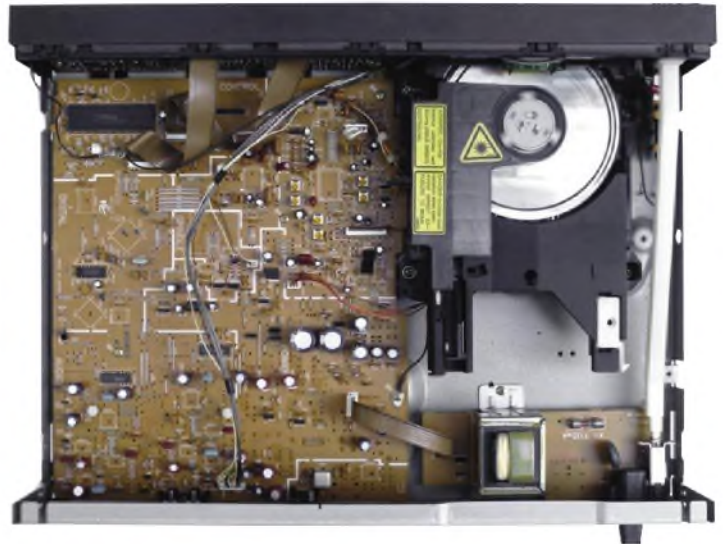
A lot going on here, and so it’s not surprising that the SL-P550 sold for £300 – worth nearly a grand today. Lots of components on the circuit board, some of which are surface-mounted chips on the flipside (their outlines have been silk-screened onto the board).
