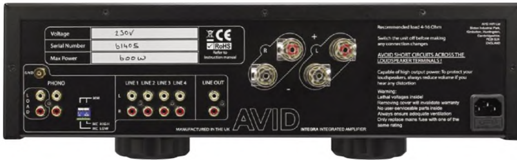
At left on the rear panel the Phono stage input for turntables. Then (going right) four Line inputs and a Line out. At centre, Left and Right loudspeaker output sockets.
