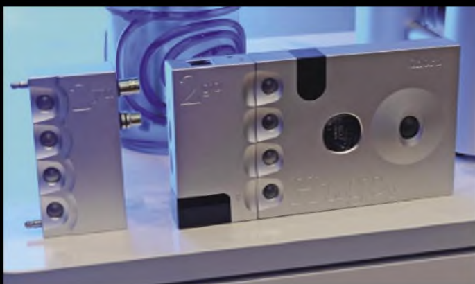
Chord Electronics 2go (£995) links Hugo2 with internet streaming music services and can play music from microSD card, whilst 2yu (£449) is a plug-in digital interface for 2go that provides S/PDIF and USB digital outputs for alternative DACs.
