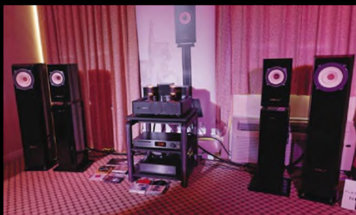
One of the few valve amplifiers at the show, the Voxative T-211 single-ended design uses one 211 valve per channel. Not much power available here, 12 Watts per channel being quoted, but Voxative have suitably sensitive loudspeakers using their own full-range drive unit. Lively sound with confident clarity.
