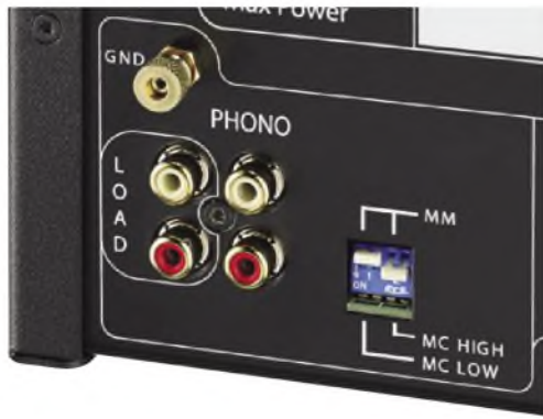
The Phono input for turntables. A single pair of RCA sockets, plus small slide switches to set gain for MM, or MC high / low. The LOAD sockets at left take MC loading resistors.
