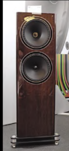
The massive – and impressive – F704 loud-speaker from Fyne Audio, with co-axial drive unit at top and bass unit below, said to deliver a shattering 96dB from 1 Watt. Price £10,999.
