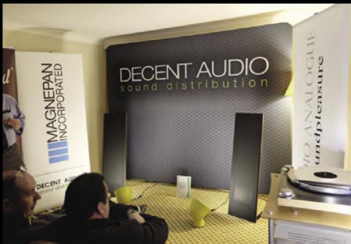
...and the other panel loudspeaker at the show was Magneplanar's new LRS (little ribbon loudspeaker). Unlike Martin Logan's electrostatics the LRS uses a conductive ribbon to drive a flat panel 48in (1.2m) high. It sounded as smooth as Maggies usually do. Imported by Decent Audio, price a very reasonable £999.50 – see review in this issue.
