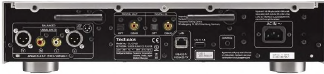
At rear left are gold plated phono socket (unbalanced) analogue audio outputs, straddling them large XLR (balanced) analogue outputs. At centre is a RJ45 ethernet socket for network connection plus a USB socket for an external hard-drive (HDD) for music storage.
