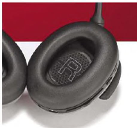
The detachable pads, made of foam covered by a synthetic leather material, are soft and provide a comfortable ear seal.
