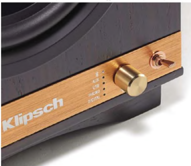
The front right loudspeaker provides access to all the various inputs: Bluetooth reception, Aux, Phono, USB and Digital.
