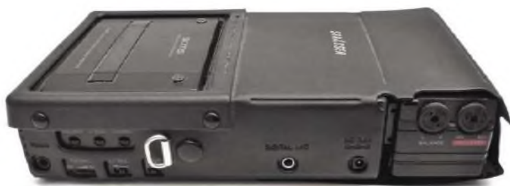
The HD-S1 ready for action in its carrying case, with the HD-A1 module fitted. The digital I/O visible on the side is a stereo 3.5mm jack socket – to get standard S/PDIF signals into and out of the unit.
