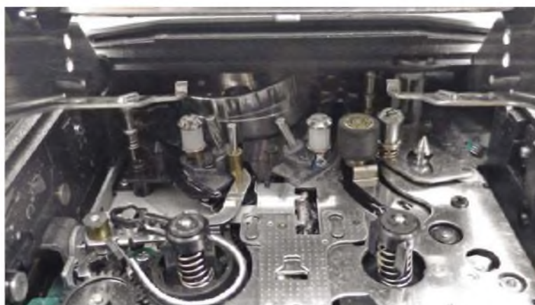
Like a camcorder guides lace up the tape around the head drum (visible at the back of the photo). The miniature pinch-roller, spool carriers and felt-covered back-tension band may have been lifted from a 8mm camcorder made by Aiwa's owner Sony.
