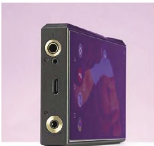
The bottom face has a sturdy 4.4mm balanced output (top), and beside it a tiny 2.5mm balanced output. At bottom a 3.5mm headphone socket also acts as a Line output (fixed volume) and a digital S/PDIF output using a supplied adaptor.
