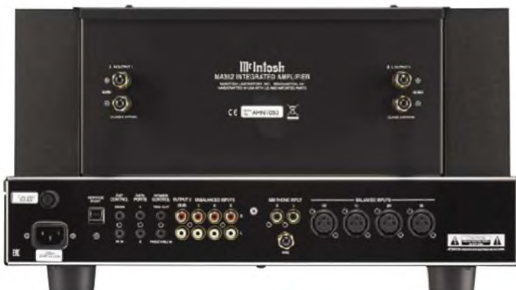
Loudspeaker terminals sit high up, just behind the power amplifier boards. Below are Line inputs, a Phono stage with earth terminal (centre) and balanced XLR inputs at right.
