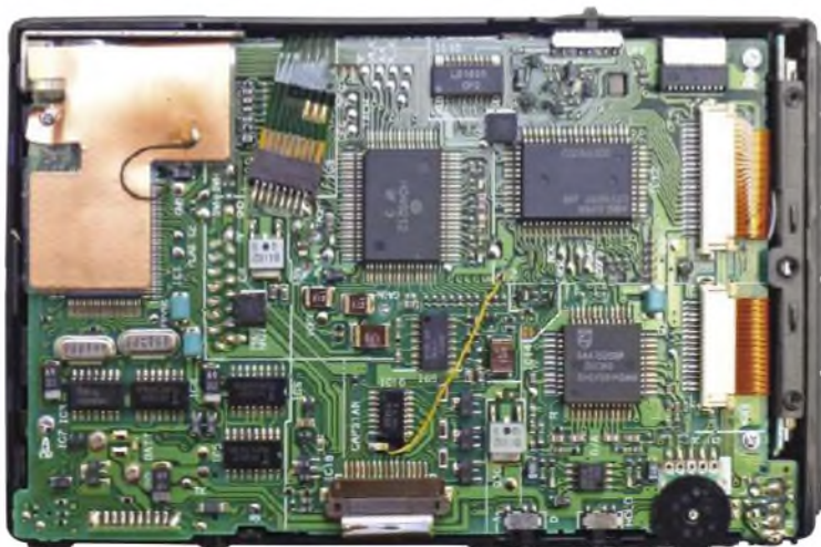
The main circuit board contains miniature surface-mounted components to keep down size and weight. One of the chips (visible towards the right of the picture) is the HD-S1's Philips SAA7320GP Bitstream DAC.
