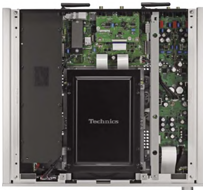
The disc drive sits in a rigid vibration free housing for maximum laser read accuracy – seen at centre. At left is an extensive screened power supply section, at rear the Bluetooth and wi-fi and at right the digital and analogue audio sections.
