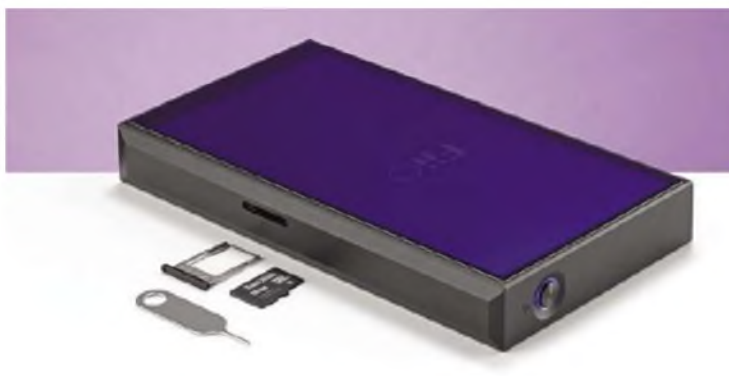
The single card slot uses a card carrier, rather than a push-n-click open slot. It's secure and dust proof, but needs a small tool seen here (supplied) to activate. A paper clip will do.
