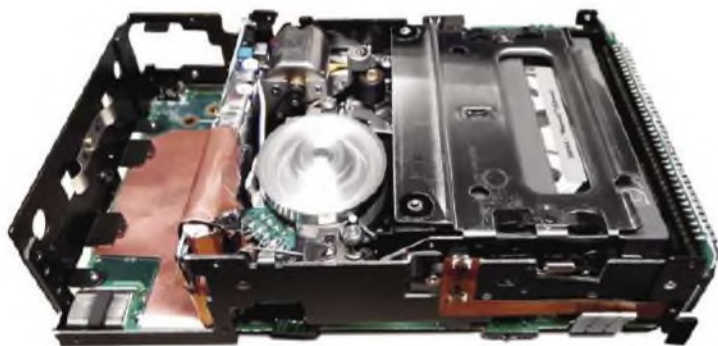
The naked HD-S1, playing a tape. Looks like the business end of a vintage camcorder – because DAT machines and camcorders shared precision-engineered mechanics and principles – a rotating drum with two helical-scanning heads. The empty space at rear is a compartment for the rechargeable battery pack.
