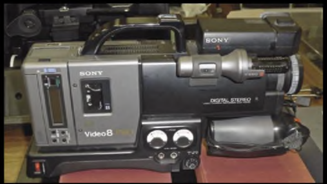
What makes this Sony CCD-V200 low-band 8mm camcorder, circa 1989, so special is that it was the first domestic cam to feature a stereo digital soundtrack. Admittedly primitive by today's standards – 10-bit, companded to 8-bit, with a sampling rate of 32kHz. The CCD-V200 included a decent stereo microphone and manual recording level with metering. This one came as part of a complete 'kit', complete with case, for £40 - a fraction of the original retail price. It needed work, though.
