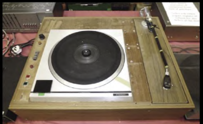
The Technics SP10 direct-drive turntable. According to the seller, a BBC employee acquired it on retirement for the basis of a digital transcription operation. The selection and arrangement of controls reflect its professional heritage. The extra-long tonearm, a homebrew effort, was included for a very reasonable £300.
