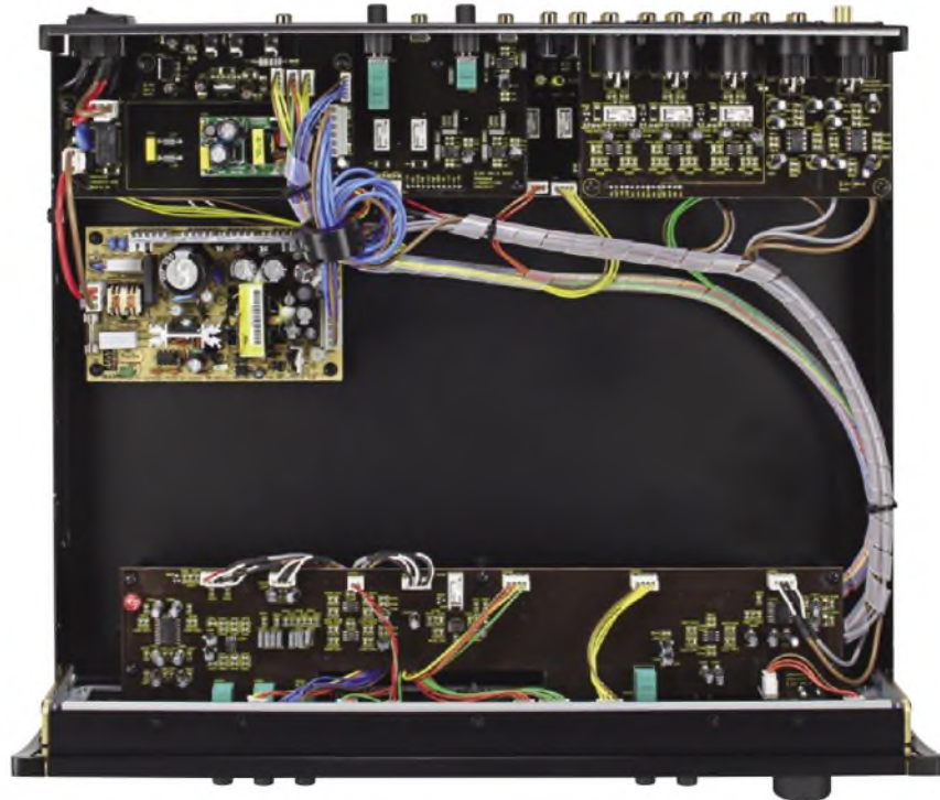
The interior of the P6 is not as busy as that of the A23+, but the layouts are similarly-neat. Note the use of miniature relays to switch between input signals, and a computer-type switched-mode power supply. This isn't in a screened compartment, but noise wasn't a problem.
