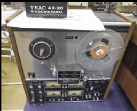
A Teac A-2340 open-reel with 7in reels and choice of speeds – 9.5 and 19cm/s. This one came with a 'mix-down' panel and manuals, but it needed work. The tape counter was damaged, and the record and playback heads had seen better days. According to the seller, there were electronics issues too. With this in mind, the £100 being demanded seemed fair.
