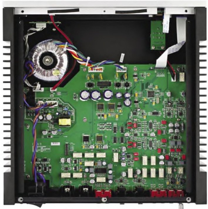
At top left, just behind the front panel, is a circular toroidal mains transformer of the linear power supply. Banks of small white, sealed long life relays switch the analogue signals. At bottom is the rear panel with inputs.
