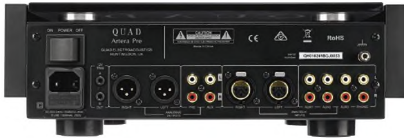
The rear panel carries a mains isolating switch, but switch on/off is by remote control, made possible by a secondary standby power supply. Big XLR input and output sockets (balanced) supplement conventional RCA phono socket inputs and outputs (unbalanced).
