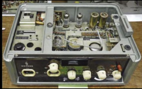
A mono "Sf V 6.6" amplifier, which employs two EL95s in push-pull to deliver five Watts, made by German firm Siemens in the mid-1960s. This was one of a pair requiring attention. £200 was somewhat optimistic, considering that the Sf V 6.6 was actually designed to sit underneath a Siemens 2000 projector – thereby explaining the lack of a top cover.
