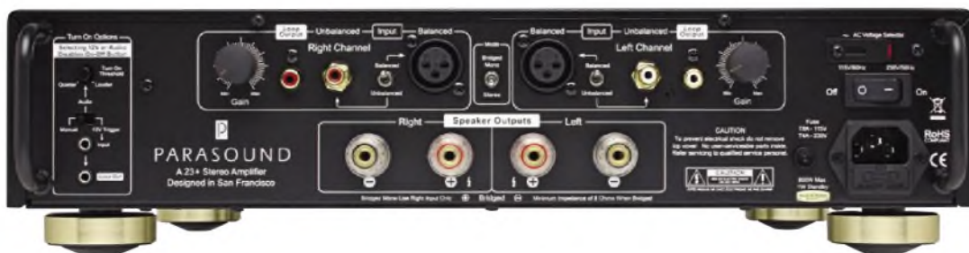
The A23+ power amplifier has balanced (XLR) and unbalanced (phono) inputs, and there are loopthrough outputs too. Input levels can be tweaked and it can be bridged into a super-powerful mono amp. A 12V trigger allows the A23+ to be switched in and out of standby by the P6. There's also a feature that will awake the A23+ as soon as audio is applied.
