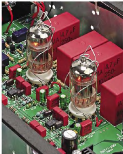
Two ECC82 output valves working in balanced mode swing 5V out via XLR.
