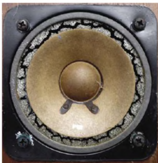
Most of the drive units have a fabric surround, which seems to be durable. The tweeters are alas an exception - the foam they use eventually disintegrates (as with other drive units using surrounds fashioned from this material). Eventually, they will end up looking like the pair you see here. These tweeters have a 16 Ohm impedance and replacements are difficult to come by. It's just as well that 're-foaming' kits are available online.
