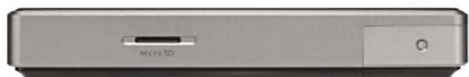
The microSD card slot can address up to 2TB, so there's plenty of storage capacity – needed for DSD.
