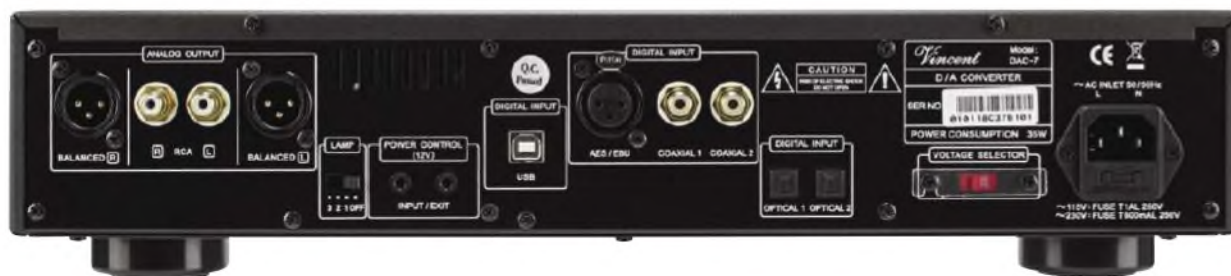
At left lies the analogue outputs, both RCA phono socket (unbalanced) and XLR (balanced). Near centre are the USB B socket for computer connection, plus an AES/EBU balanced digital input, two electrical S/PDIF inputs via gold plated sockets, and then two optical inputs.
