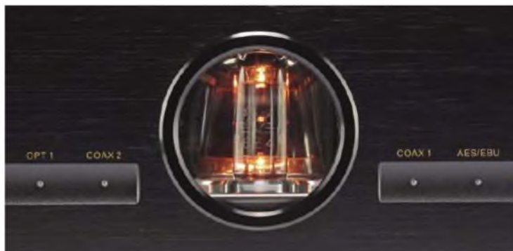
The bright glow comes from the 6Z4 rectifier valve, not from LEDs! There's a warm up time of many seconds.
