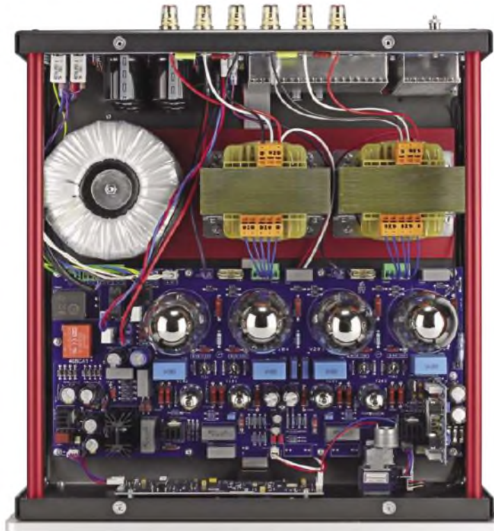
The Copland is built on a neatly arranged modern circuit board (blue). At top left is a large toroidal mains transformer and to its right Copland's large output transformers. Four KT150 power output valves are below. At bottom right is an Alps Blue motorised – for remote control – volume control.
