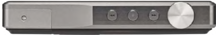
The large volume control at right has high resolution. To its left sit track skip and pause/play buttons.
