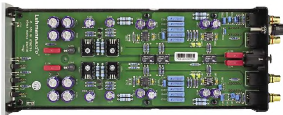
A neat internal circuit board with full size components (no Surface Mount Devices) and basic 8-pin silicon chips, plus small-signal relays (centre). Conventional but neatly laid out and symmetrical.
