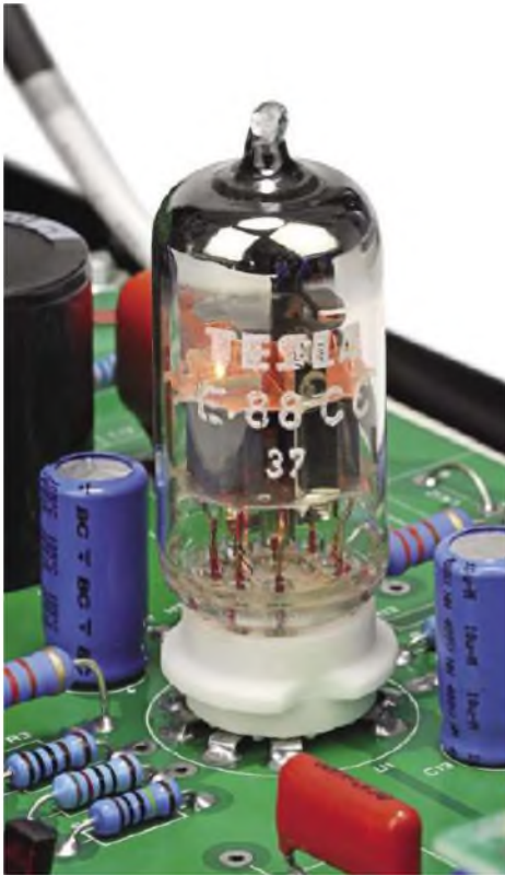
The single Tesla E88CC double-triode valve sits in conventional PCB base. Those wanting a bit more glitz can order a base with gold plated pins, at extra cost.
