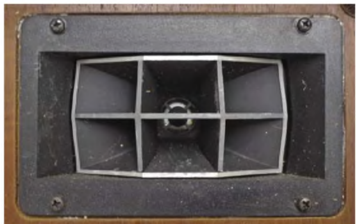
With its multicellular horn, this looks a bit like something you'd find in a concert FA system - only on a miniature scale. It is however the CS-88A supersonic tweeter ('supertweeter'), which cuts in at 14kHz or so.
