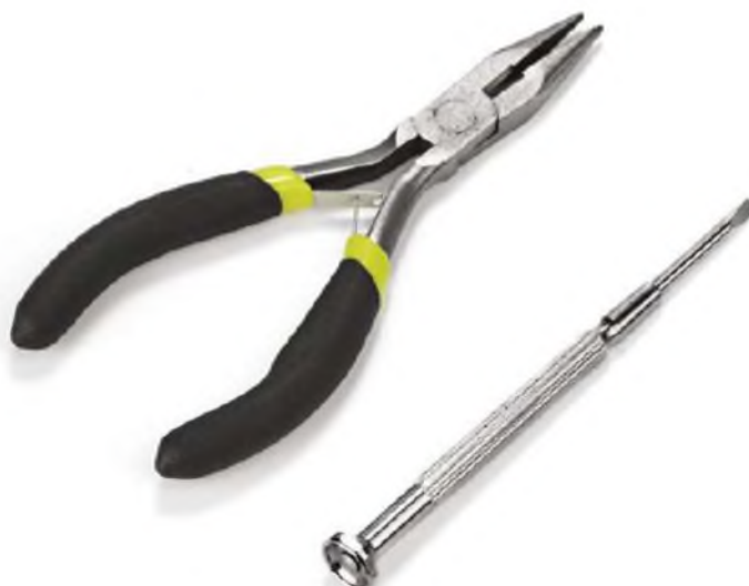
Tools needed are a pair of fine long-nose pliers and a small jewellers' screwdriver.
