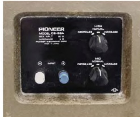
Here are the 'push-fit' speaker terminals and the rotary three-position switches that allow the midrange and treble response to be tailored. Full response is achieved in the 'increase' position; in the normal and decrease positions, the midrange and treble are respectively -1.5dB/-3dB and -2dB/-4dB.
