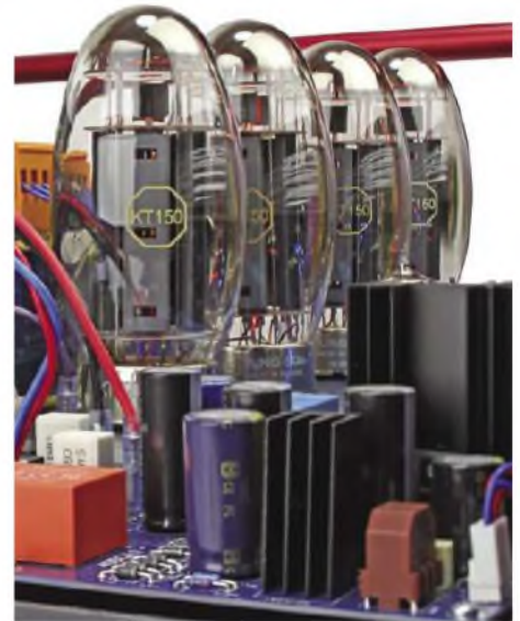
The KT150 valves in situ.
