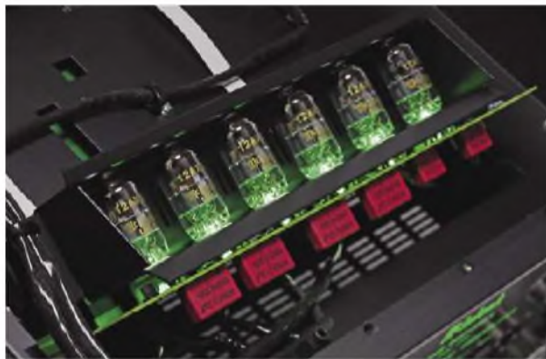
Beneath the C70's top panel lie six 12AX7 preamplifier valves, visible beneath a clear window.
