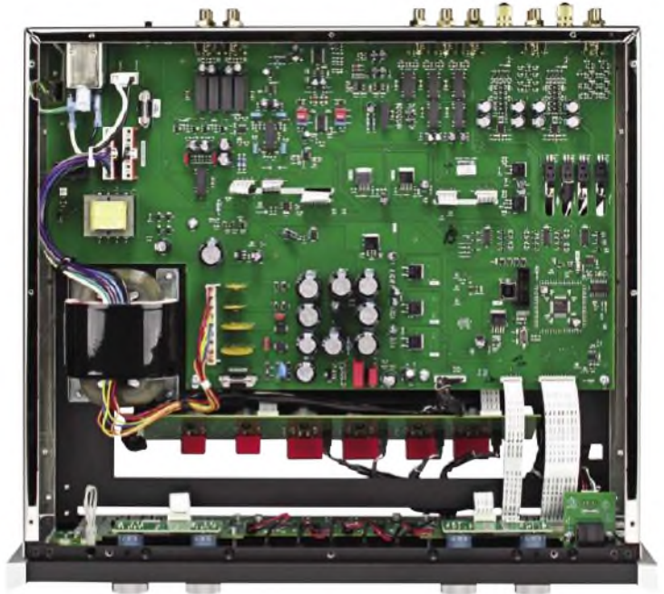
Inside the C70, a big C core mains transformer at left and much solid-state circuitry too.
