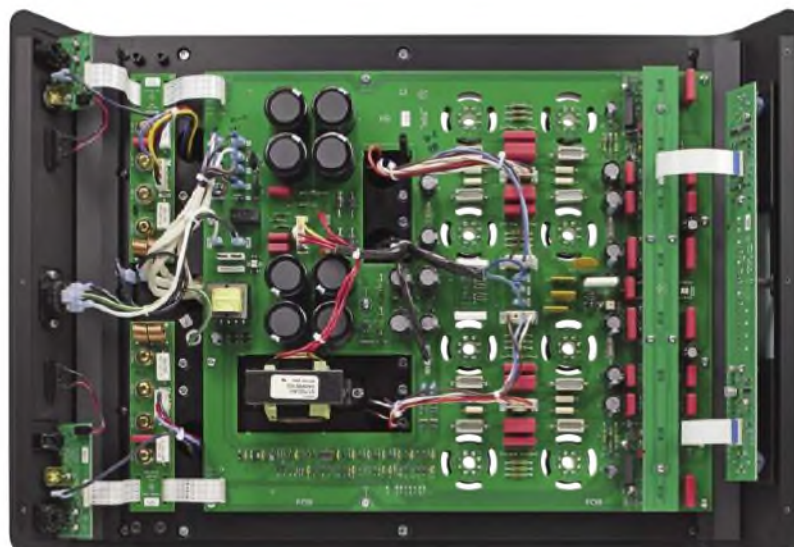
Underneath the power amplifier sit eight (round black) smoothing capacitors, a choke and front display board at right.
