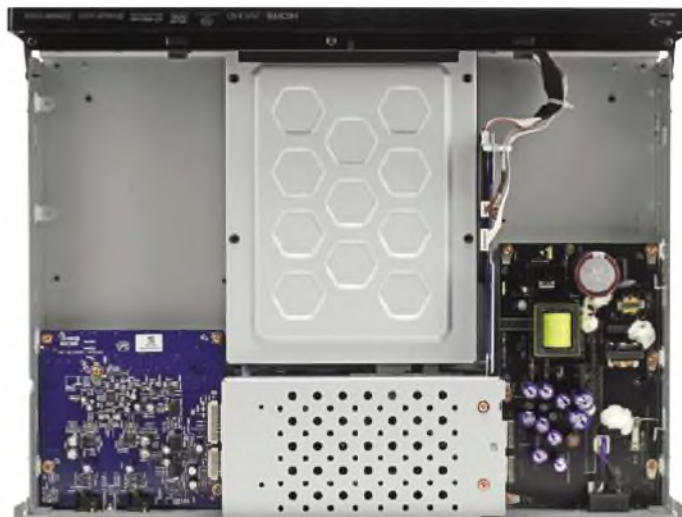
In the middle is the transport, beneath which is a screened section containing the player and video circuitry. On the lower right is the switched-mode power supply; its opposite number is the audio board, which is based on the premium 'Velvet Sound' AK4490EQ DAC from AKM.
