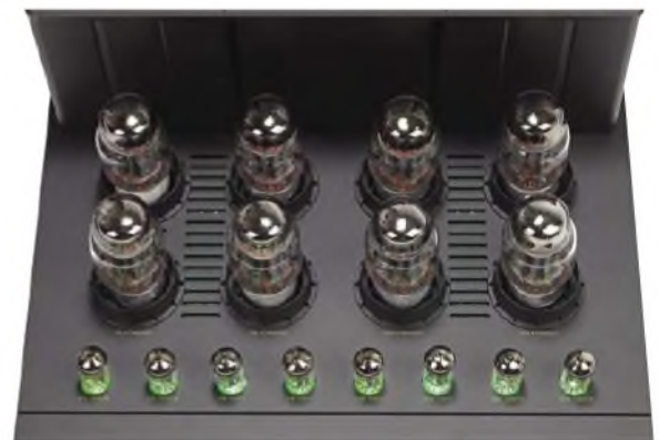
Eight KT88 output valves, fronted by a row of small signal valves, here lit green by LEDs set beneath them. Blue is a switchable option.
