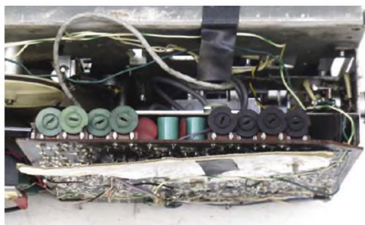
Level and bias adjusters, accessible from the back of the machine, are provided to optimise ferric and chrome tapes for accurate Dolby tracking and frequency response with blank tapes.
