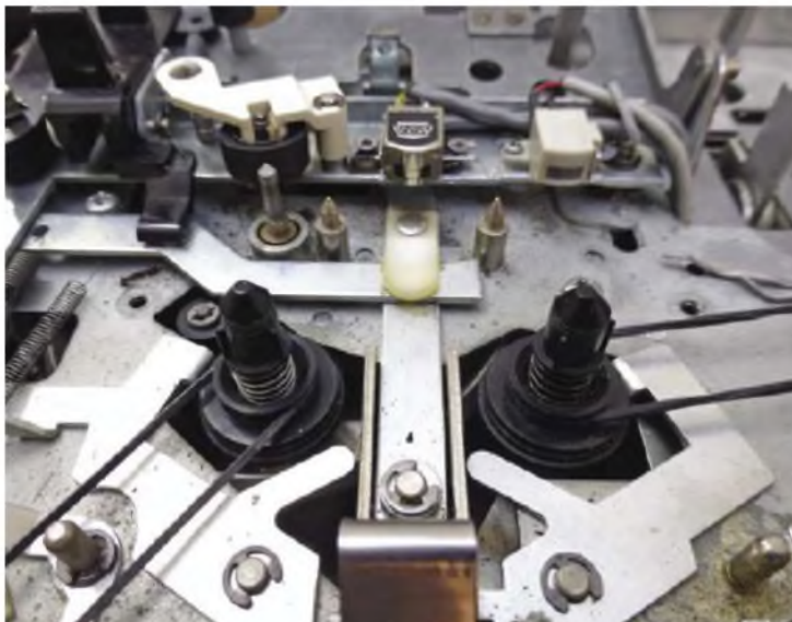
The Wollensak mechanism is simple but effective – and very well made. This 201 doesn't have the original tape head – it has been replaced at some point.
