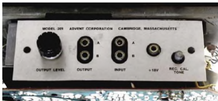
Line inputs and outputs via phono sockets. A microphone pre-amplifier was a separate purchase, powered from the 18V DC phono socket. A level control adjusts the 201's output to suit an external amplifier, and an oscillator has been provided for calibration and line-up purposes.
