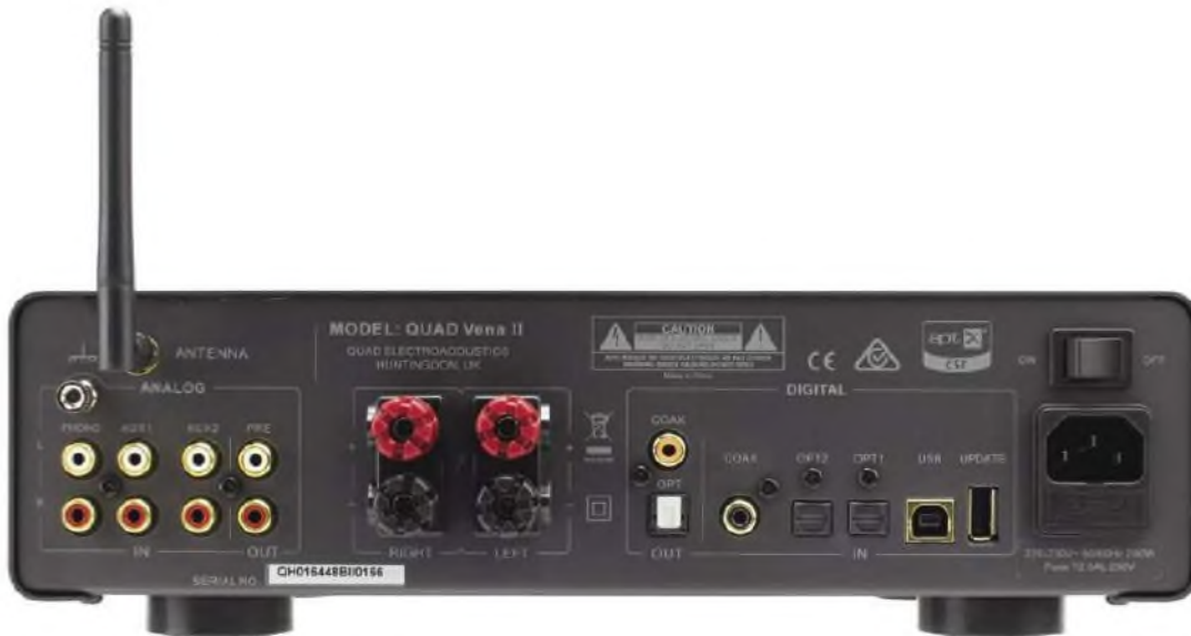
It may look bare and the 'speaker terminals basic, but there are a lot of inputs on the rear panel, from analogue turntable (MM) at left through to digital USB at right, plus an aerial for Bluetooth.
