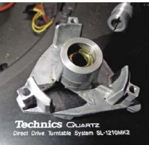
The main bearing from an SL-1200 Mk2. It can be replaced with an 'aftermarket' type with clearly audible benefits.
