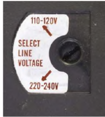
A mains selector, accessible with the platter removed, allows this S-1200 Mk2 to accommodate a range of mains voltages. Japanese models, like the MK3, are 'fixed' to 110V - you'll need a step-down transformer to use them in the UK.
