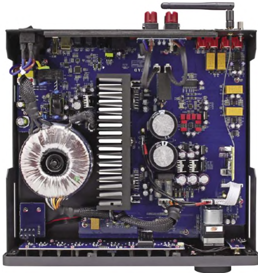
A toroidal mains transformer at left of the Quad's linear power supply. At middle sits the amplifier's finned alloy heat sink and at bottom right the Alps motor driven volume control.
