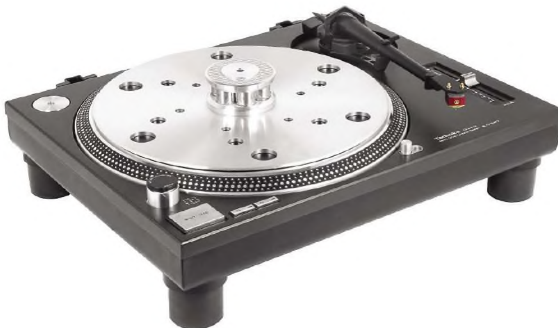
A Timestep Technics Evo modified Technics SL-1200 Mk2 with SME309 arm, improved main bearing, plinth and platter, and with puck and external power linear supply. Used by Hi-Fi World for measurement and listening purposes.
