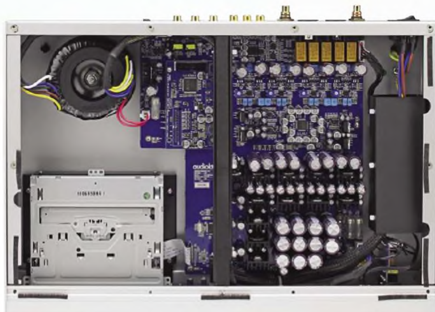
The Audiolab uses a linear power supply with toroidal transformer (top left) plus a slot-loading CD drive (bottom left). Both these are isolated from the main circuit board to avoid interference. Note all the smoothing capacitors (bottom right!).
