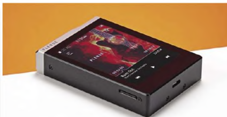
A micro-SD slot on the left side of the player accepts up to 128GB of extra memory storage.
