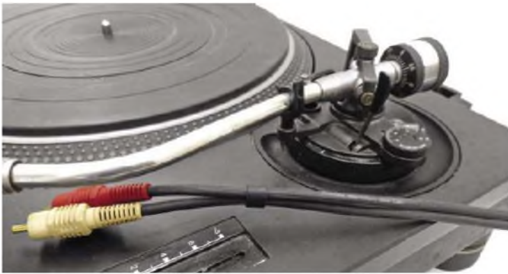
The 'stock' tonearm of the SL-1200 was designed for punishing DJ use, rather than to be the ultimate statement of audio fidelity. A great feature is its ability to accept SME-type bayonet headshells.
