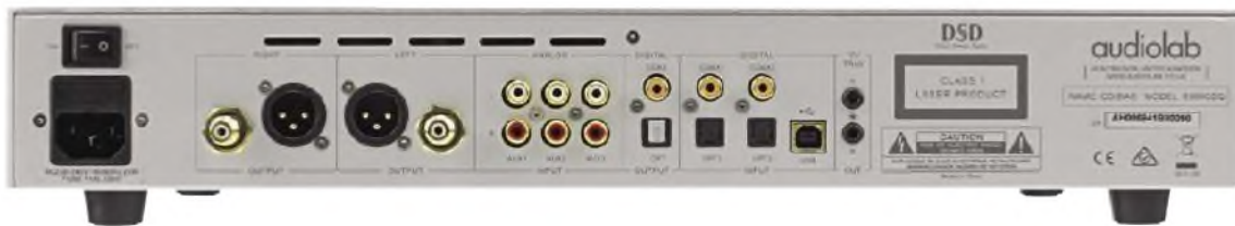
The rear has both phono-socket and XLR outputs (left). Digital inputs are co-axial and optical, plus USB (right). There are three analogue line inputs too (centre).
