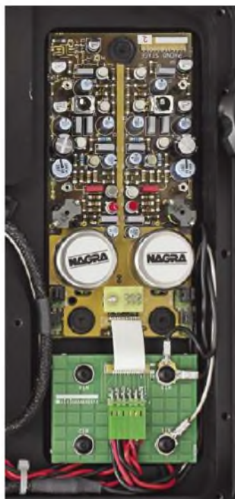
Nagra's phono board with gain switches near top, cylindrical MC input transformers below, and MM/MMC jumpers just below them.
