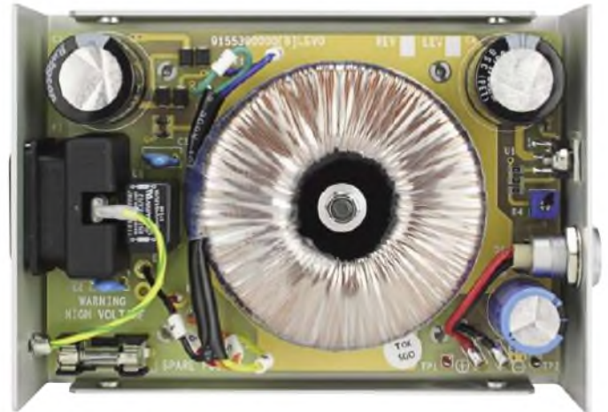
A toroidal mains transformer dominates the interior of Nagra's linear power supply – no switch-mode here.
