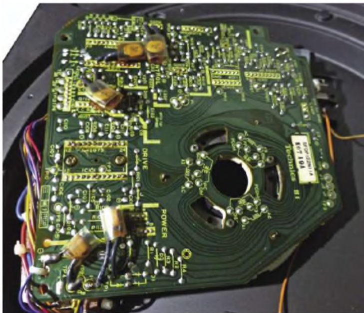
An SL-1200 Mk2 circuit board, the connections to the Direct-Drive motor's coils can clearly be seen. Technics used the same basic design, which has stood the test of time, for many years.
