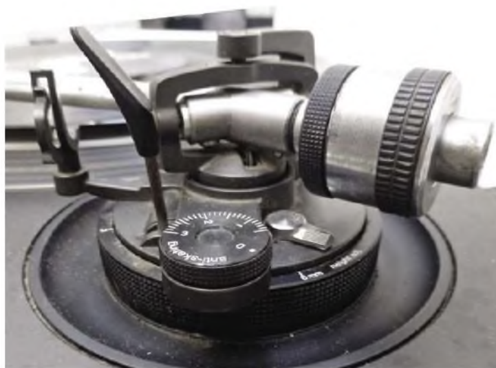
The arm can be raised or lowered by a lockable rotating collar. This feature and an anti-skating range and counterweight that can accommodate playing weights up to 3g (more with some modern versions), allow the arm to be used with a wide range of cartridges.
