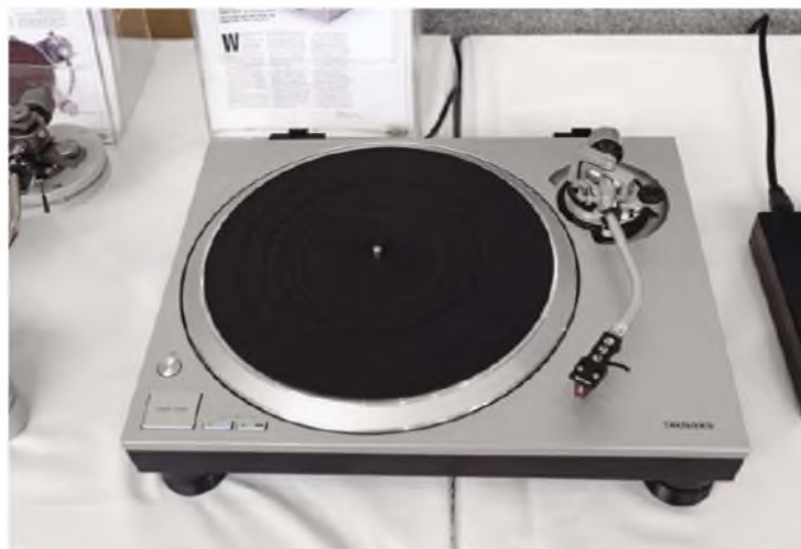
Technics new SL-1500C turntable lacks stroboscope and cue light, but comes with phono stage and Ortofon 2M Red budget MM cartridge.
