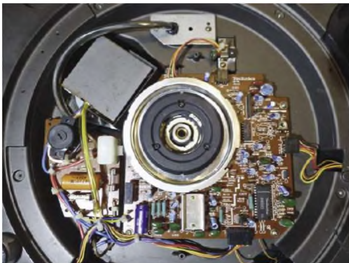
Beneath the SL1200 Mk2's platter are control and heatsinked drive chips, plus mains transformer shielded to reduce hum.
