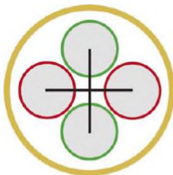
A Star Quad balanced cable has two pairs of cables twisted together to give greater rejection of electromagnetic interference due to its symmetry relative to outside sources.
