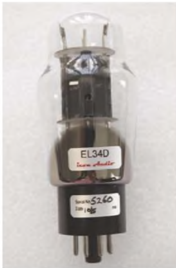
Icon Audio's new EL34D triode valve – a plug-in replacement for the classic EL34 pentode.
