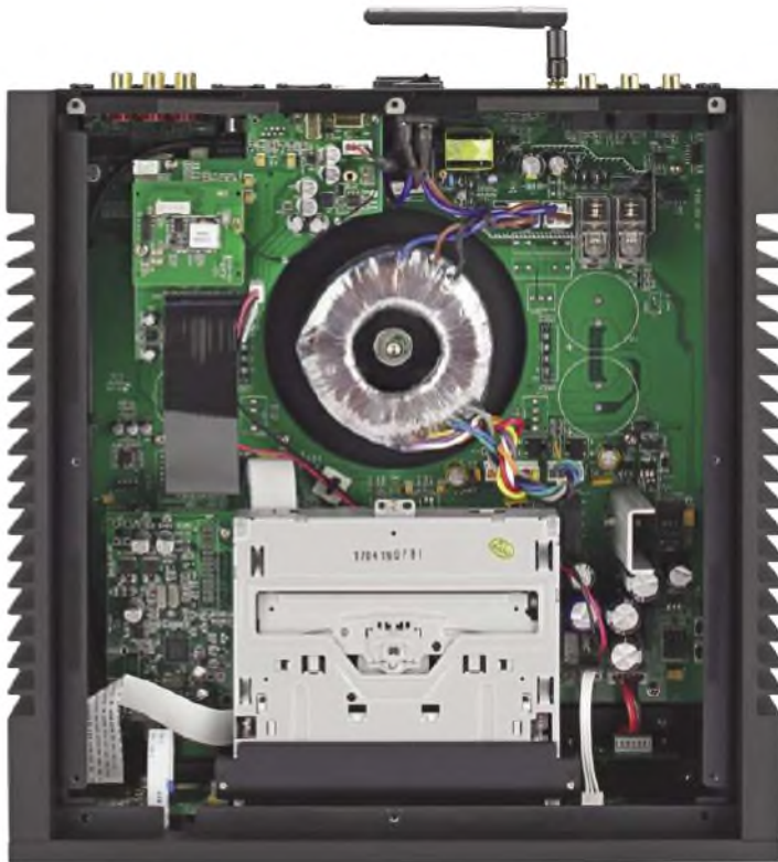
Central to the Artera Play+ is a big linear power supply fed from a large toroidal mains transformer – the shiny round thing. Most manufacturers use cheap switch-mode supplies nowadays; Quad have put audiophile effort into the Play+.
