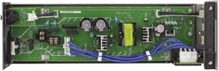
The external power supply is a switch-mode type, able to work on any mains voltage.
