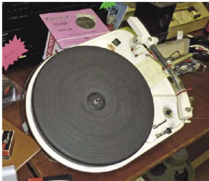
The Garrard 4HF came after the 301 and "was part of a cheaper range of turntables with integrated tonearms" says David Mansell.
