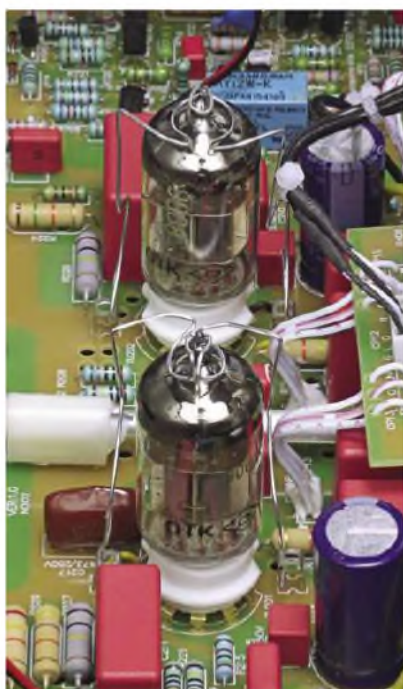
The two 6N1P-EV triodes with spring retainers and ceramic bases.
