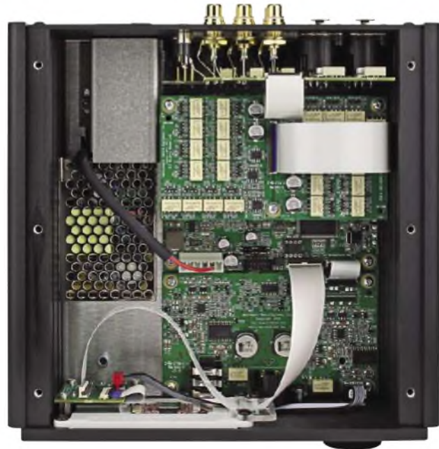
The integrated power supply (left) is a quiet and cool-running switch-mode design. Obvious are the banks of surface-mount relays (64 in all!), which form part of the unit's cost-no-object, all-analogue volume control system. These, Benchmark claim, offer 0.5dB of resolution per step (of which there are 256).
