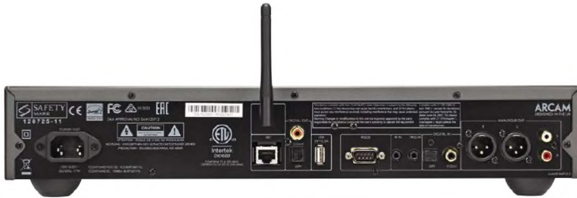
The CDS50 rear panel has an Ethernet socket for wired network connection and wi-fi aerial too (both at centre). There's a USB A socket for flash drive, digital optical and electrical inputs and, at right, both phono socket and XLR analogue audio outputs.
