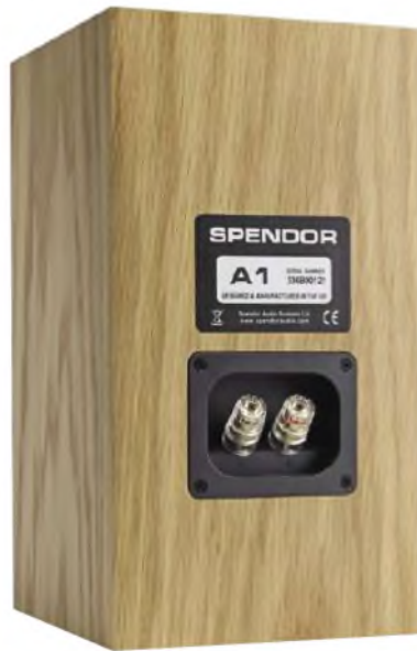
The A1s are a sealed-box design, making placement easy. Their binding posts are of high quality.
