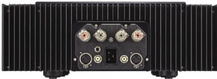
The rear of the SPM 1050 Mk II has gold-plated balanced XLR and unbalanced RCA inputs, alongside sturdy loudspeaker outputs.
