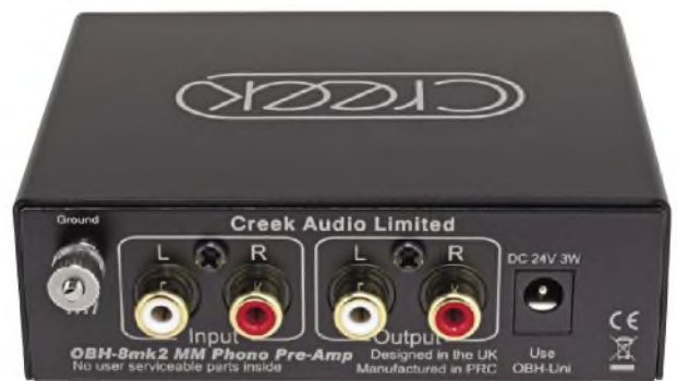
The rear panel is simplicity itself, phono socket inputs and outputs only, plus a 24V d.c. power socket.
