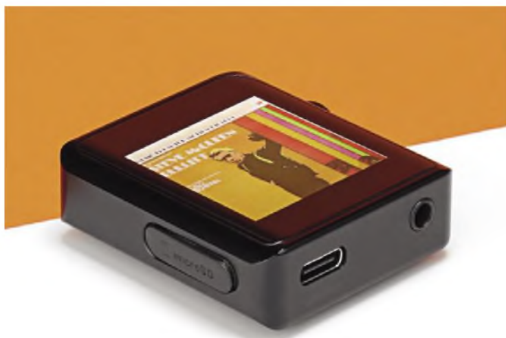
One micro-SD card slot with simple plastic cover, a headphone / line output (no optical digital) and USB socket.
