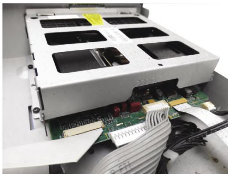
The CD burner, showing the laser sled (under the metalwork) and the various connections. It can copy at double-speed from the play-only transport and supports CD-Text.
