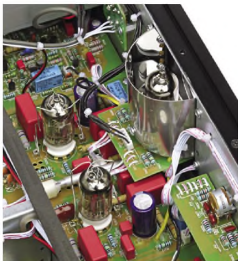
Behind the front panel window is an alloy reflector surrounding the 12AX7 input valve – seen at right.
