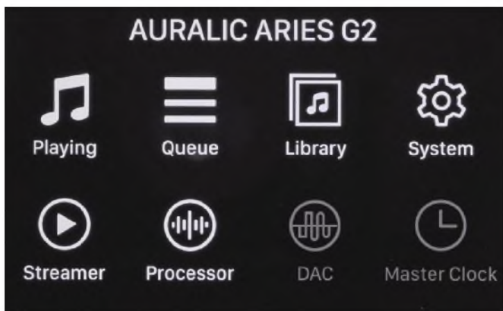
The Aries G2's main front-panel screen, divided into eight categories. Unless you're using the Vega G2 streaming DAC, or another Auralic model equipped with Lightning Link, the DAC and master clock icons will be greyed-out. Note the lack of an Internet radio menu.
