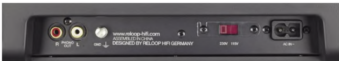
A simple rear panel with one set of phono outputs and earth terminal. There also a voltage select switch (230/110v) and an unusual voltage inlet with asymmetric calculator-style socket.
