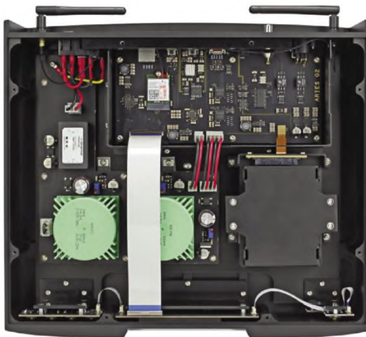
The neat internal layout of the Aries G2. There are two linear power supplies driven by those green transformers, plus a small standby supply. An internal bay for a 2.5in hard drive or Solid State Drive (SSD) sits a bottom right. At rear sit wi-fi aerials. The whole sits in a rigid machined alloy one-piece case.
