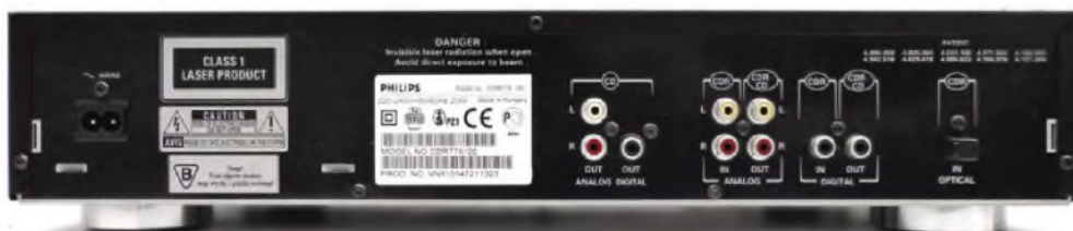
The CDR775 had optical and coaxial digital inputs for recording from sources like DAT, DCC, Minidisc or DAB; there's also an analogue input for 'needle-drops' (via your phono stage) and archiving tapes.
