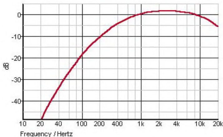
The common IEC A Weighting curve (courtesy Sengpiel Audio). "I think it's a bit dishonest and maybe somewhat misleading" says Vince Hawtin.
