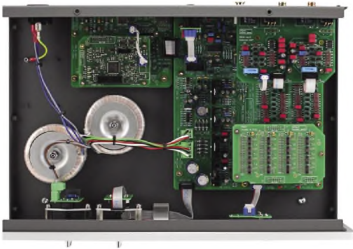
At bottom-right is the R-2R DAC board - count those resistors! Underneath it is a powerful DSD chip that does decoding and conversion of serial data into the parallel form needed by the DAC section.
