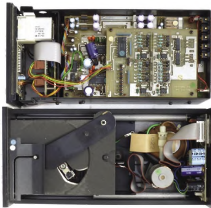
The 207 was one of the first 'two-box' CD players. One box contains the Philips CD mechanism and its power supply, while the other contains most of the electronics. As can be seen, the standard of construction is high - as one would expect from a British-made product that happened to be one of the most expensive CD players then available!
