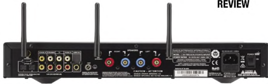
The rear panel has analogue and digital inputs, aerials for wi-fi and Bluetooth, as well as solid 'speaker binding posts. It's tightly packed but all connections are easy to access.
