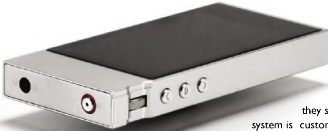
A nice spin-wheel analogue-feel volume control, track skip and play/pause buttons, plus an on/off button at top and single 3.5mm stereo jack at left, for Phones or Line.
