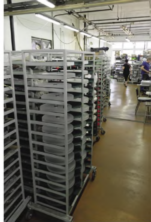
Acrylic platters with fitted centre spindles stacked high as they go through the manufacturing process.
