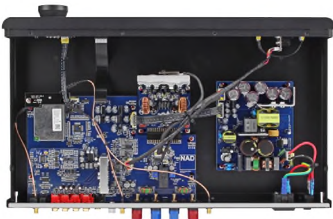
The C338 has a custom Class D amplifier built around the well-regarded Hypex module. At right sits a compact switch-mode power supply. There's a lot in a small case.
