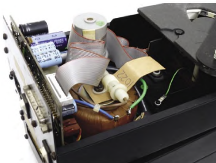
To extend and withdraw the glass-fronted disc tray, Meridian built in an enormous Philips DC motor that seems like overkill! It's coupled to the drawer mechanism via a toothed belt. The ribbon cable connects the Philips CD loader (a CDM-1 or CDM-4, depending on your unit's vintage) to a computer-like DB25 socket on the rear panel and thence to the electronics half of the 207. Note too Meridian's use of a toroidal mains transformer.
