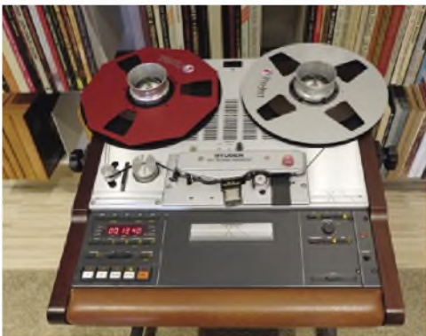
Pro-ject's Studer A807 open reel recorder, threaded with a 1/4in tape of Pink Floyd's 'Dark Side of the Moon'.
