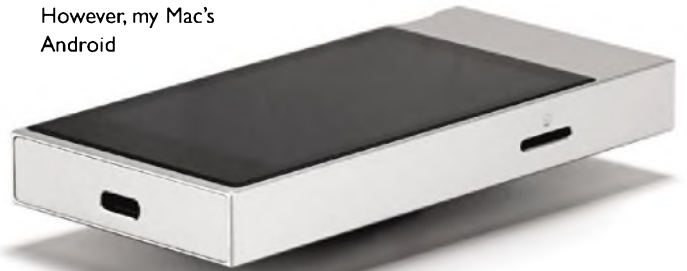
USB C digital connector on the bottom face and single 512GB microSD card slot at right.
