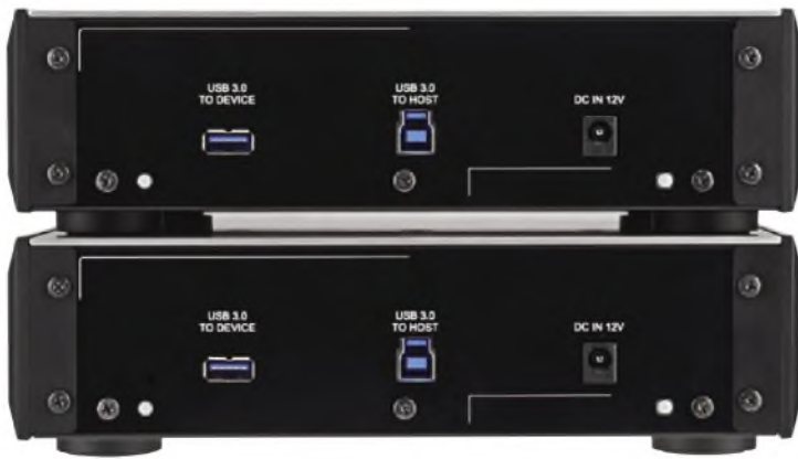
USB sockets are used for connecting both units to the main Melco music library, in my case a Melco N1A Mk2.
