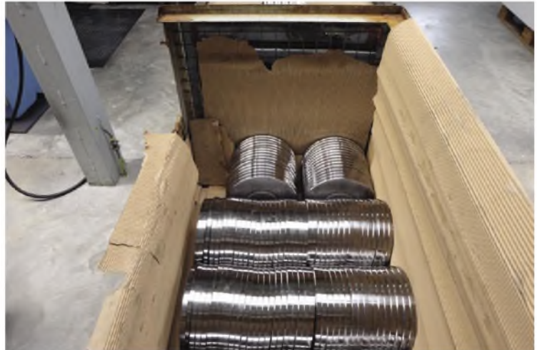
Aluminium platters sit in shiny lines after being turned on metal lathes.
