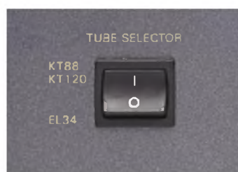
A side-mounted rocker switch changes bias to suit EL34s, KT88s and even KT150s PrimaLuna say.
