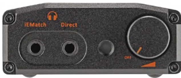
Two sockets are provided for headphones of different sensitivity – the ‘direct’ one ‘goes louder’! Next to this is the LED, which confirms the state of internal battery charge and what type of signal is being applied. The volume control is combined with an on/off switch
