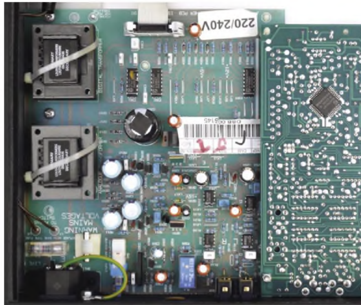
Inside the Arcam Delta Black Box 3. Note the presence of two mains transformers, which feed separate supplies for the analogue and digital sections of the unit. The adjacent digital board is 'track-side up', which means the surface-mounted Philips SAA7321GP Bitstream converters – which operate in dual-differential mode – are visible. The quality of construction is to Arcam's usual high standard.
