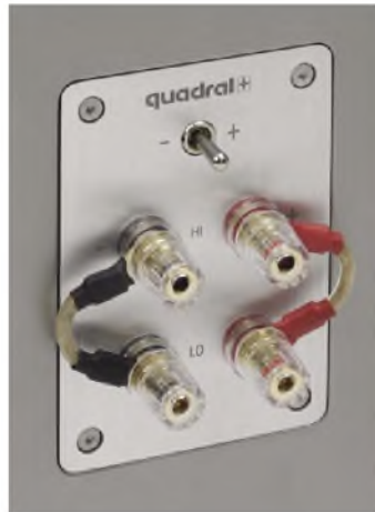
On the rear panel is a toggle switch to alter high-frequency response. It can be set to +/- or neutral.
