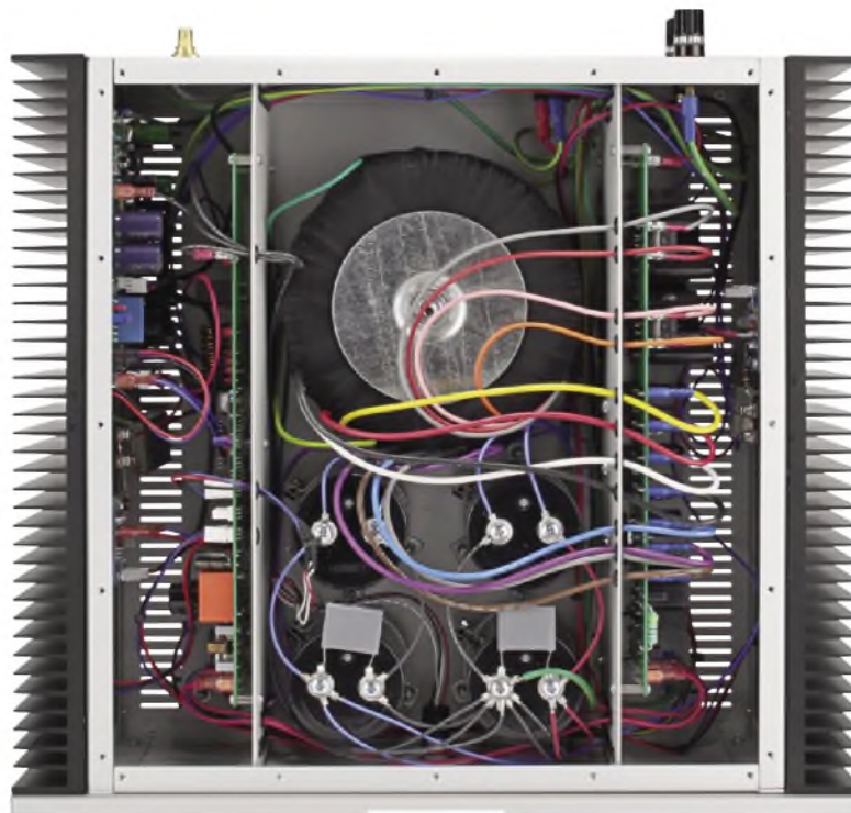
The Longdog monoblocks employ a large toroidal transformer to power the output section of the amplifier, as well as the smaller push-pull sections.
