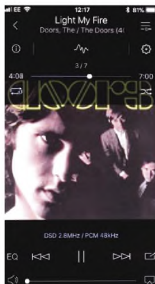
The DoP selector of Onkyo's HF Player that will run on an iPhone. It sends DoP out through the Lightning socket, to external DoP enabled DSD DACs.
