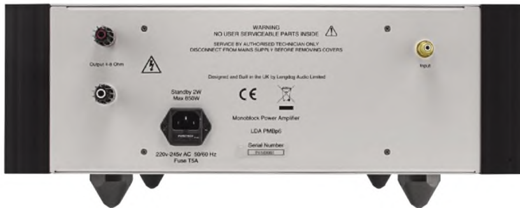
Loudspeaker binding posts, a single RCA input plus an IEC mains input take up the back of the LDA P6. Simple - but effective. There is no balanced XLR input.
