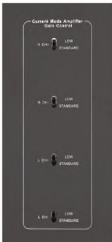
Recessed slide switches on the base of the CMA400i determine headphone-amplifier gain (1.1 or 2.5dB).
