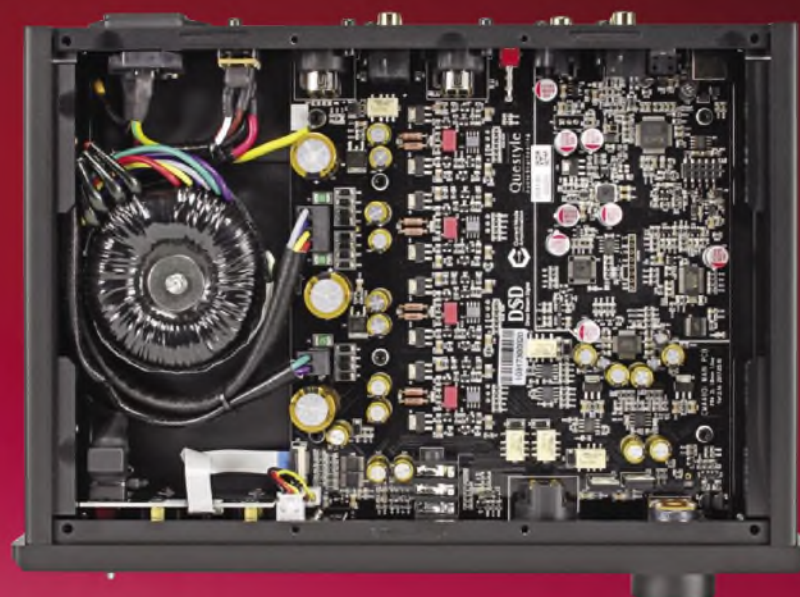
Internally, from left to right is the mains power supply with toroidal transformer, headphone amplifier and digital section with AKM AK4490 DAC chip.
