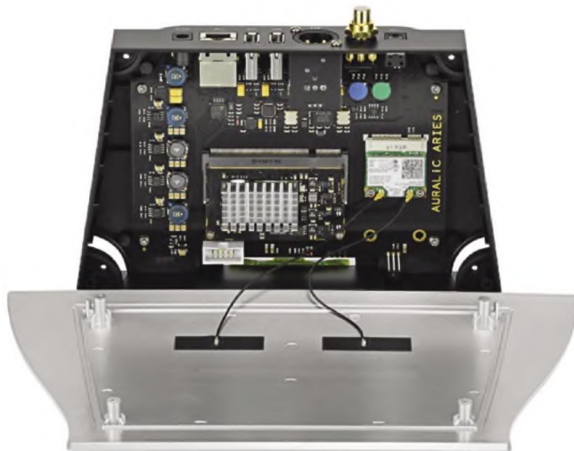
Inside the Auralic uses two FemtoClocks (one for USB, a second for all other inputs) to reduce jitter.
