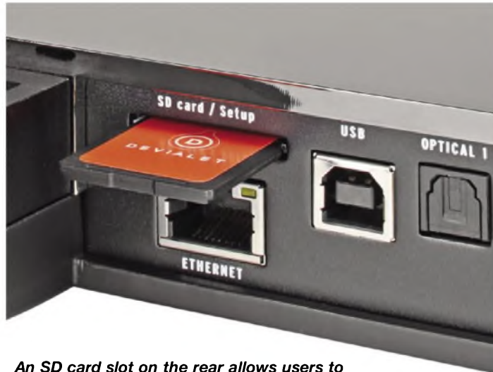
An SD card slot on the rear allows users to configure the amplifier to personal taste.
