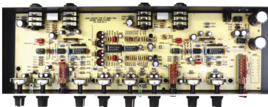
The Aphex 104's economical offers two channels of Aphex Aural Excitement and 'Big Bottom' processing. Most of the chips are standard op-amps, with the exception of a LM13700 'transconductance amplifier – associated with the exciter's filter. Earlier models had the chip numbers removed to prevent the design being copied.
