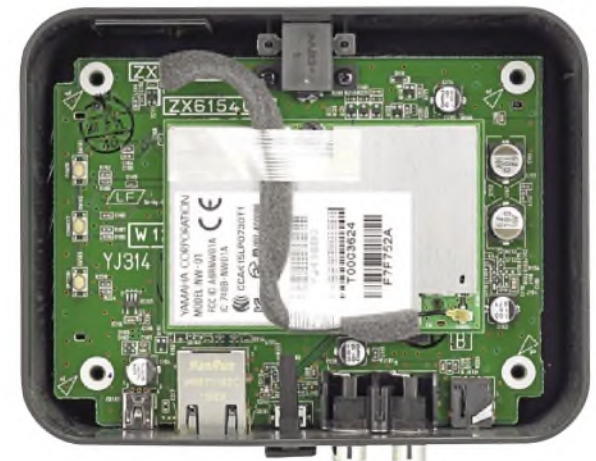
The internal circuitry of the WXAD-10 is neatly laid out and features a Burr-Brown PCM5121 DAC chip.
