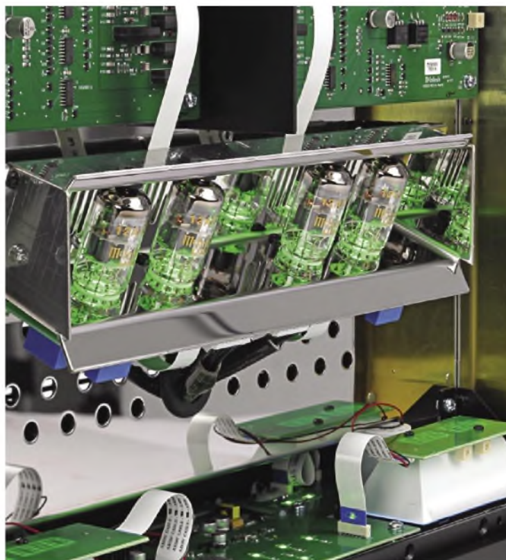
The four 12AX7s sit in their own compartment at top, visible through a window in the top cover. An LED sits under each, lighting orange at warm up and green when running.
