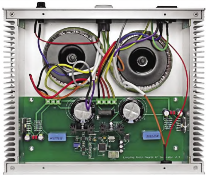
A mains regenerated power supply from Longdog Audio, purposed for turntables, including the Garrard 401.
