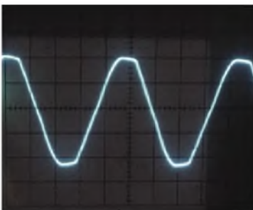
The distorted (3%) mains waveform in North West London. Note flat tops and triangulation.
