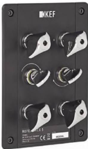
The loudspeaker connection panel features KEF's innovative selection method - turn the centre controls to the left for bi-wiring or the right for single-wire. Clever and convenient.
