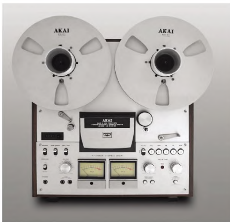
The Akai GX630 open reel tape recorder. Its glass crystal ferrite heads do not wear, says Dave Tutt.
